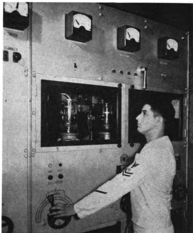
Gilbert Madrig, RM-2, tunes intermediate power amplifier, part of the 500-KW equipment at NAVRADSTA (T) Annapolis.
