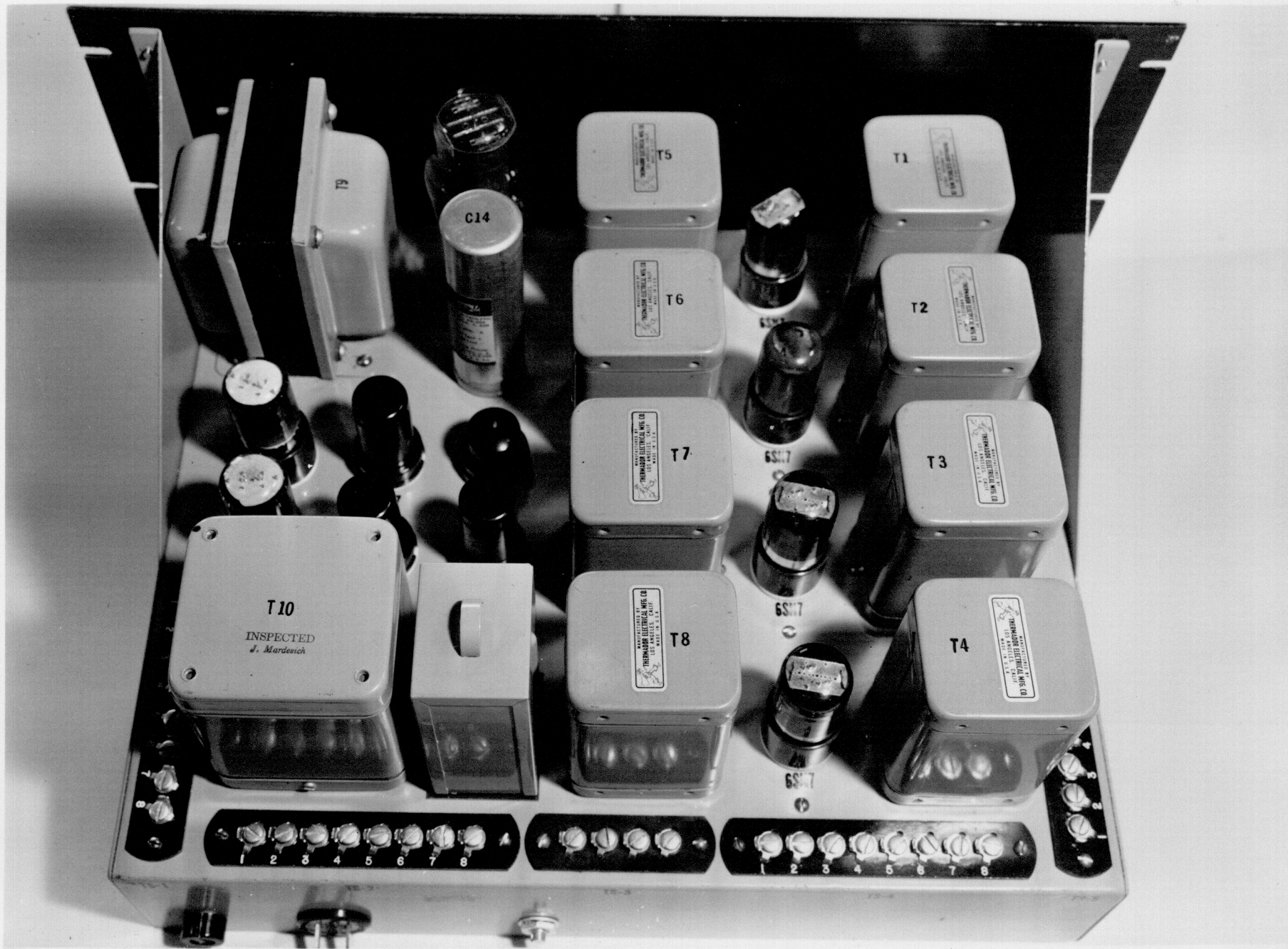
2495-45 Puget Sound Navy Yard 15 May 1945 Photograph (L) Electronic Mixer, Back View.
