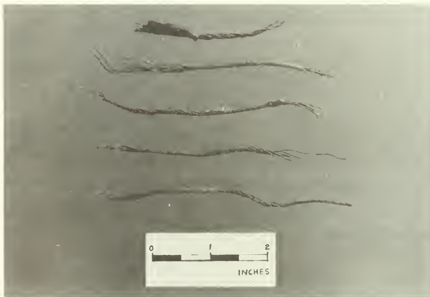
Photograph 69: Seven-strand copper wire
