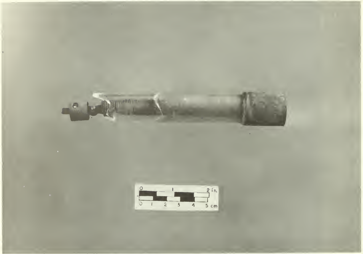
Photograph 60: High voltage fuse--fast acting with rapid heat response to break the circuit
