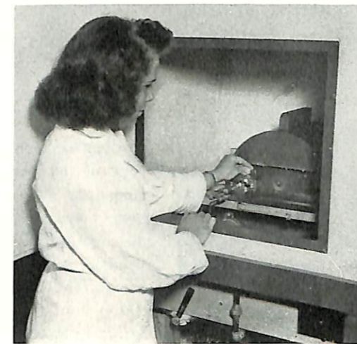
FIGURE 5—The finishing operation is known as wet lapping. The coolant used here is a mixture of equal parts of water and propylene glycol. Crystals must be lapped to a tolerance at little as 0.0005 inch.
