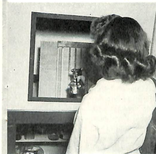
FIGURE 7—When crystals have been cut and lapped, they are placed in a holder as shown. The faces are cleaned by sand blasting before a silver solution is sprayed on.
