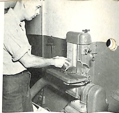
FIGURE 3—Bar ends must be ground to create an index for correct orientation. This is done on a belt sander using a v-block jig fitting two faces of the pyramid-shaped crown.
