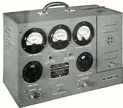
FIGURE 1—Model OCL Tube Analyzer also provides voltage and resistance measurement facilities.
