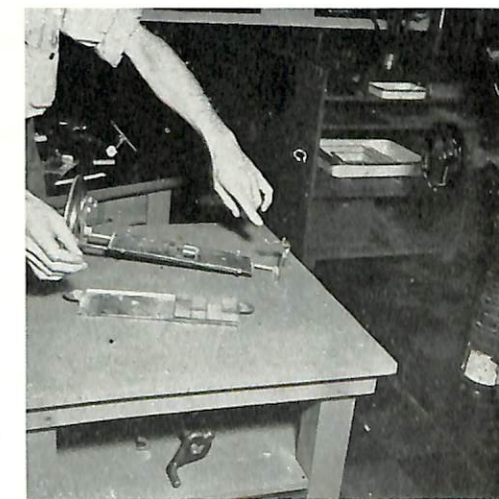
FIGURE 9—Rack for holding crystals in the sputtering chamber. Note clips for attaching the heating coil and gold wire.
