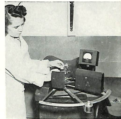
FIGURE 6—Here the accuracy of orientation is being checked by an X-ray machine. Where extreme accuracy is desired, every crystal is tested. For orders requiring less precision, only one crystal out of five or ten is checked.
