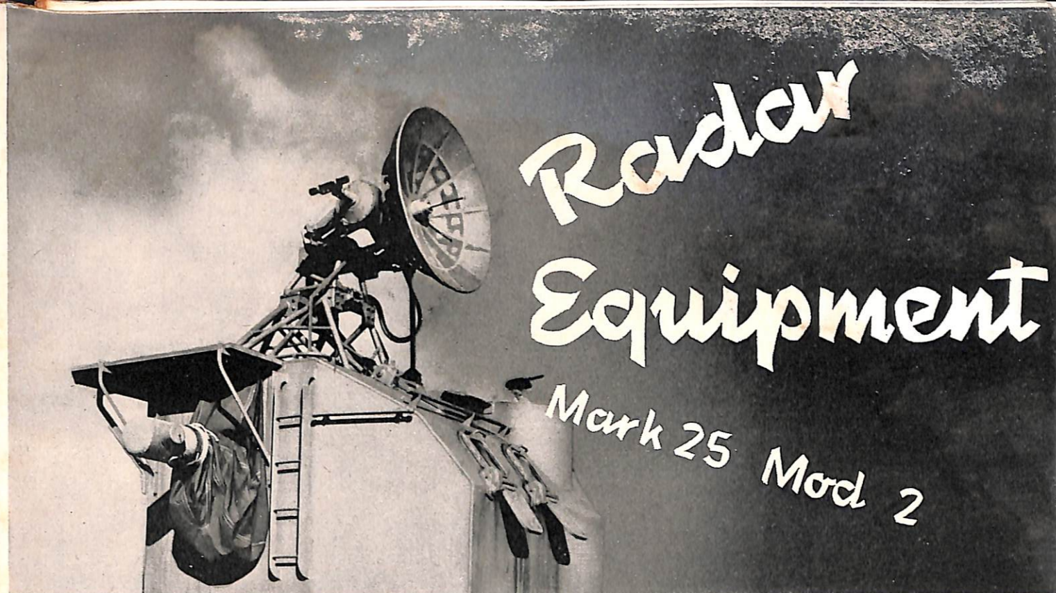
Radar Equipment Mark 25 Mod 2 antenna assembly mounted on a Gun Director Mark 37.
