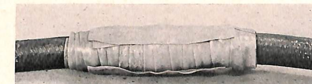
FIGURE 5—Preform ready for insertion in the mold.
