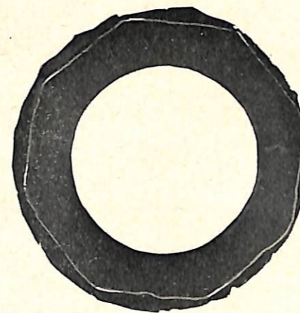
FIGURE 2—Photograph of a packing gland nut that has been removed by means of a cold chisel. Note the damaged edges.
