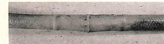
FIGURE 4—Cable jacket knitted together.
