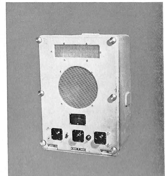
FIGURE 1—The Navy Type CMX-49545 Speaker-Amplifier.
