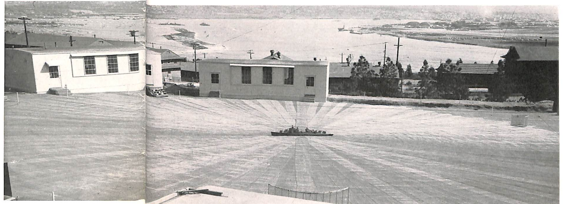
FIGURE 1—General view of a portion of the model range facilities, showing ship model and measuring-apparatus antenna. In the background beyond the Laboratory buildings lies San Diego harbor, suggestive of the practical application of the model range.
