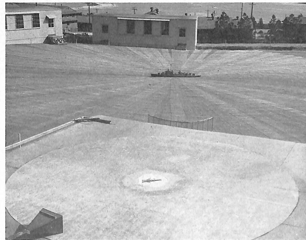
SCALE MODELS on SIMULATED OCEANS are used by the U.S. Navy Electronics Laboratory's model range for research into antenna characteristics. In the background a 1/24-scale brass destroyer stands on metal webbing and in the foreground a 1/480-scale vessel floats in a pool of mercury. Studies of such models have enabled the laboratory's scientists to originate and develop many devices of permanent value to the Navy communications system.
