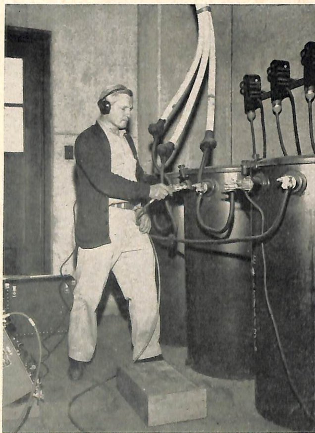
Use of the AN/PRM-1 and Antenna AT-211/PRM-1 in measuring electronic interference levels at transformers located in a sub-station supplying power to a receiving activity.
