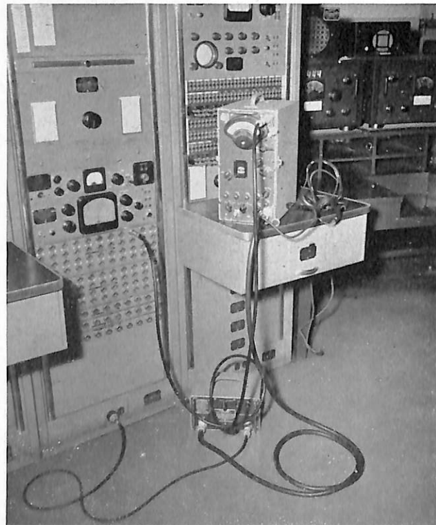
AN/PRM-1 with impedance matching network CU-197/PRM-1 (50 ohm) connected to an antenna switching system.
