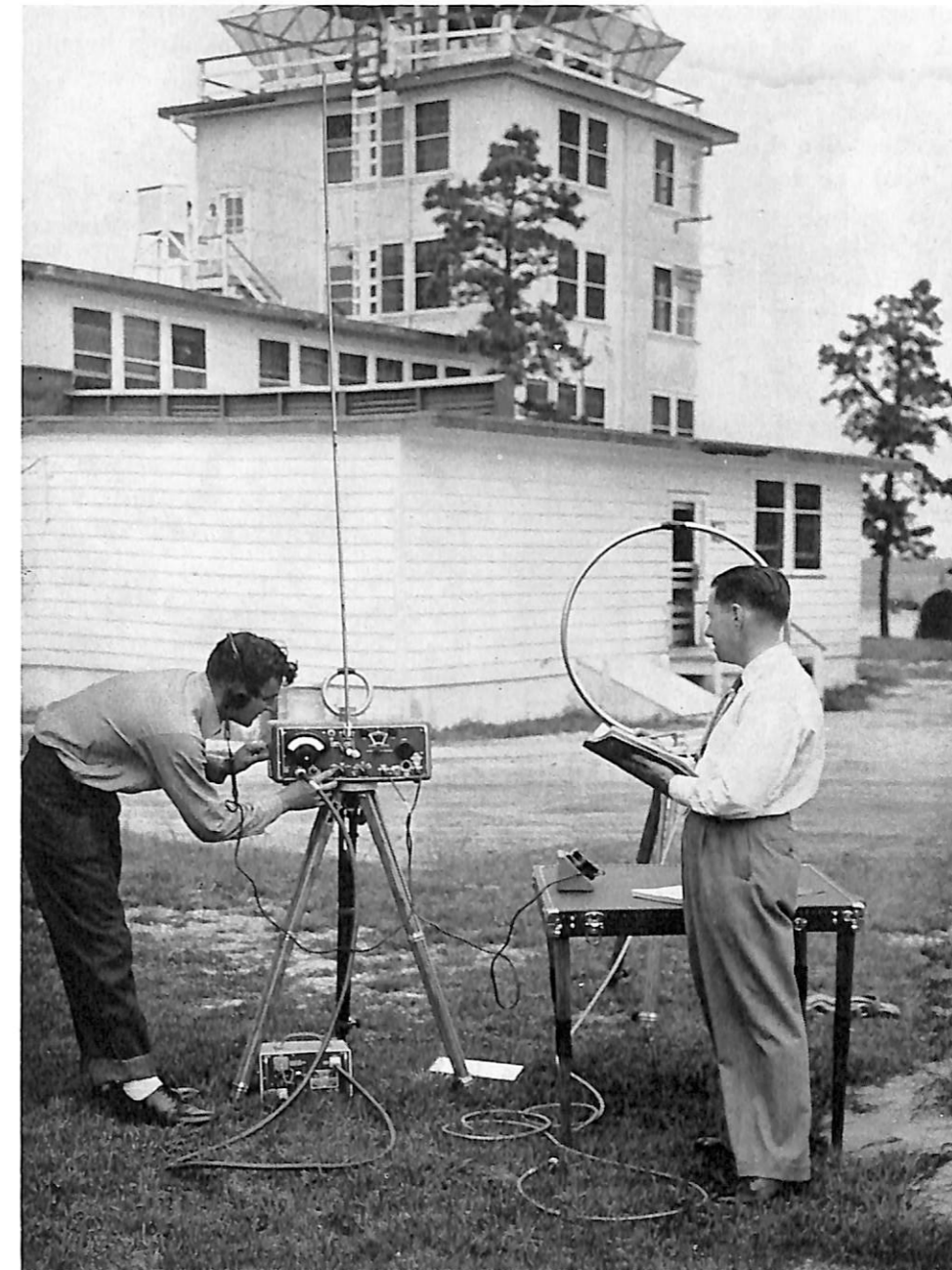
Measuring and locating sources of radiated electronic interference using the AN/URM-6 radio interference and field intensity measuring equipment.
