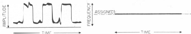
FIGURE 2.—Receiver response to on-off keyed signals when converted by (left) a conventional detector and (right) by an FM discriminator.
