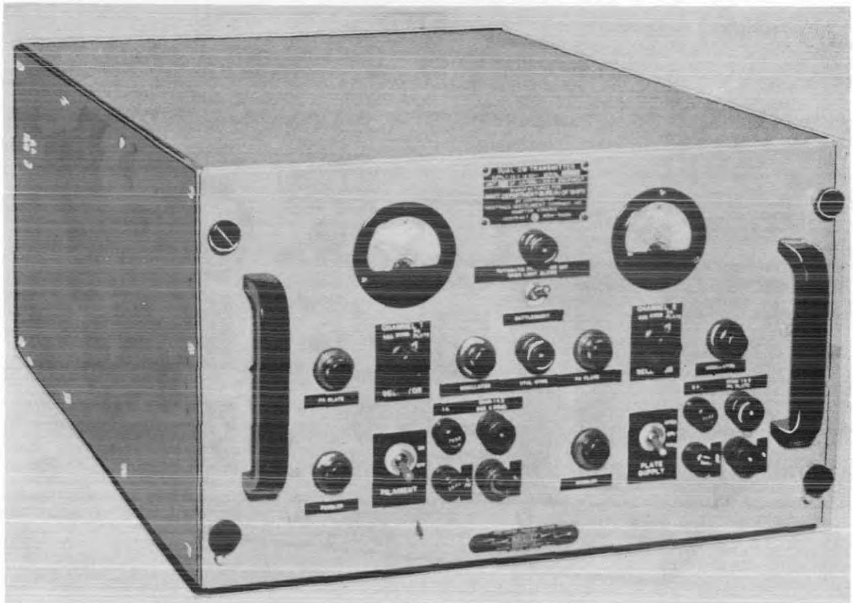
Radio Ranging Set AN/URN-4(XN-1) Dual LF-CW Transmitter
