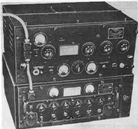
VHF Radio Transmitting and Receiving Equipment TBS, TBS-1 thru -8
