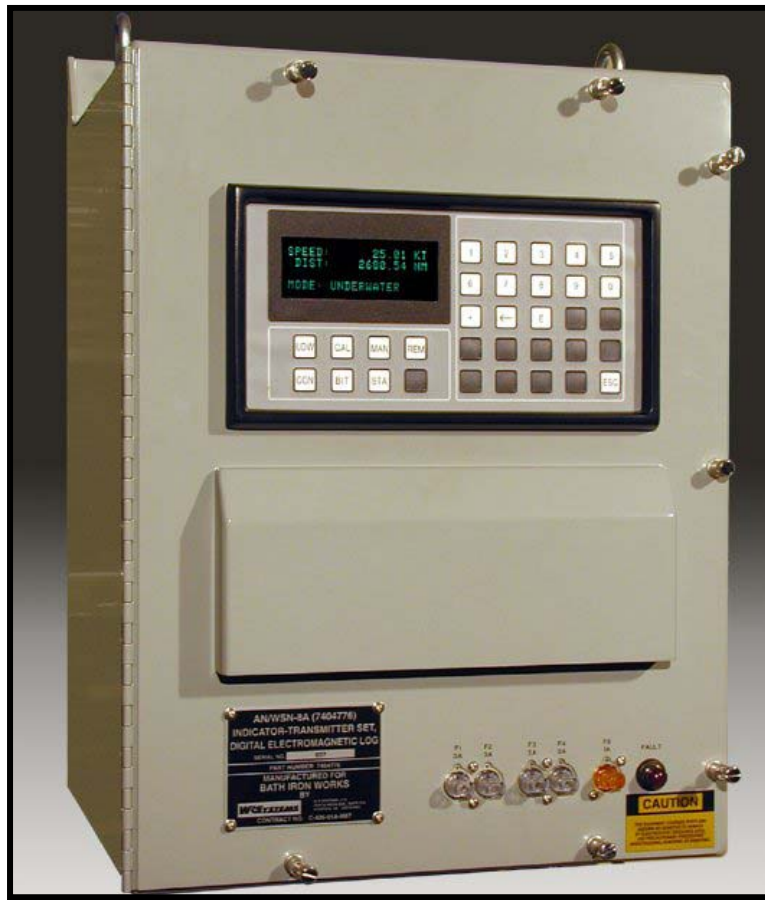
Figure 10-47.— AN/WSN-8A Digital Electromagnetic Log Indicator Transmitter.
