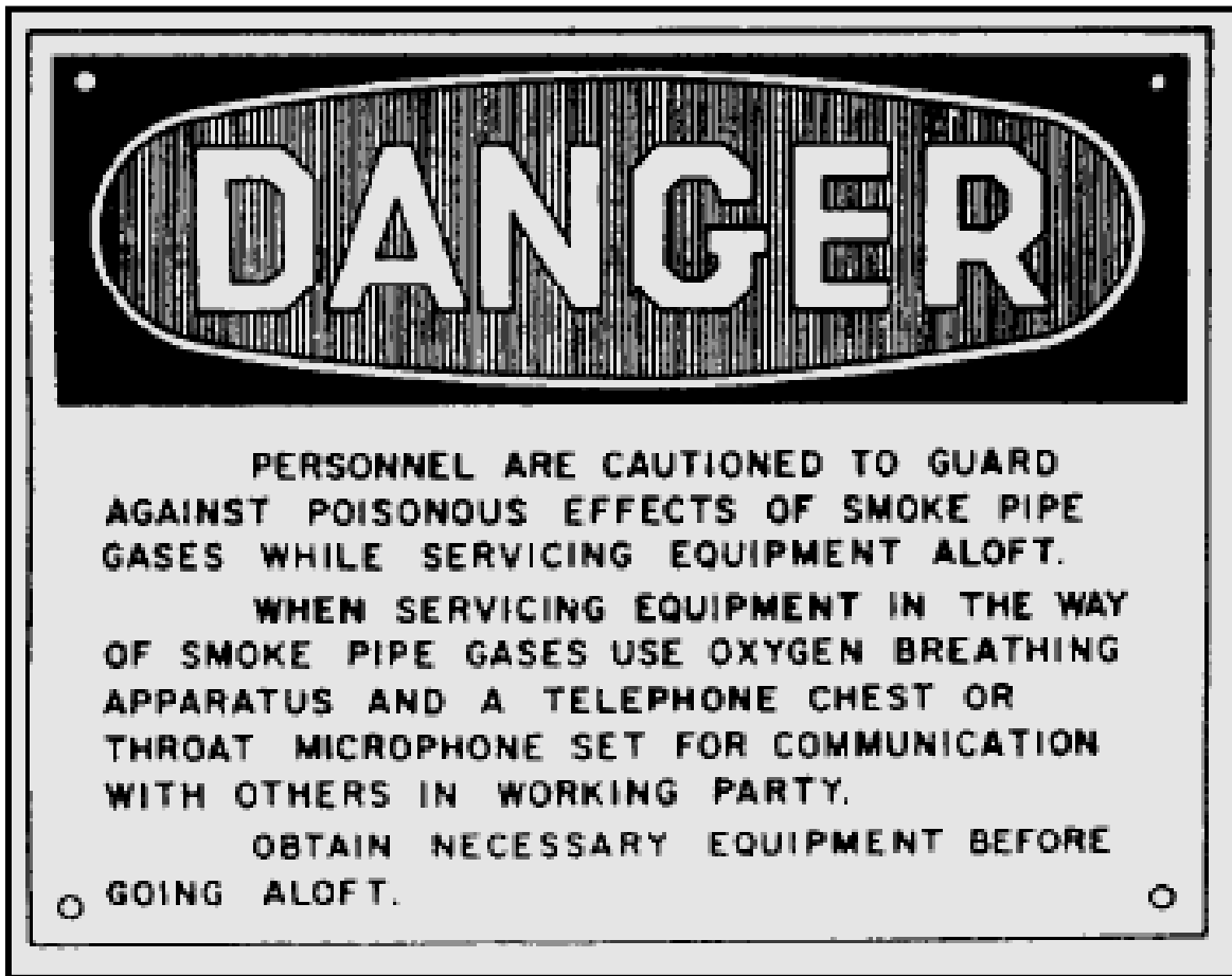
Figure 1-2.-Smoke pipe gases warning sign.
