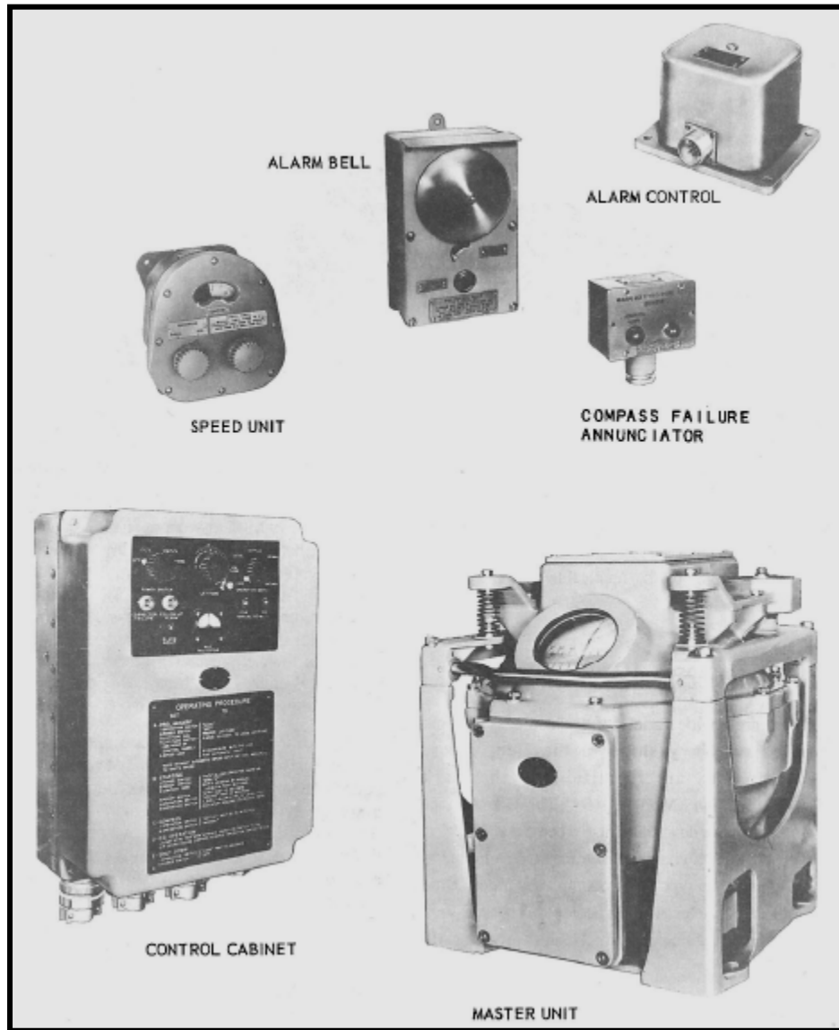
Figure 4-22.—Mk 23 Mod 0 gyrocompass equipment.
