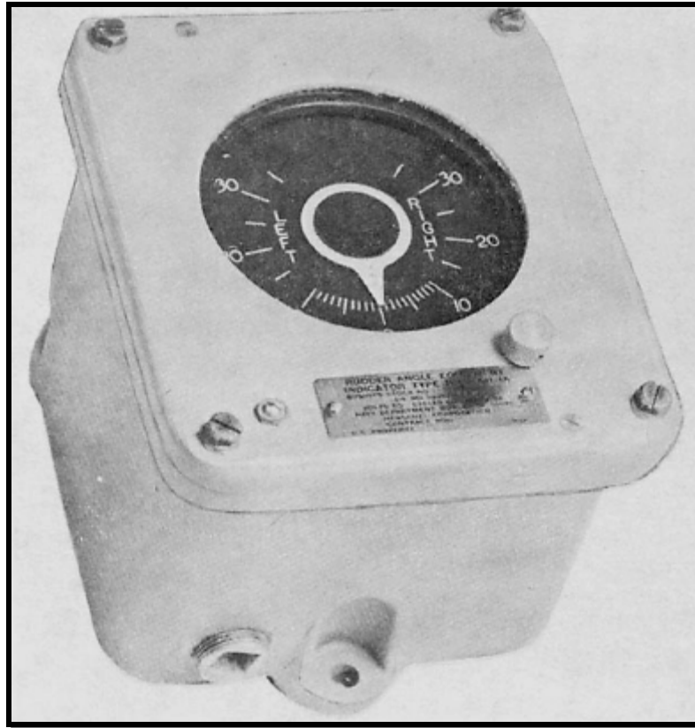
Figure 10-10.—Rudder angle indicator (circuit N).
