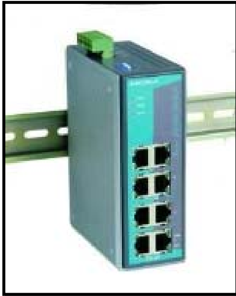
Figure 7-35.— Moxa EtherDevice Switch.
