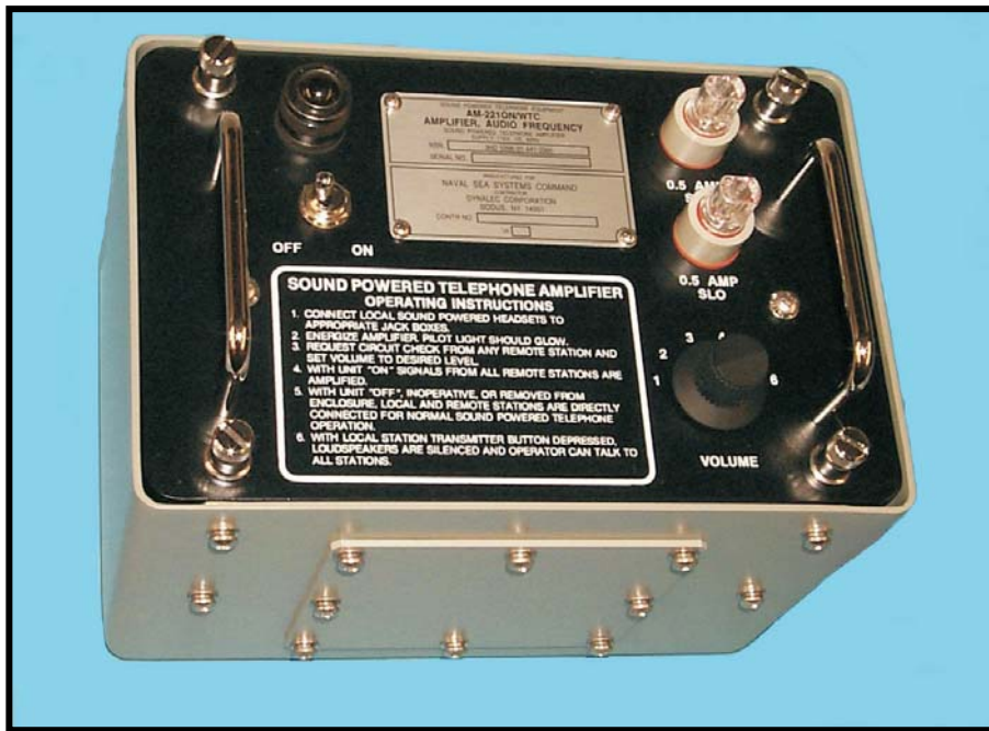
Figure 5-15.—AM-2210N/WTC Sound Powered Amplifier.
