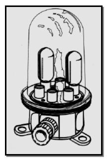
Figure 2-105- Wave-Off Indicator Monitor Assembly.
