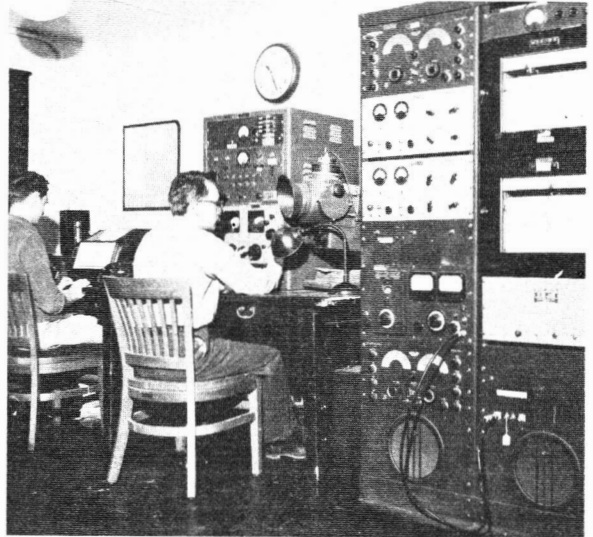
Equipment at right records intensity of radio waves while incoming teletypewriter messages bring data on solar and atmospheric disturbances to radio forecasting center of IGY World Warning Agency.
