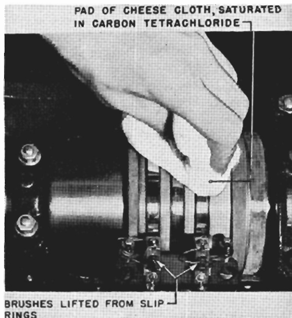
FIGURE 5.—Method of cleaning slip rings.
