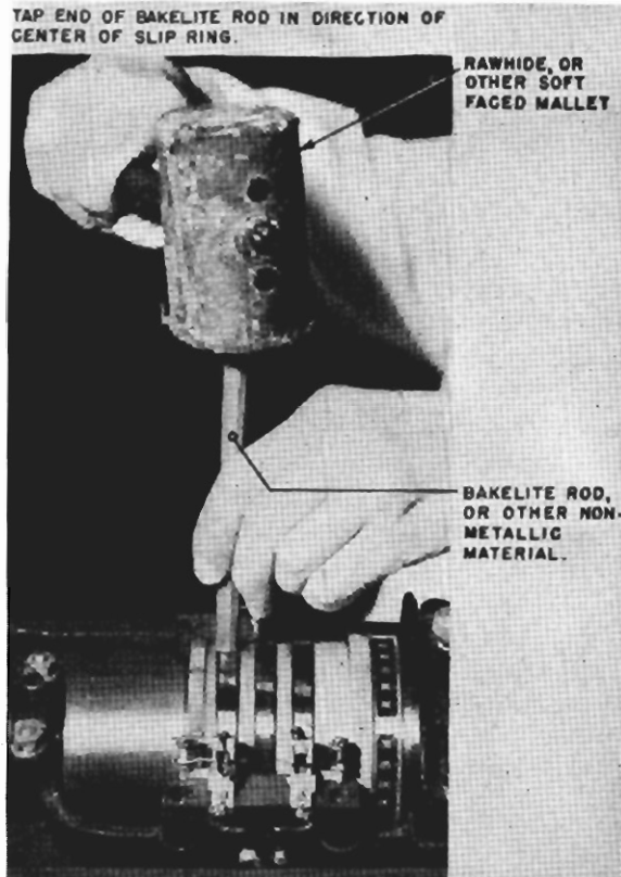
FIGURE 2.—Method of improving the concentricity of the slip rings.
