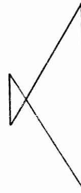
Figure 30d. Distorted trapezoid due to voltage b.
