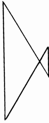
Figure 30c. Distorted trapezoid due to voltage a.
