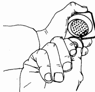
Figure 2-35. Removal Tool Application for Crimp Contacts
