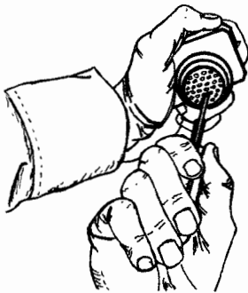
Figure 2-34. Insertion Tool Application for Crimp Contacts
