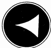
SSB pattern excessive bias on 5894 stage.
