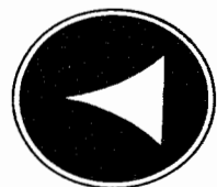
AM pattern excessive bias on 5894 stage.
