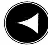
AM pattern excessive bias on 5894 stage.
