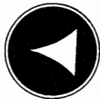
SSB pattern excessive bias on 5894 stage.
