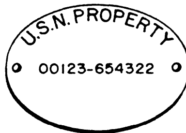
Figure 3-14.-Sample plant property identification tag.
