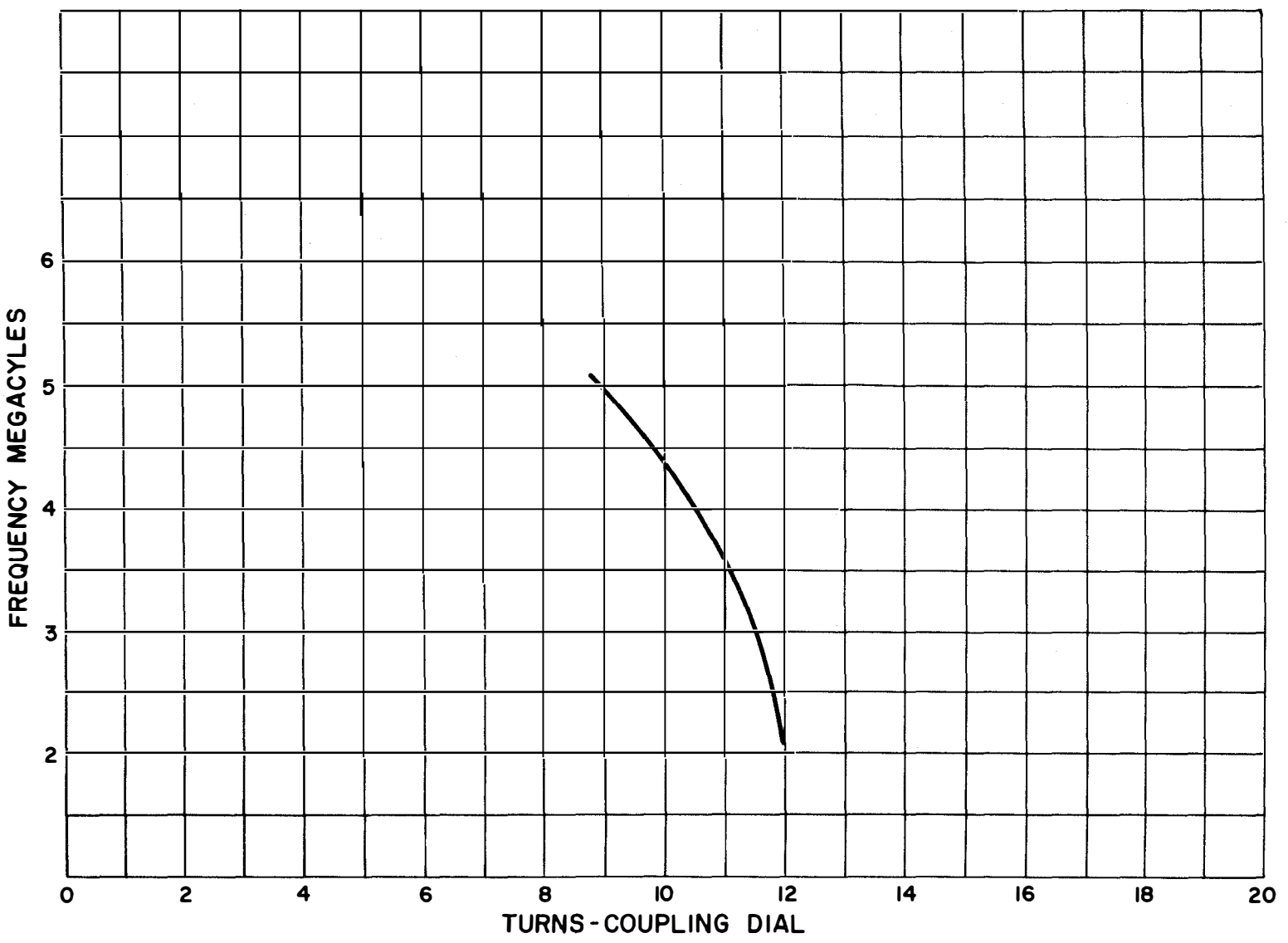
Figure 6-4. Coupling Graph, Antenna Coupler CU-998/FRA-49(V) (2 to 6 mc)
