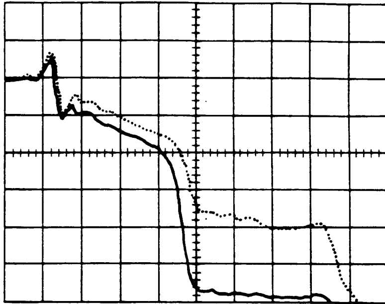
FIGURE 2-18. Low Band – Both terminating resistors are shorted in this display.
