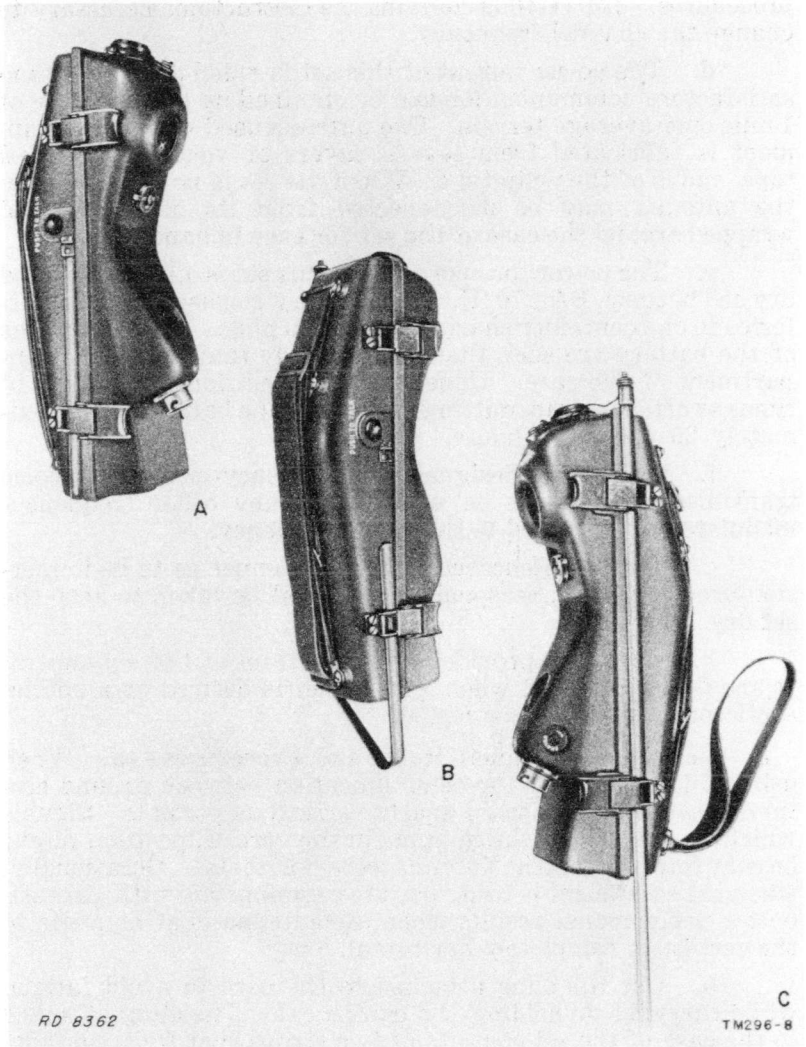
Figure 2.—Installation of antenna.
