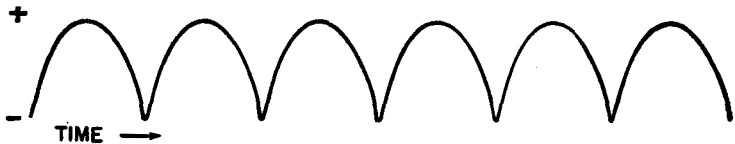
Figure 55.—Output of a full-wave rectifier.
