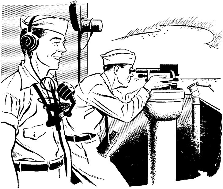
Figure 191.—Taking a bearing with an alidade.
