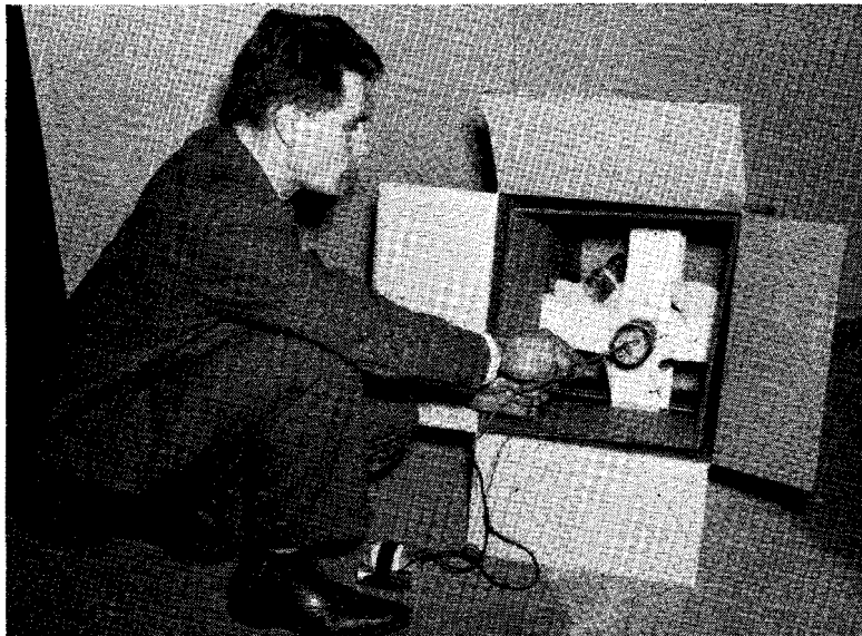
FIGURE 2.—Method of testing Type CWL-S61 Electron Tube without removing it from the shipping container.
