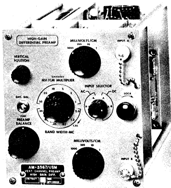
OSCILLOSCOPE SUBASSEMBLY VERTICAL CHANNEL HIGH GAIN DIFFERENTIAL PREAMPLIFIER AM-3567/USM
