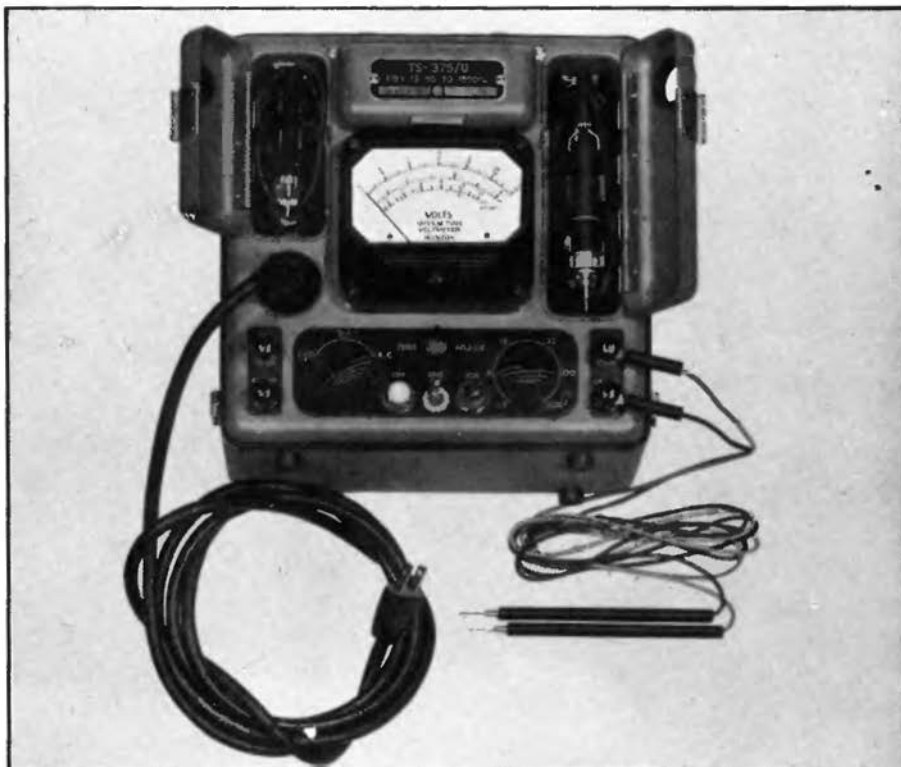
Figure 2-3. Front View Showing Test Leads and Power Cable Connected for Use
