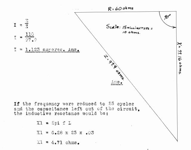
Computing by vector diagram for the resultant impedance:
