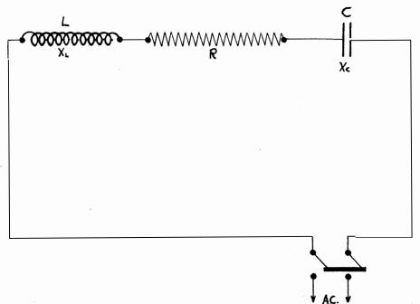
Alternating Current circuit containing Industive Reactance. Capacitive Reactance. and Resistance in series.
