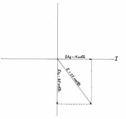
QUESTION #43. How is the phase difference in a series circuit computed by equation when the values of the reactance and resistance are known?
