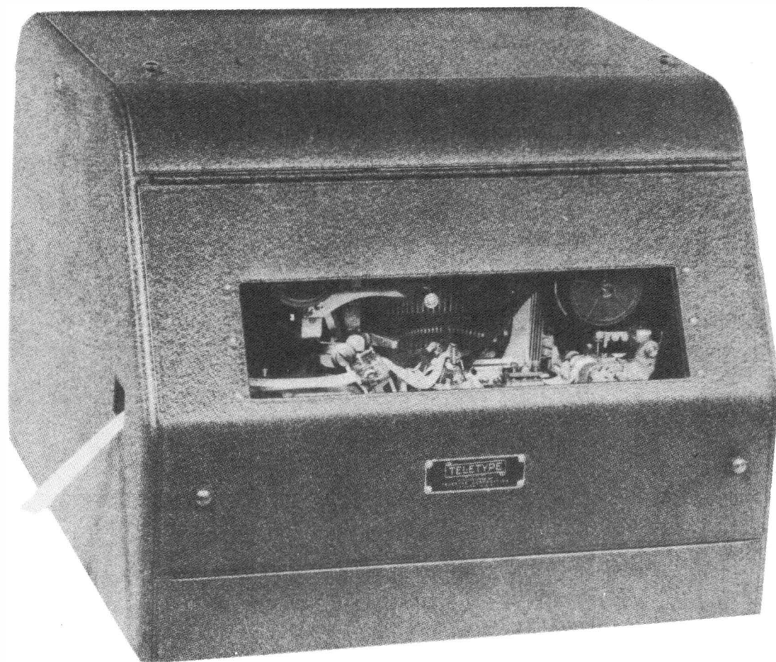
REPERFORATOR TRANSMITTER DISTRIBUTOR WITH COVER (TYPING FRXD 4)
