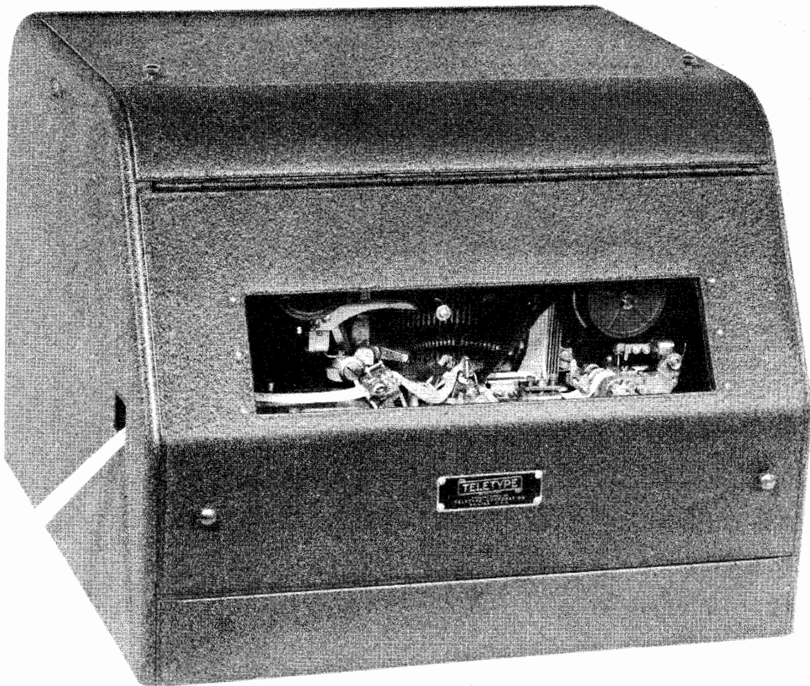
REPERFORATOR TRANSMITTER DISTRIBUTOR WITH COVER (TYPING FRXD4)
