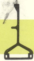
155767 Slide — Used for operating shift fork by one to six, adjacent function levers
