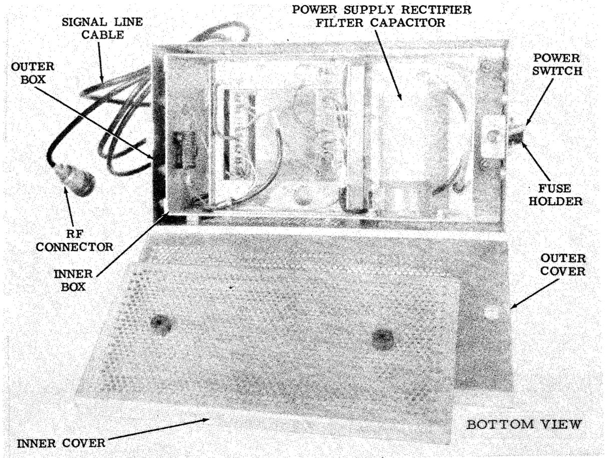
Figure 3-23. Typical Parts of an ESA - Double Box Construction (Sheet 2 of 2)
