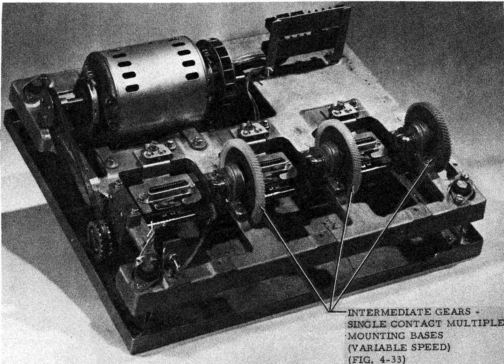
Figure 4-32. Single Contact Multiple Mounting Bases
