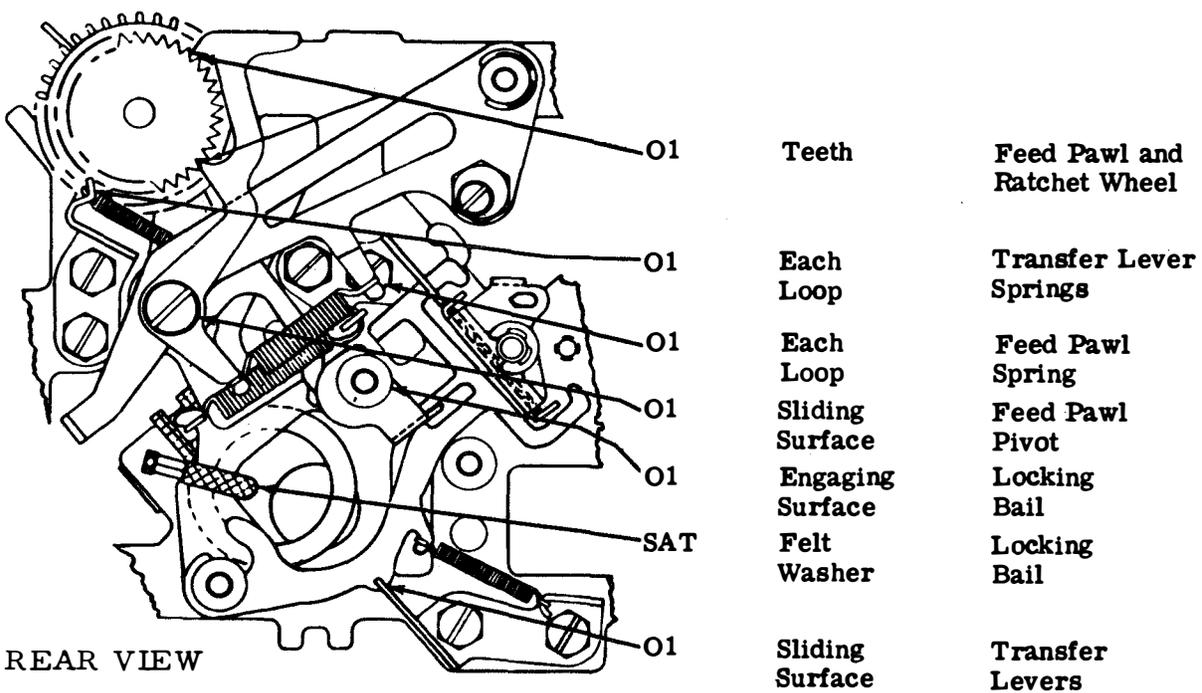
Figure 4-15. Transfer Mechanism
