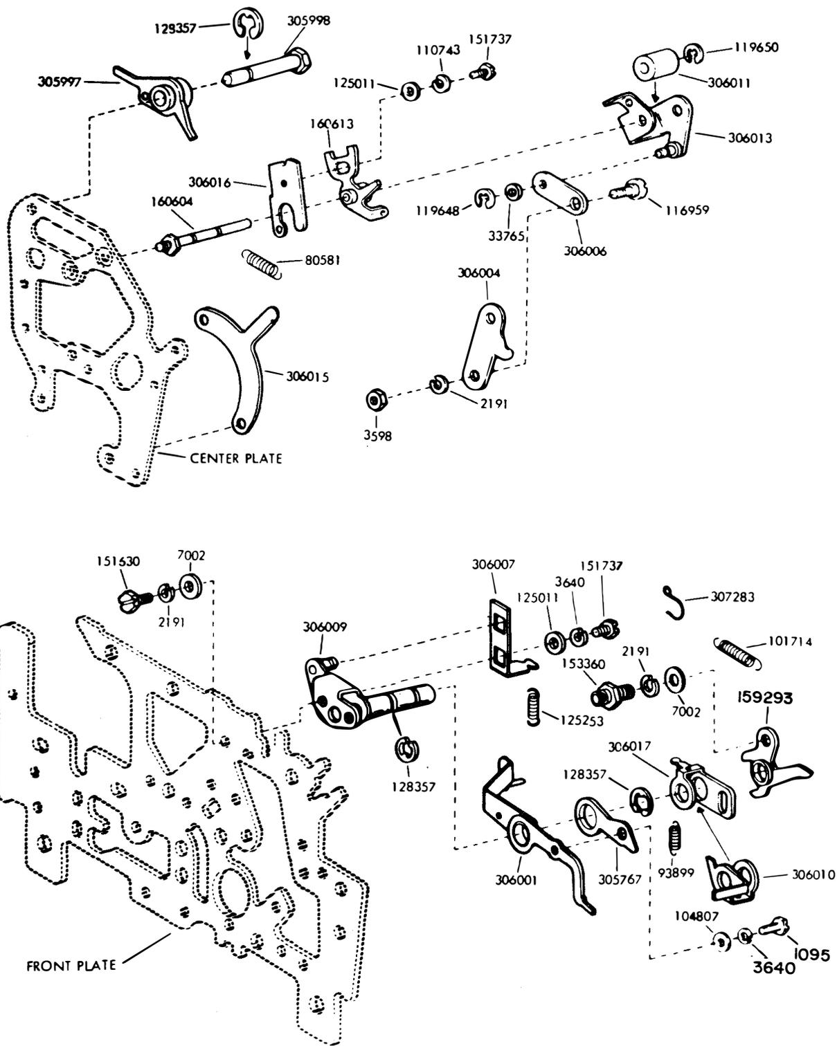
Figure 7-20. Tape-Out Mechanism for Mechanically Coupled Dual Transmitter Distributor (Early Design)
