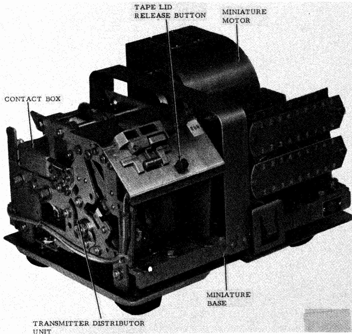
Figure 1-6. Transmitter Distributor Set Model 28 - Miniaturized
