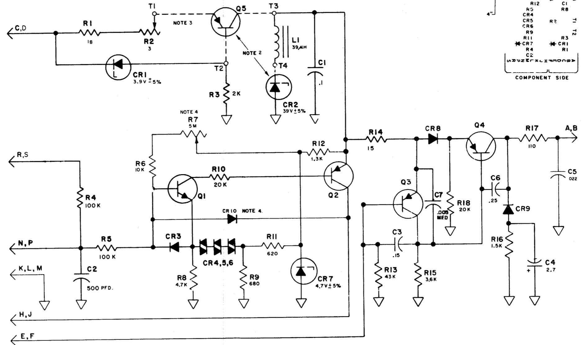
Figure 5-15. Clutch Magnet Driver 321991 Schematic Diagram (Sheet 2 of 2)
