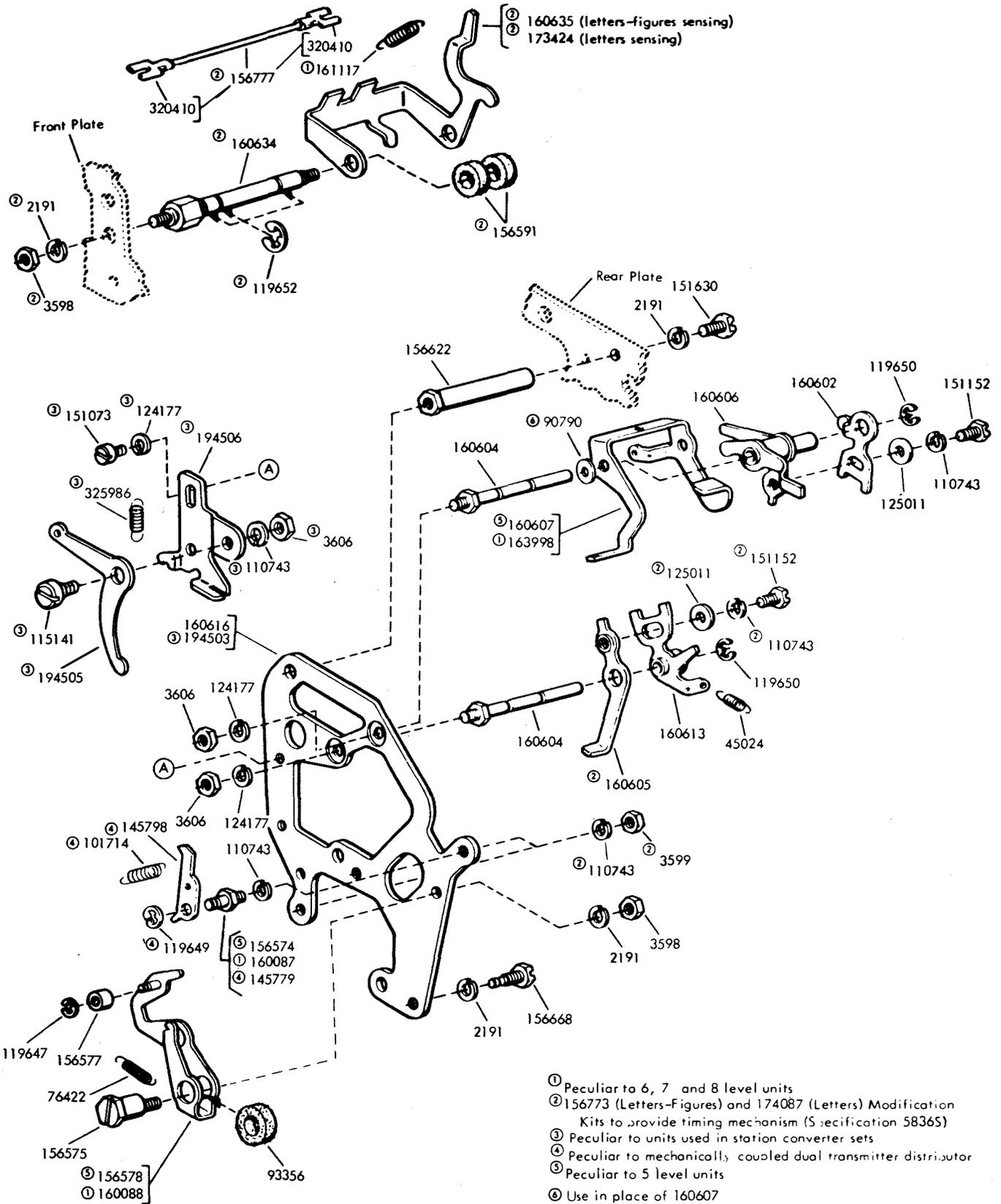
Figure 7-6. Center Plate and Timing Mechanism
