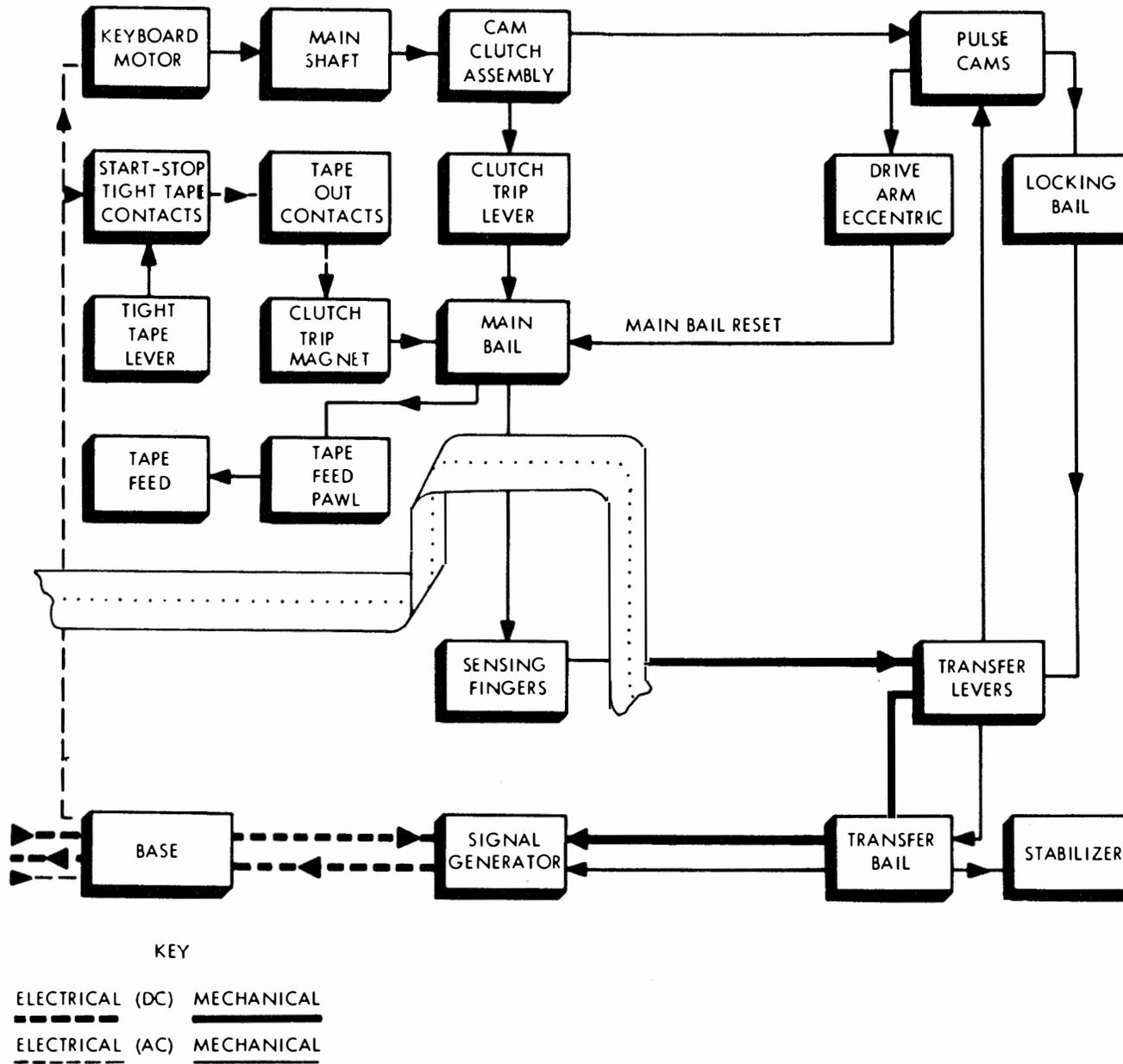
Figure 3-7. TD Functional Block Diagram
