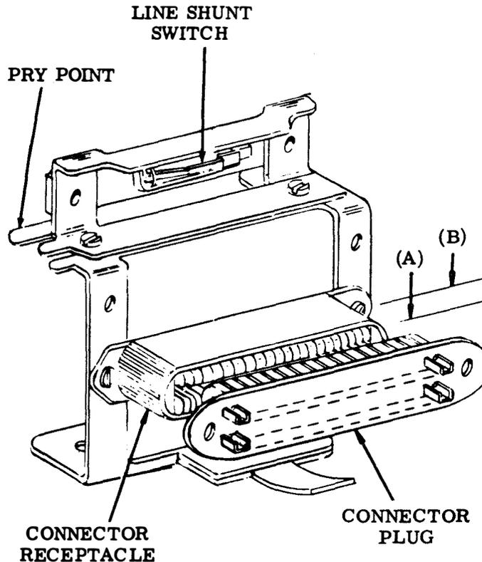
Figure 6-47. Line Shunt Switch
