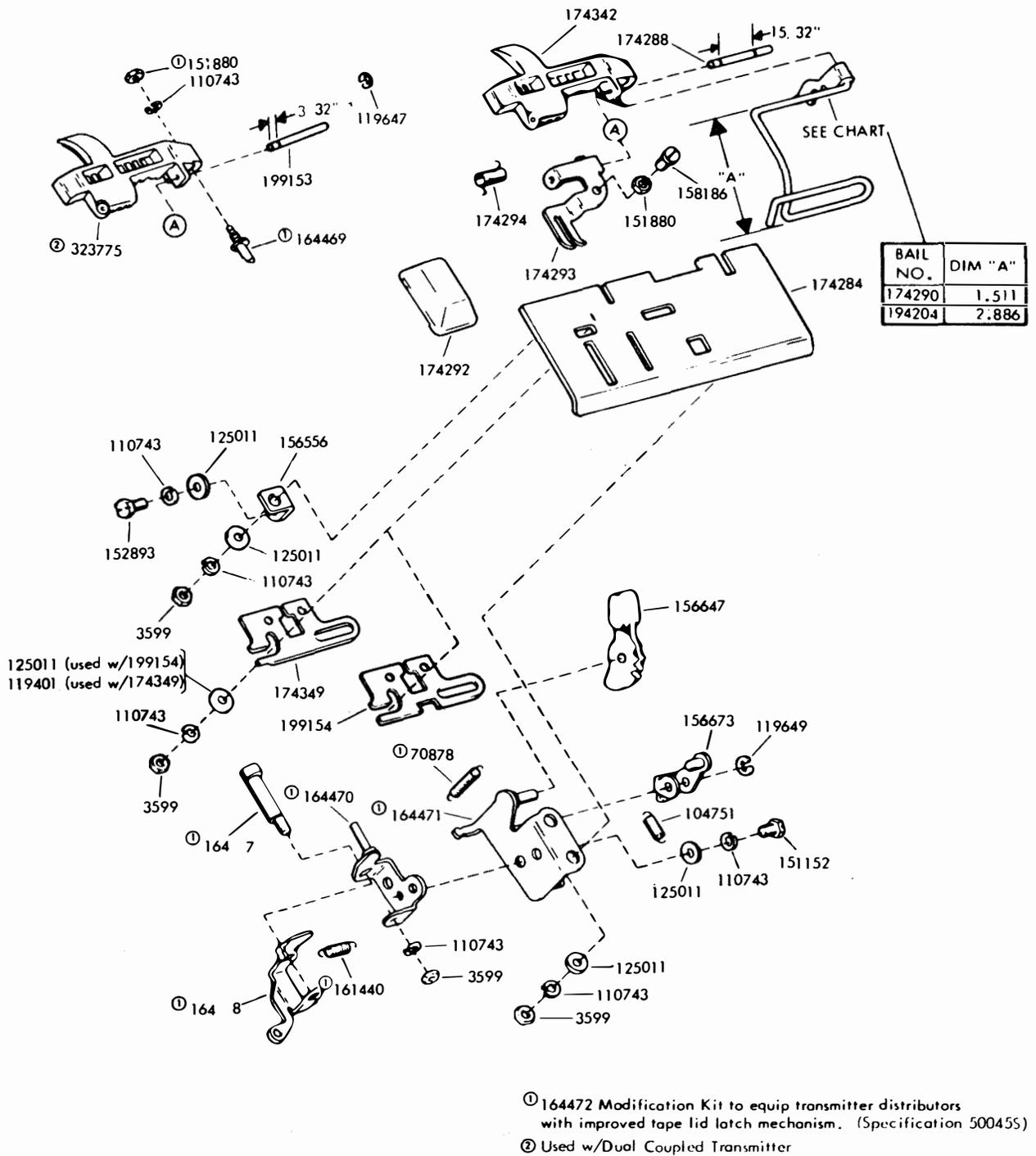
Figure 7-16. Tape Guide Plate Mechanisms (Sheet 2 of 3)
