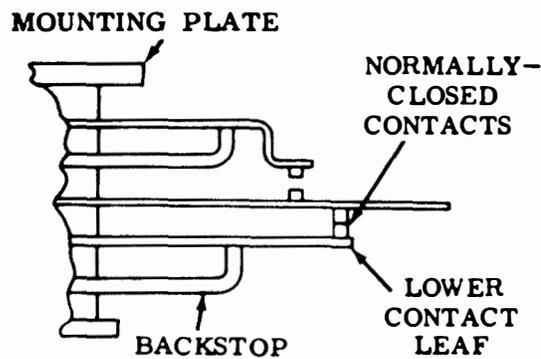
Figure 6-54. Normally-Closed Contacts - Backstop
