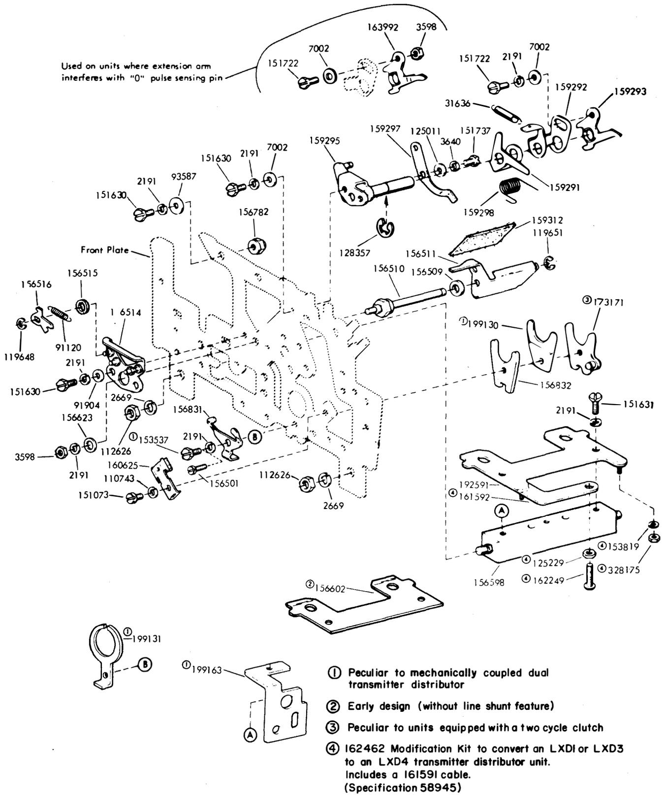
Figure 7-2. Front Plate Mechanism (Sheet 2 of 3)
