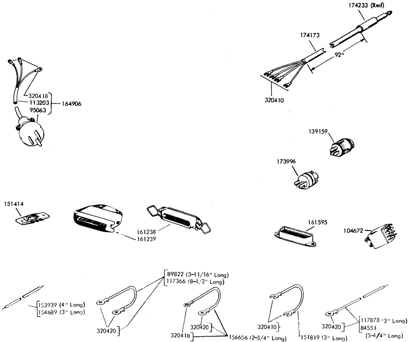
Figure 7-32. Cable Components
