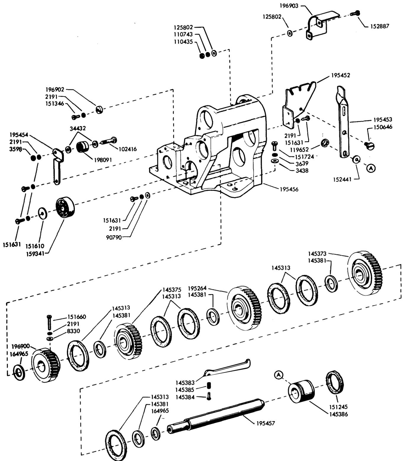
Figure 7-35. Modification Kits 195442 and 195443 to Add Three-Speed Gearshift Assemblies (Sheet 2 of 3)
