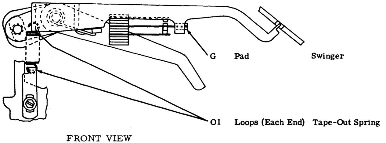
Figure 4-17. Tape-Out Sensing Mechanism (Variable Features)
