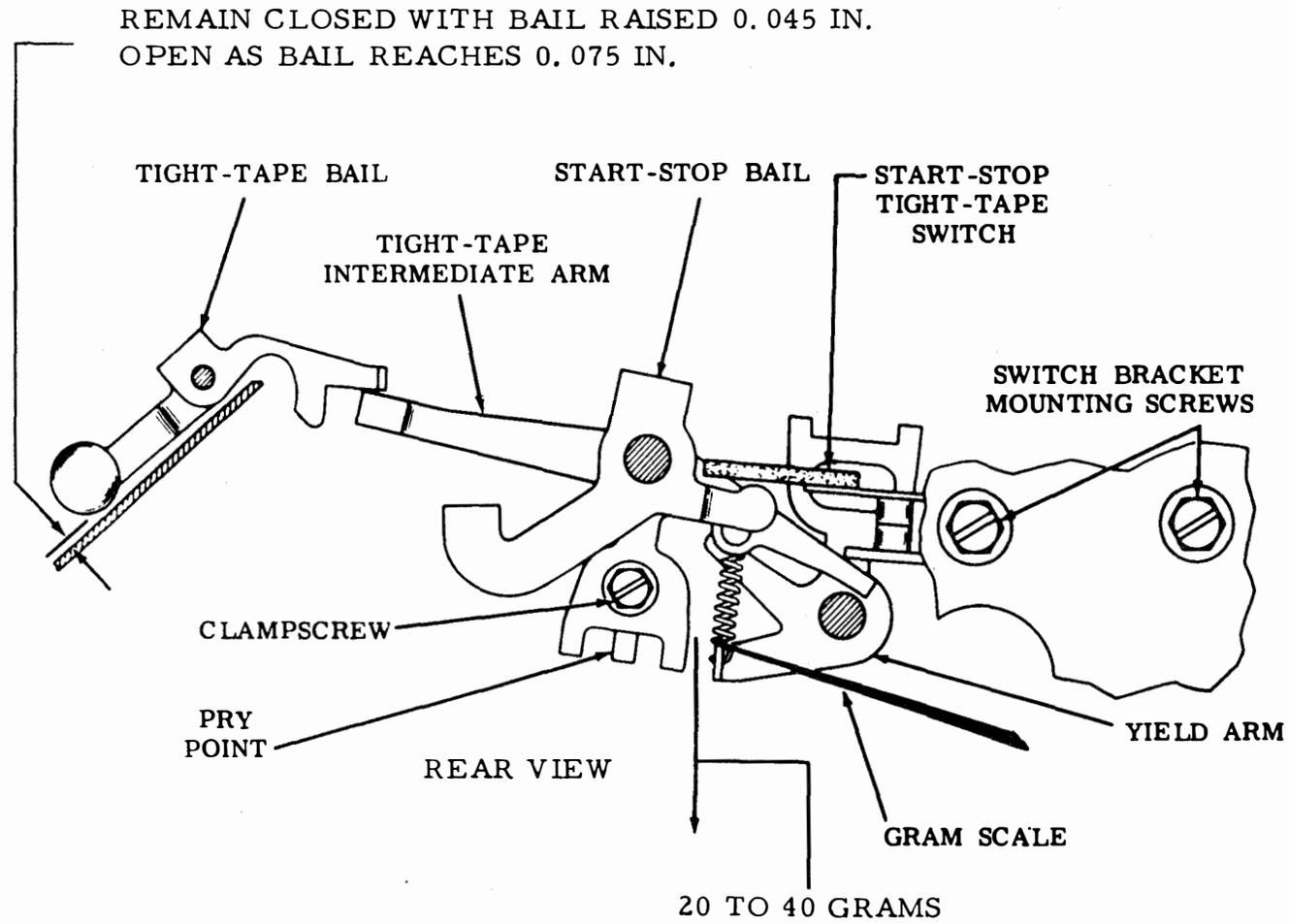
Figure 6-21. Tight-Tape Intermediate Arm and Tight-Tape Arm Spring
