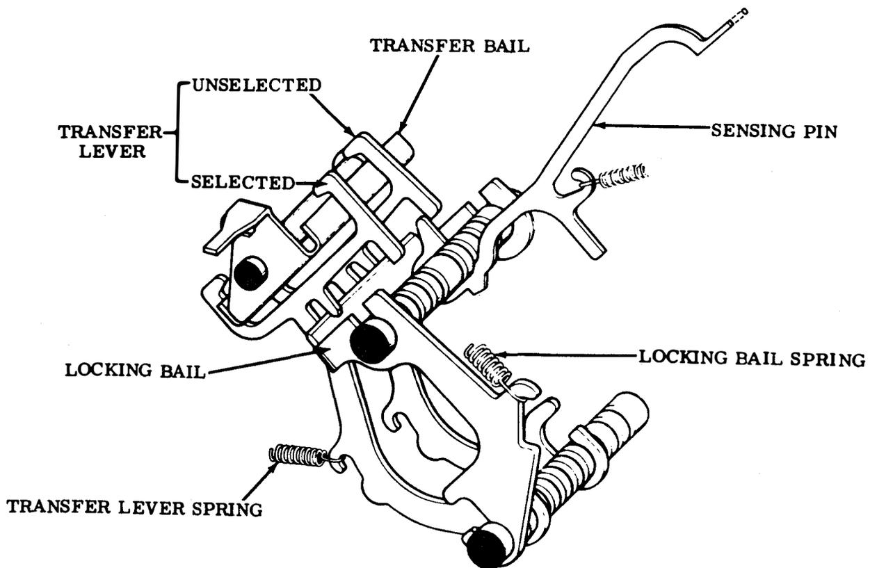
Figure 3-11. Locking Bail and Transfer Lever Mechanisms
