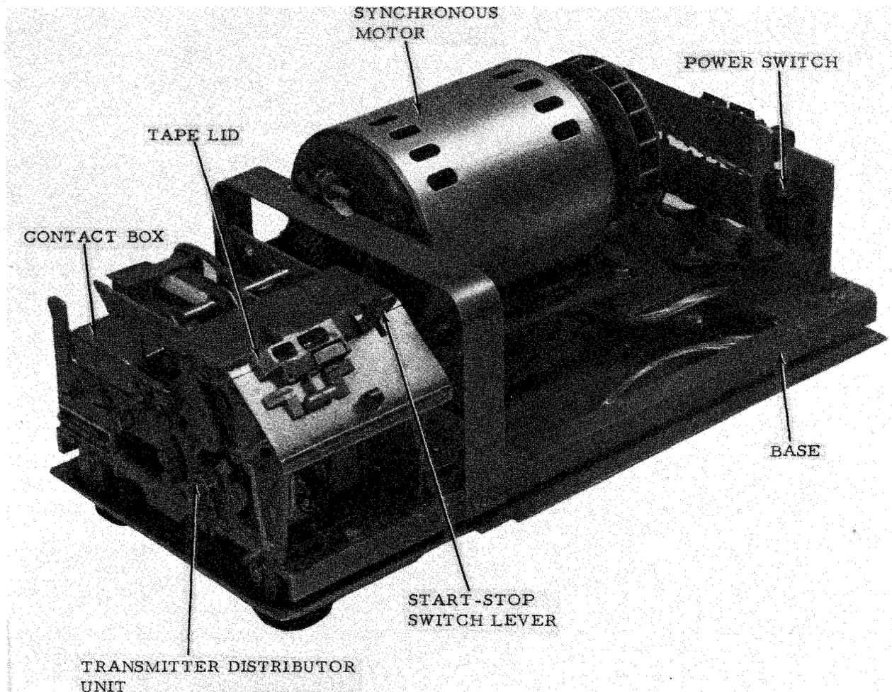
Figure 1-5. Transmitter Distributor Set Model 28 - Regular Size (Cover, Cover Plate, and Panel Removed)
