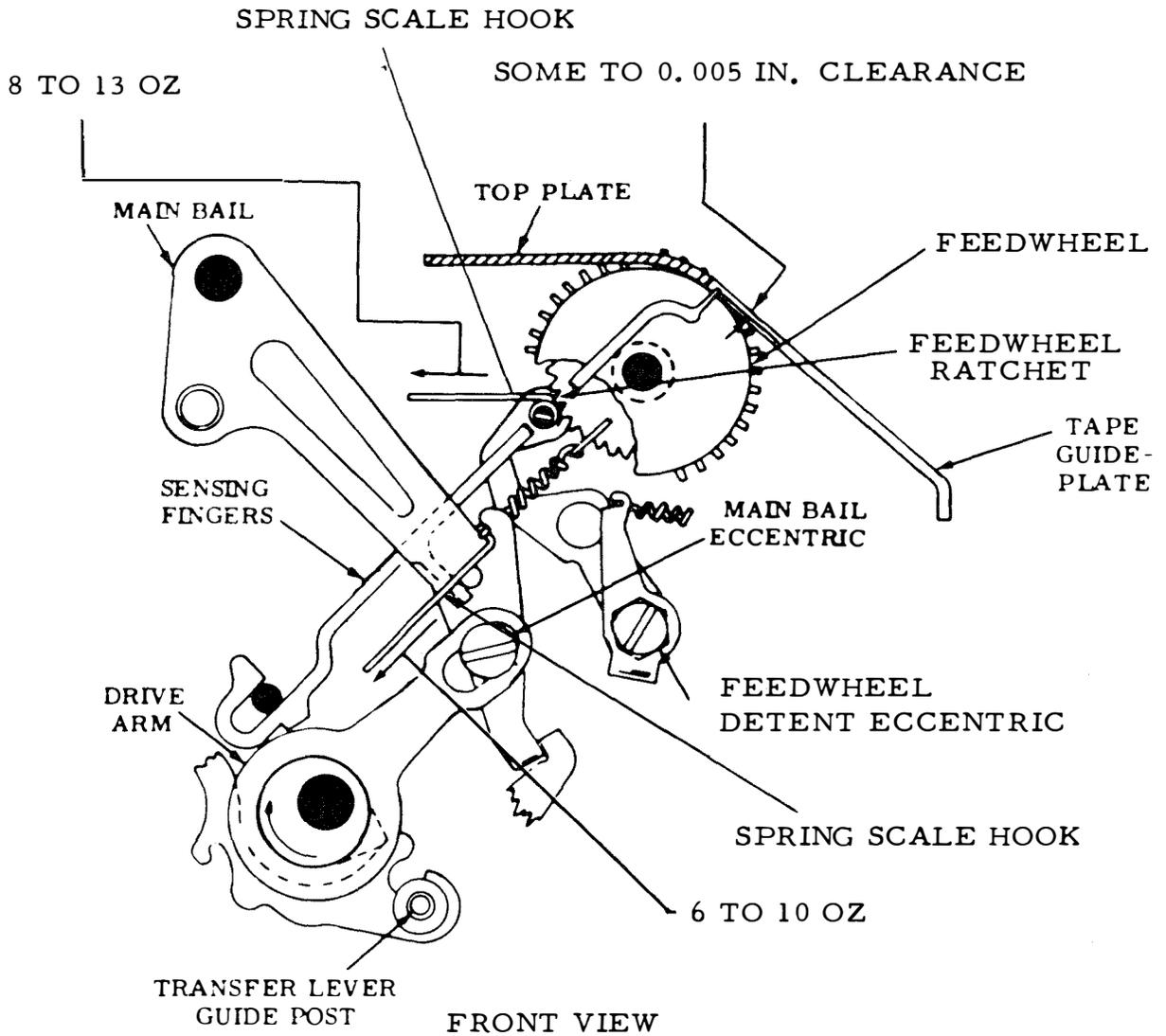
Figure 6-22. Main Bail Spring, Feed Ratchet Detent Spring and Main Bail Trip Lever
