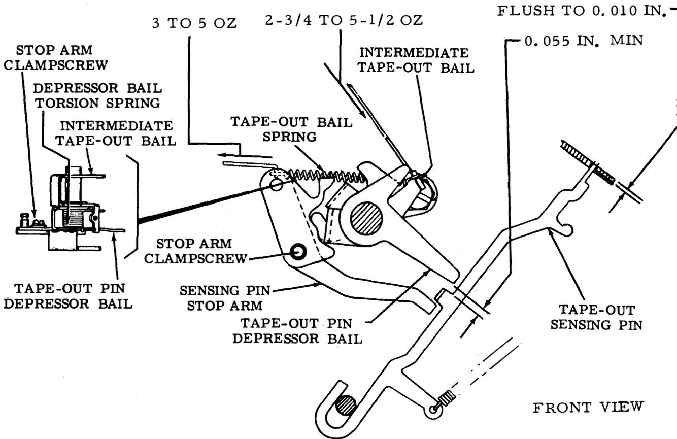
Figure 6-17. Tape-Out Sensing Pin, Depressor Bail Torsion Spring, and Intermediate Tape-Out Bail Spring
