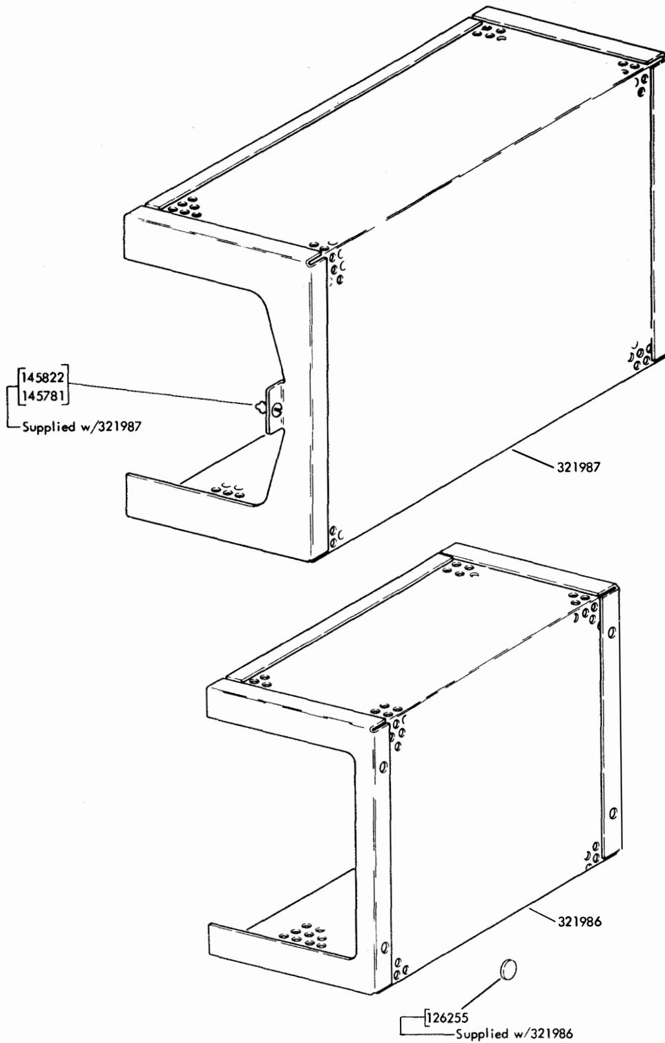
Figure 7-48. Electrical Service Assembly Covers (Sheet 1 of 2)
