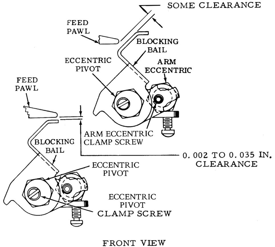
Figure 6-73. Blocking Bail Arm Eccentric and Blocking Bail Eccentric Pivot
