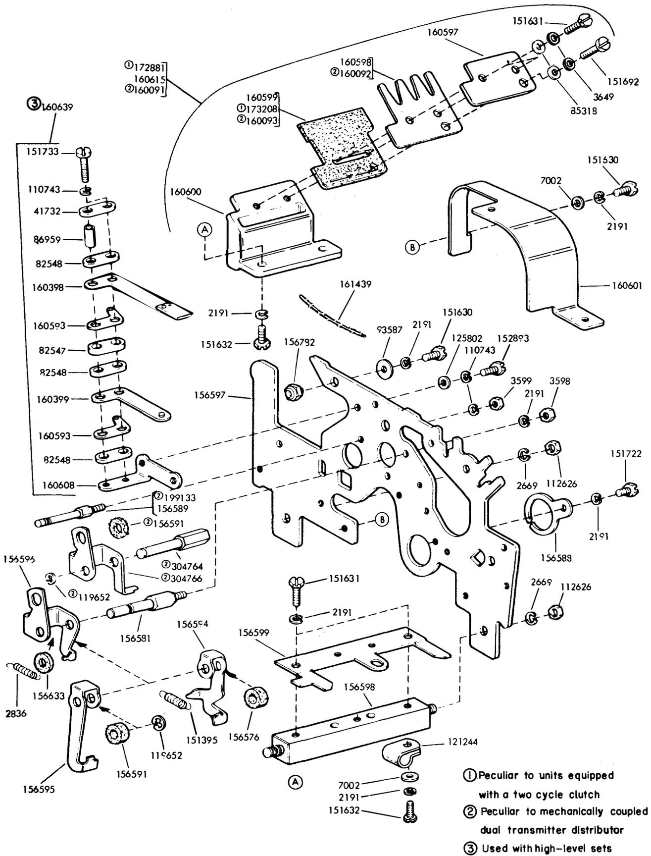
Figure 7-7. Rear Plate Mechanism
