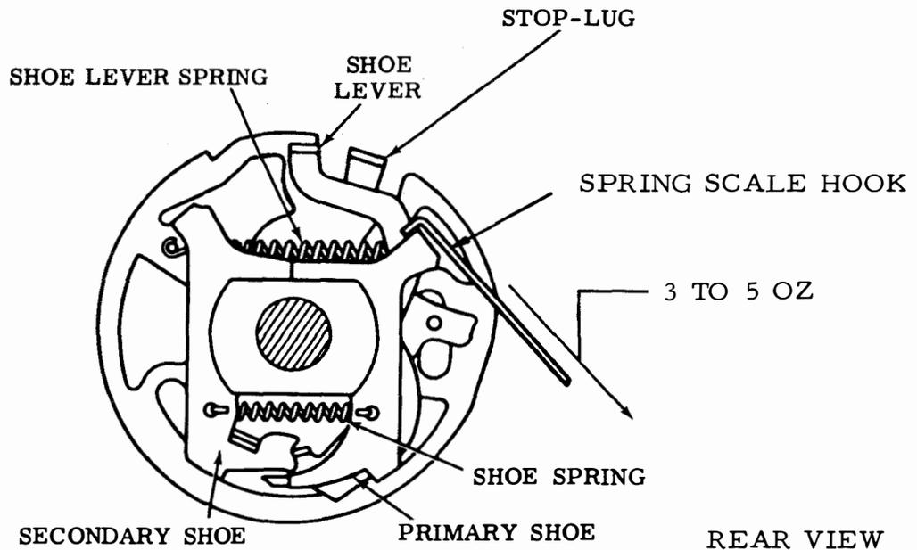
Figure 6-2. Clutch Shoe Spring
