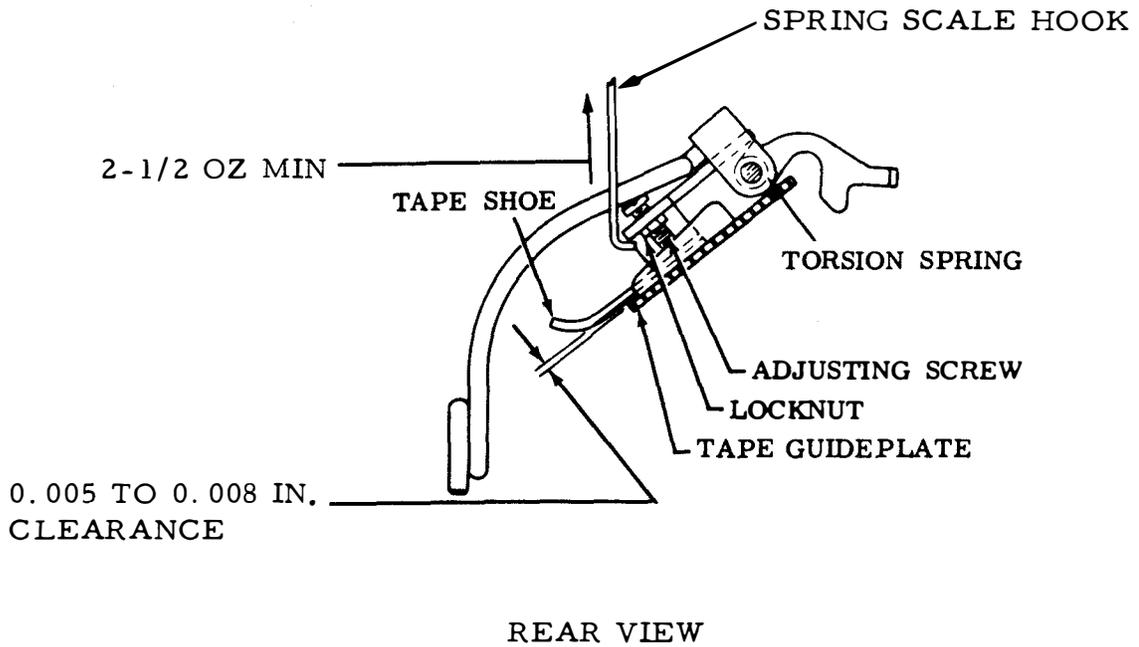
Figure 6-50. Torsion Spring and Tape Shoe
