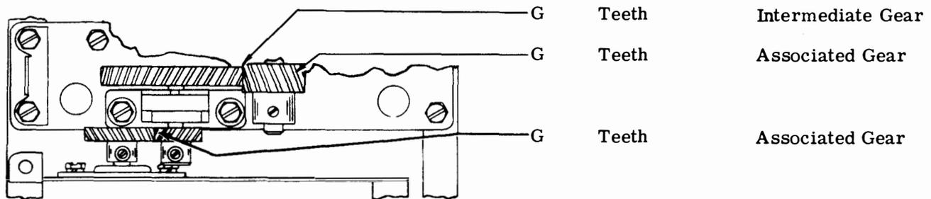
Figure 4-29. Intermediate Gear - Multicontact Single Mounting Bases
