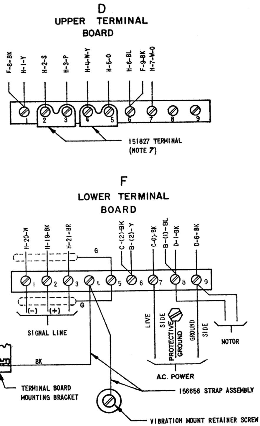
Figure 5-8. Transmitter Distributor Base LXDB19 Wiring Diagram
