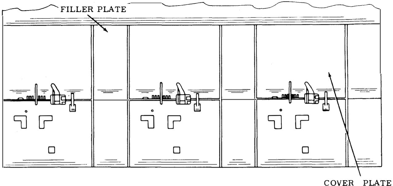
Figure 6-48. Cover Plates and Filler Plates
