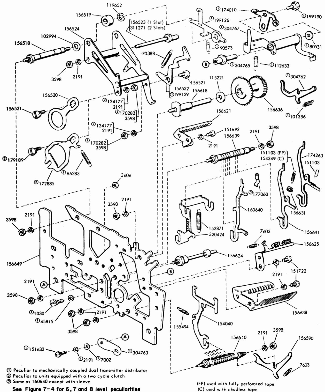
Figure 7-1. Front Plate Mechanism (Sheet 1 of 3)
