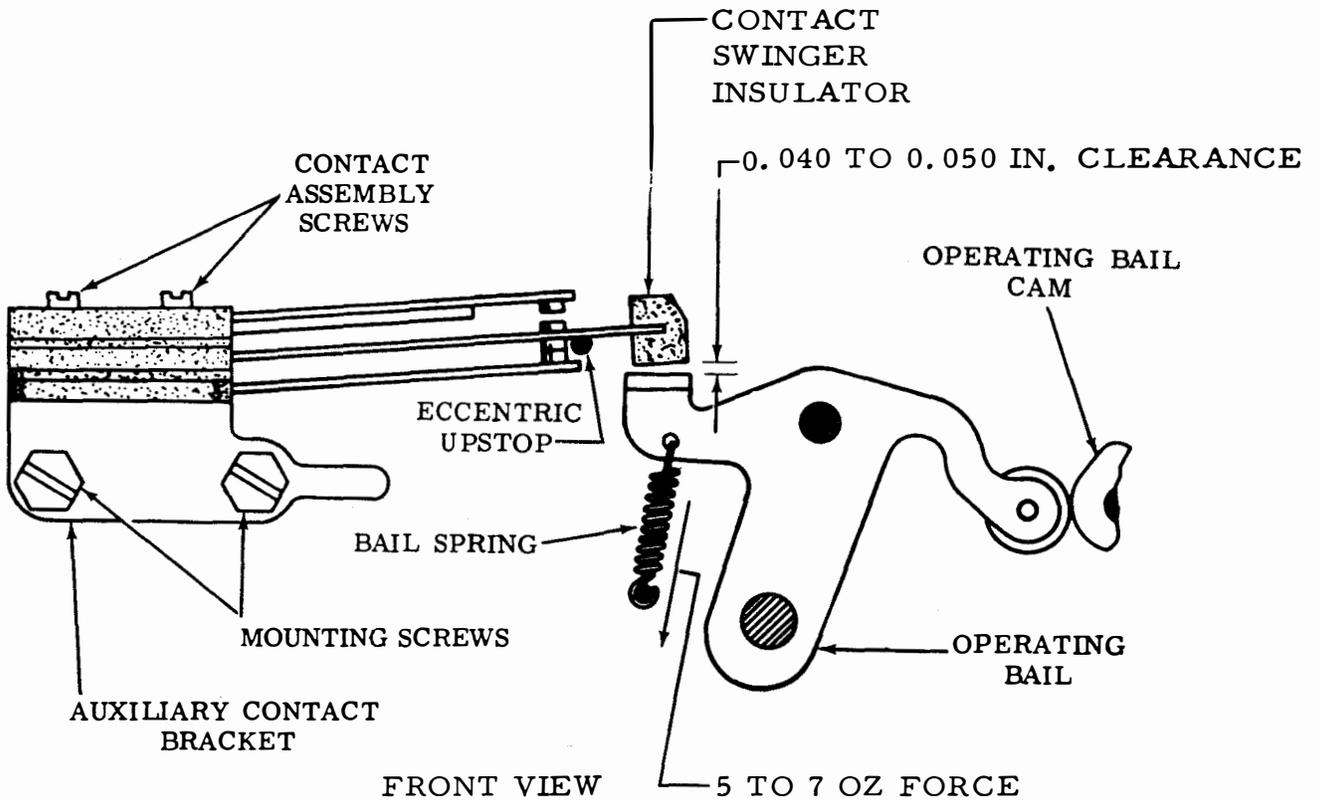
Figure 6-62. Contact Sensing Arm and Auxiliary Contact Operating Bail Spring
