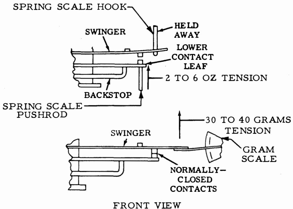
Figure 6-55. Normally-Closed Contacts - Spring
