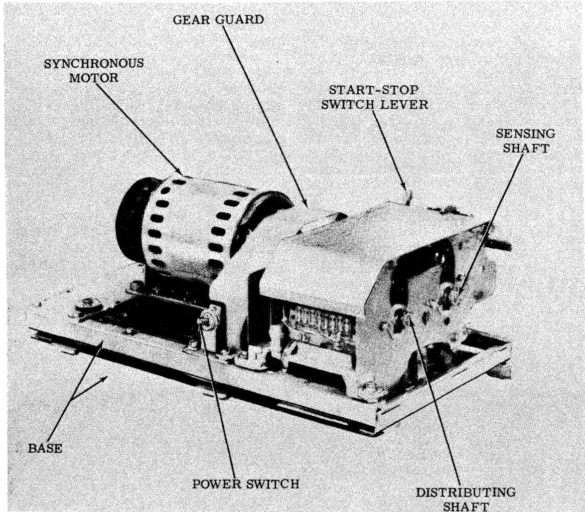
Figure 1-7. Transmitter Distributor Set Model 28 - Regular Size, Multicontact (Cover Removed)
