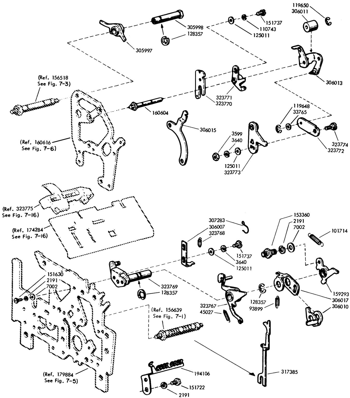
Figure 7-19. Tape-Out Mechanism for Mechanically Coupled Dual Transmitter Distributor
