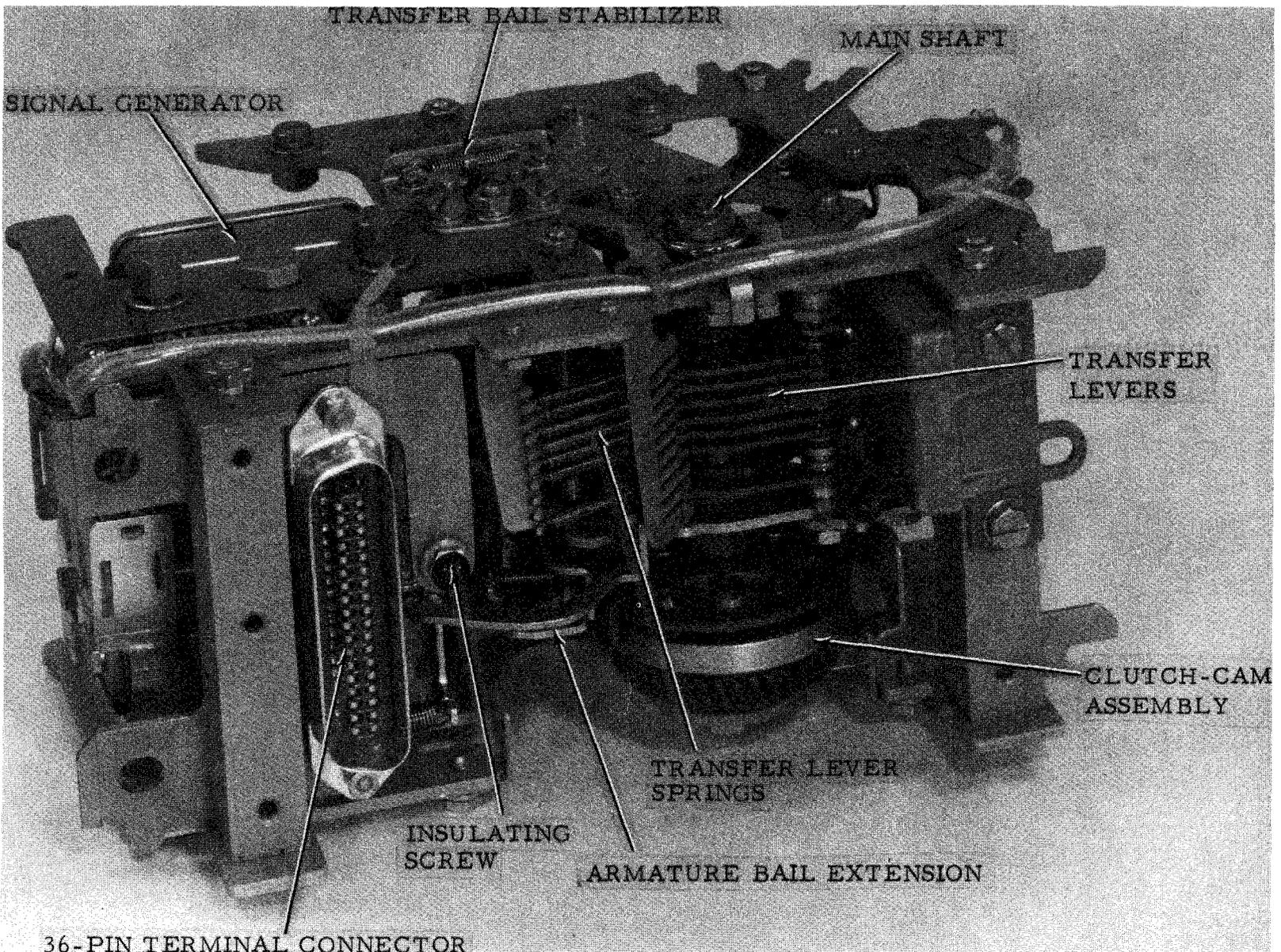
Figure 3-5. Transmitter Distributor Unit - Bottom View
