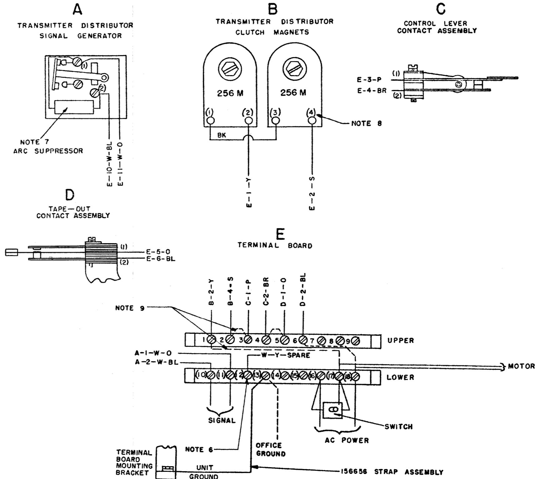
Figure 5-1. Transmitter Distributor Unit LXD1 Wiring Diagram
