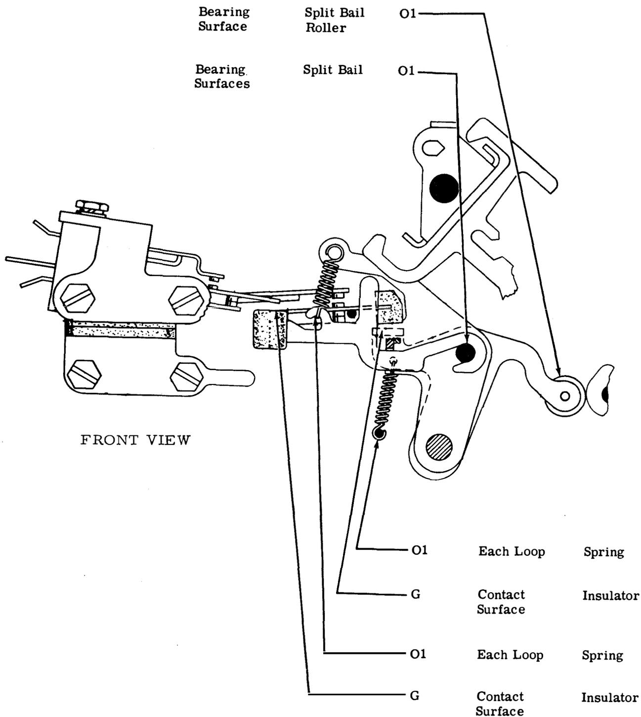
Figure 4-18. Code Reading Contacts (Variable Features)
