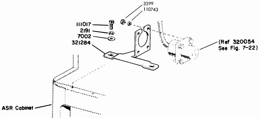
Figure 7-23. Mounting Components for Contact Box Cable - RFI Suppression Features for Low-Level Sets
