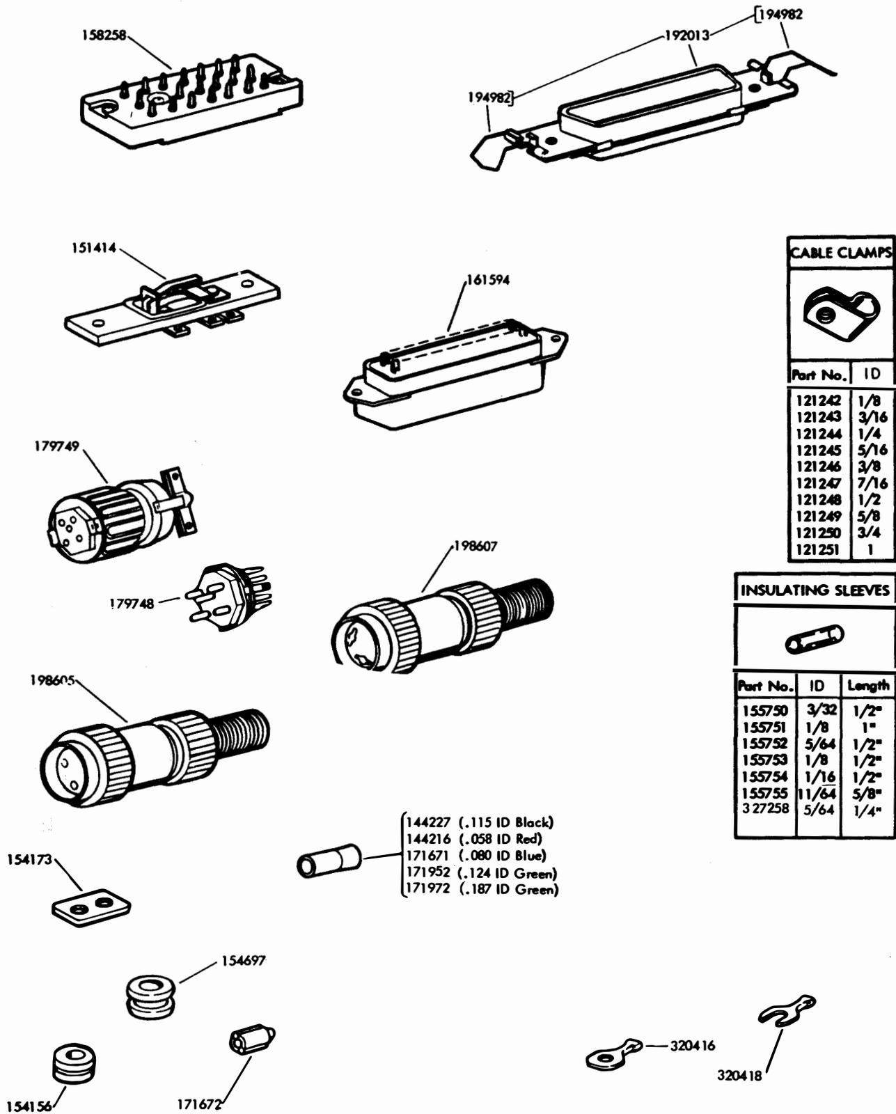
Figure 7-21. Cable Components
