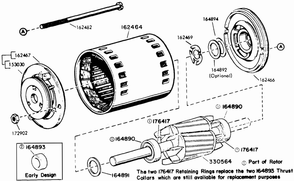
Figure 7-39. Synchronous Motor Assembly 151795 (Standard) - Used on LMU3 and LMU38
