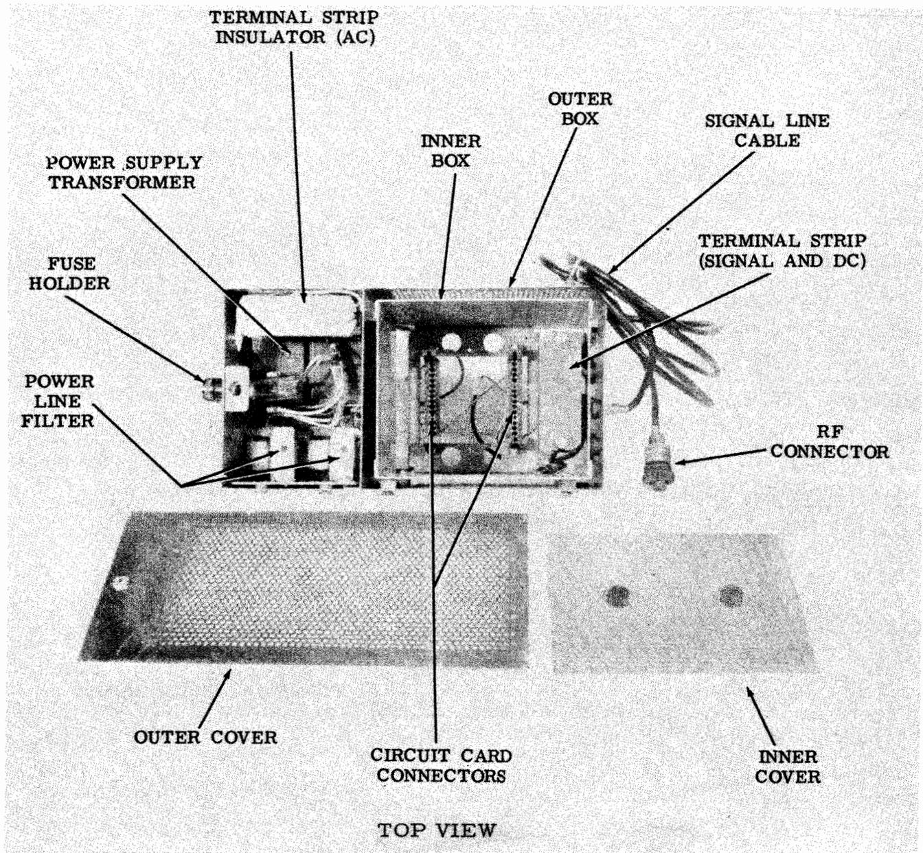
Figure 3-23. Typical Parts of an ESA - Double Box Construction (Sheet 1 of 2)
