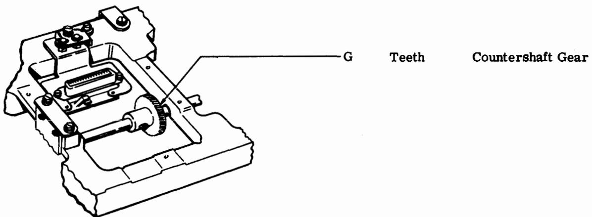
Figure 4-31. Countershaft Gear - Single Contact Multiple Mounting Bases (Common Speed)
