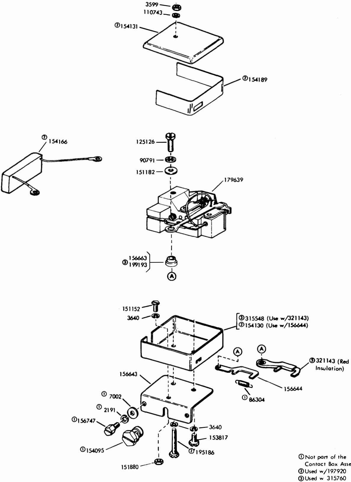
Figure 7-12. Contact Box Assemblies - 192600 (Neutral Transmission), 197920 (Neutral Transmission with Arc Suppression), 305008 (Polar Transmission), and 315760 (Polar Transmission with Insulated Drive)
