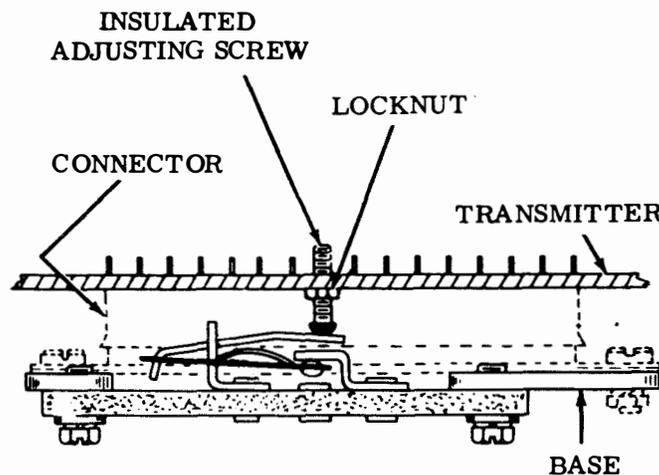
Figure 6-34. Line Shunt Switch
