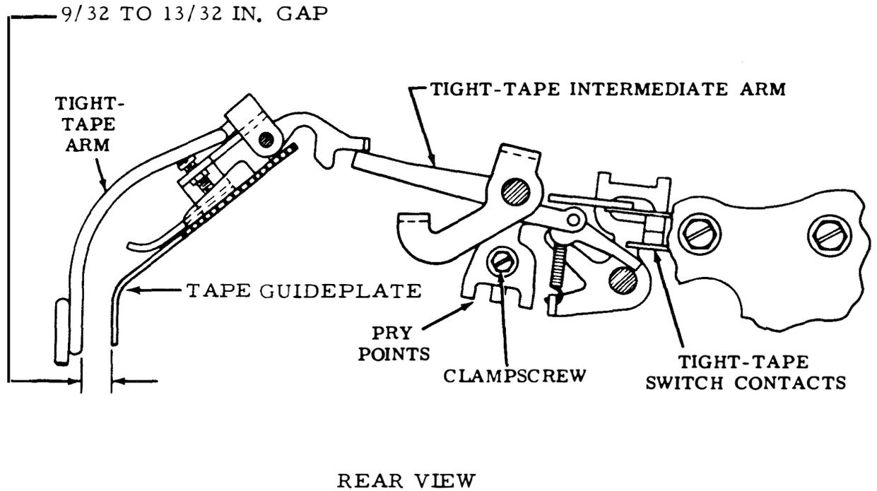
Figure 6-49. Tight-Tape Switch
