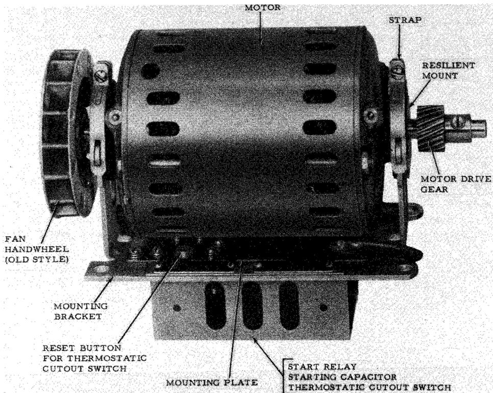
Figure 1-18. Typical Standard or Heavy Duty Synchronous Motor Unit
