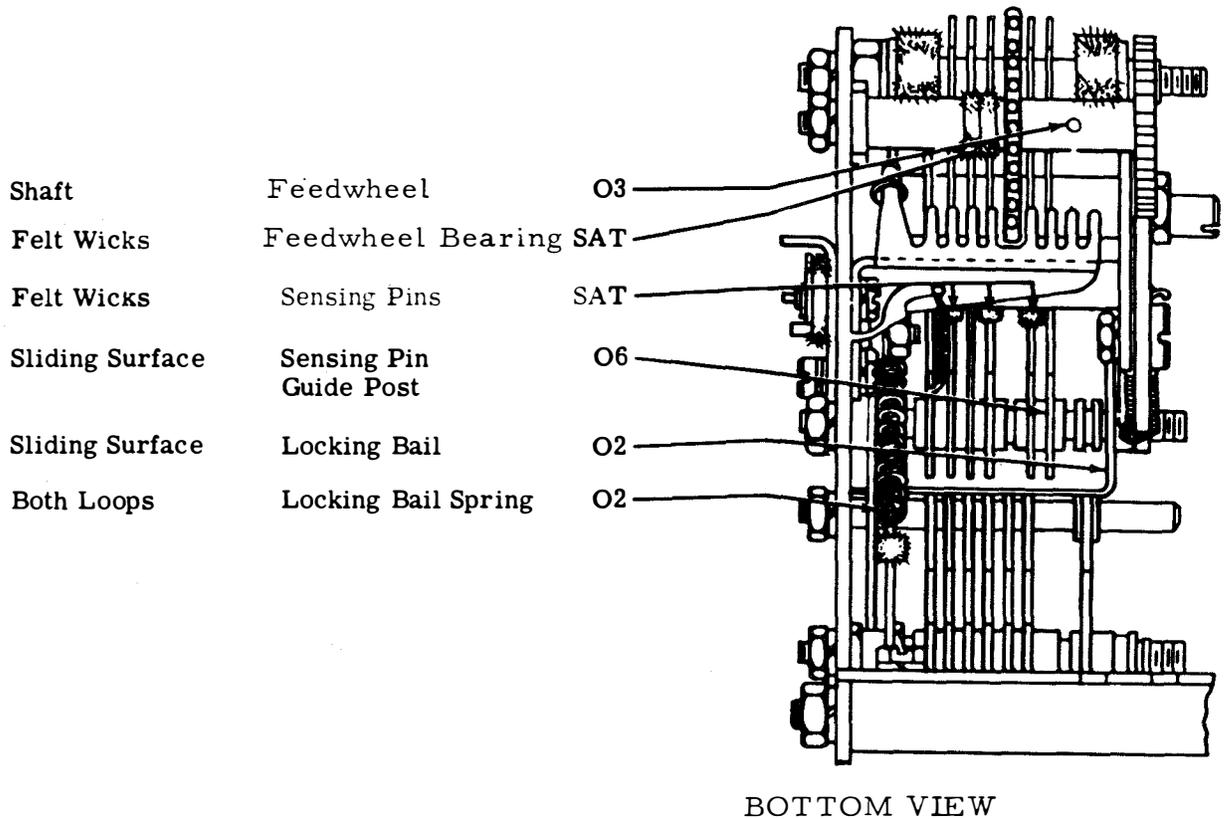
Figure 4-14. Sensing and Feed Assembly
