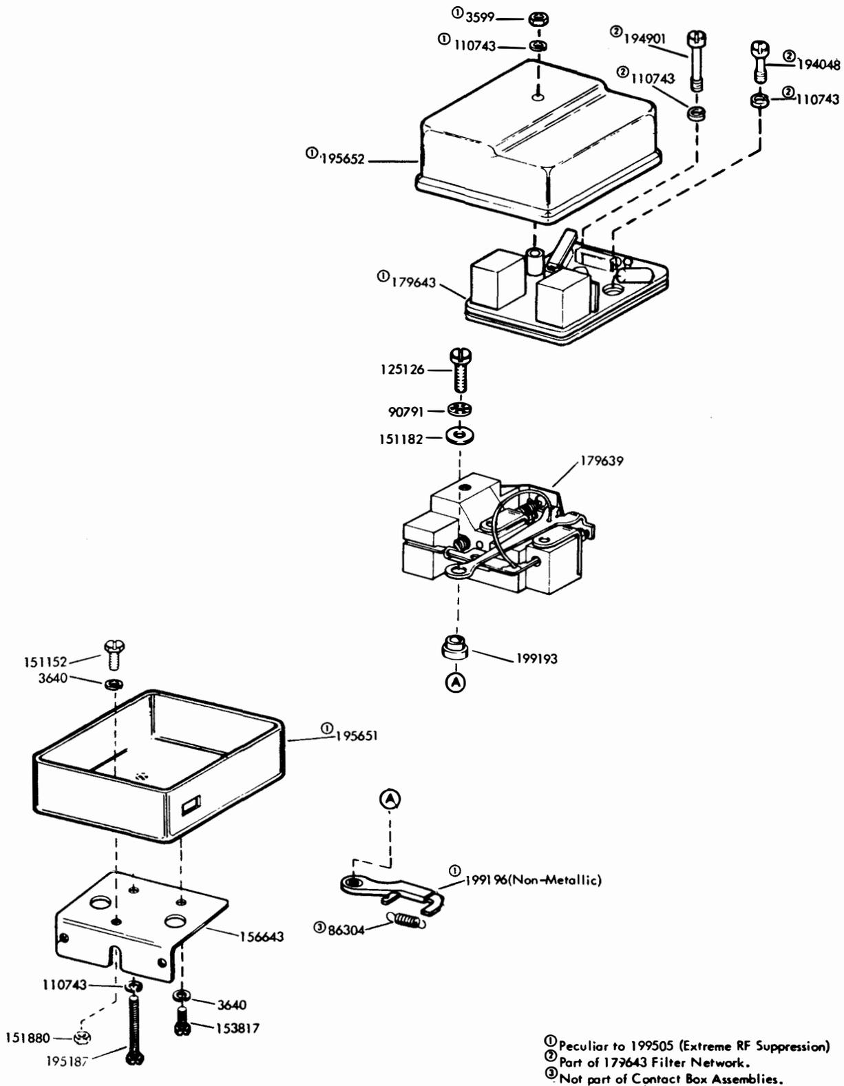
Figure 7-11. Contact Box Assemblies - 198610 (Low-Level Keyer) and 199505 (Extreme RF Suppression)
