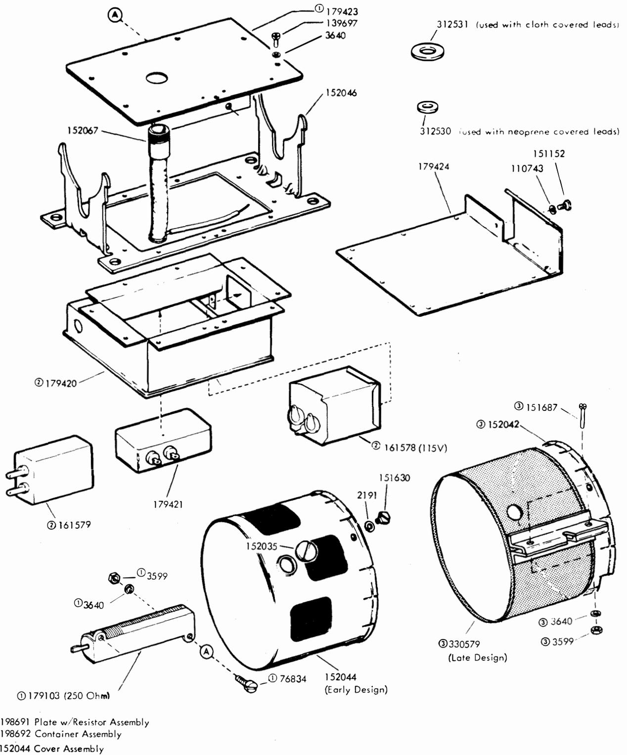
Figure 7-47. Series Motor Mounting Parts with RF Suppression - Used on LMU39 and LMU41
