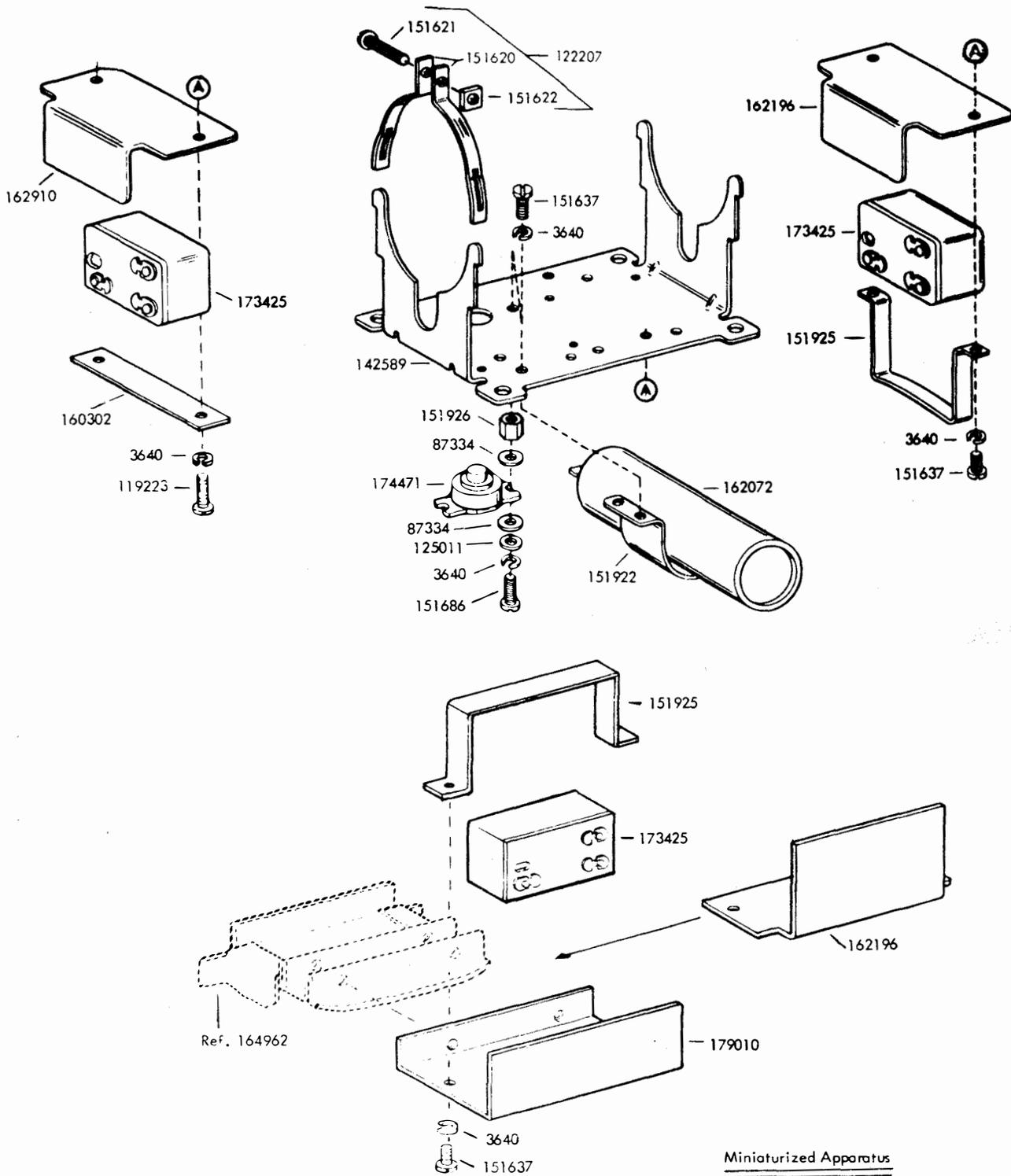
Figure 7-42. Relay and Capacitor Mounting (Synchronous) Used on LMU19
