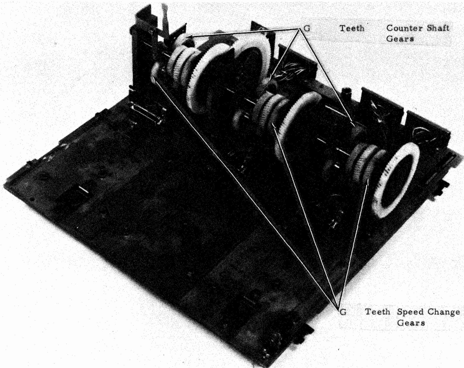
Figure 4-36. Drive Gears and Speed Change Gears - Multicontact Multiple Mounting Bases (Variable Speed)
