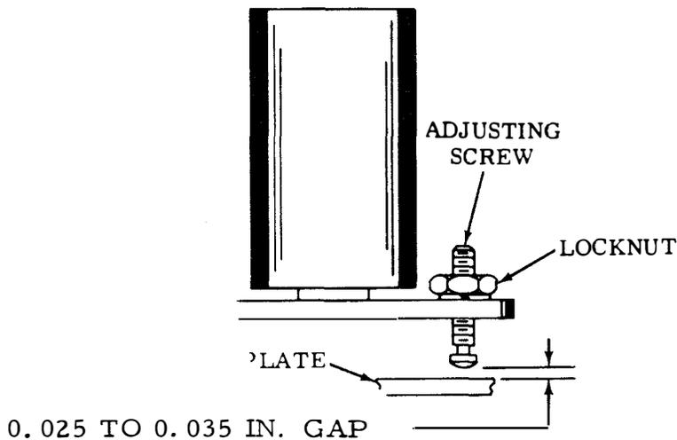
Figure 6-72. Magnet Armature Gap
