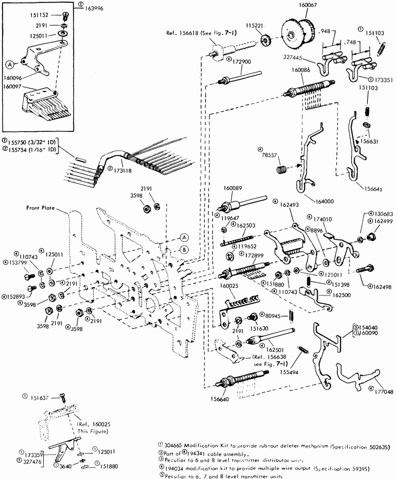
Figure 7-4. Front Plate Mechanism (6, 7, and 8 Level Units)
