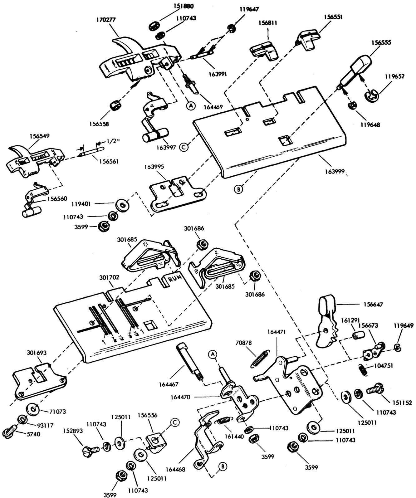
Figure 7-17. Tape Guide Plate Mechanisms (Sheet 3 of 3)
