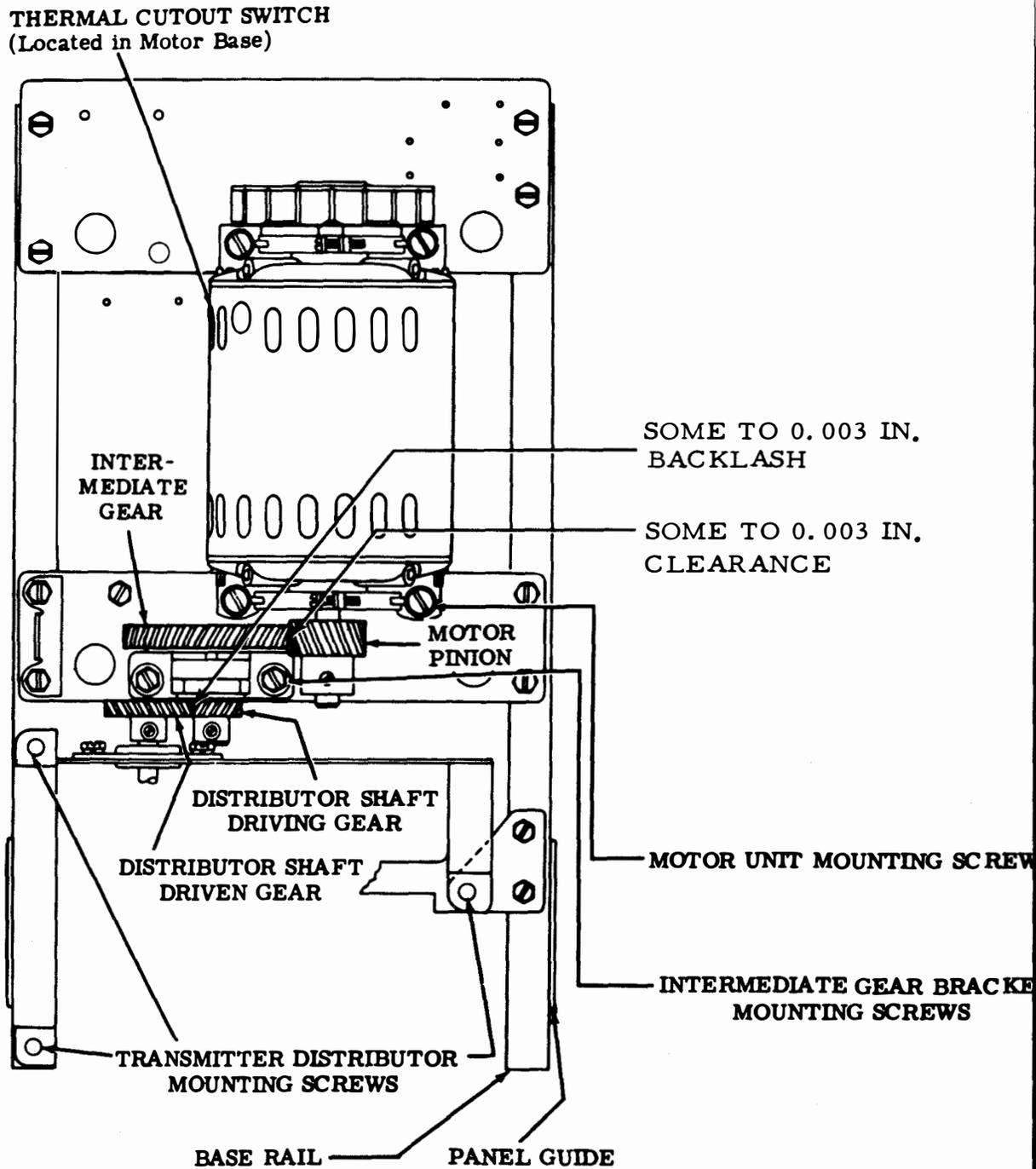
Figure 6-40. Intermediate Gear Assembly and Motor Pinion
