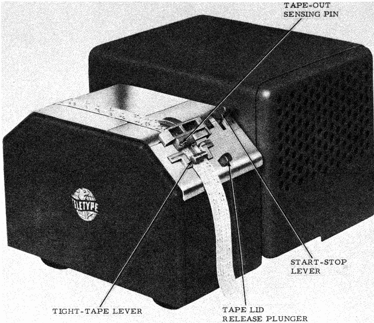
Figure 2-1. TD Set Controls and Indicators
