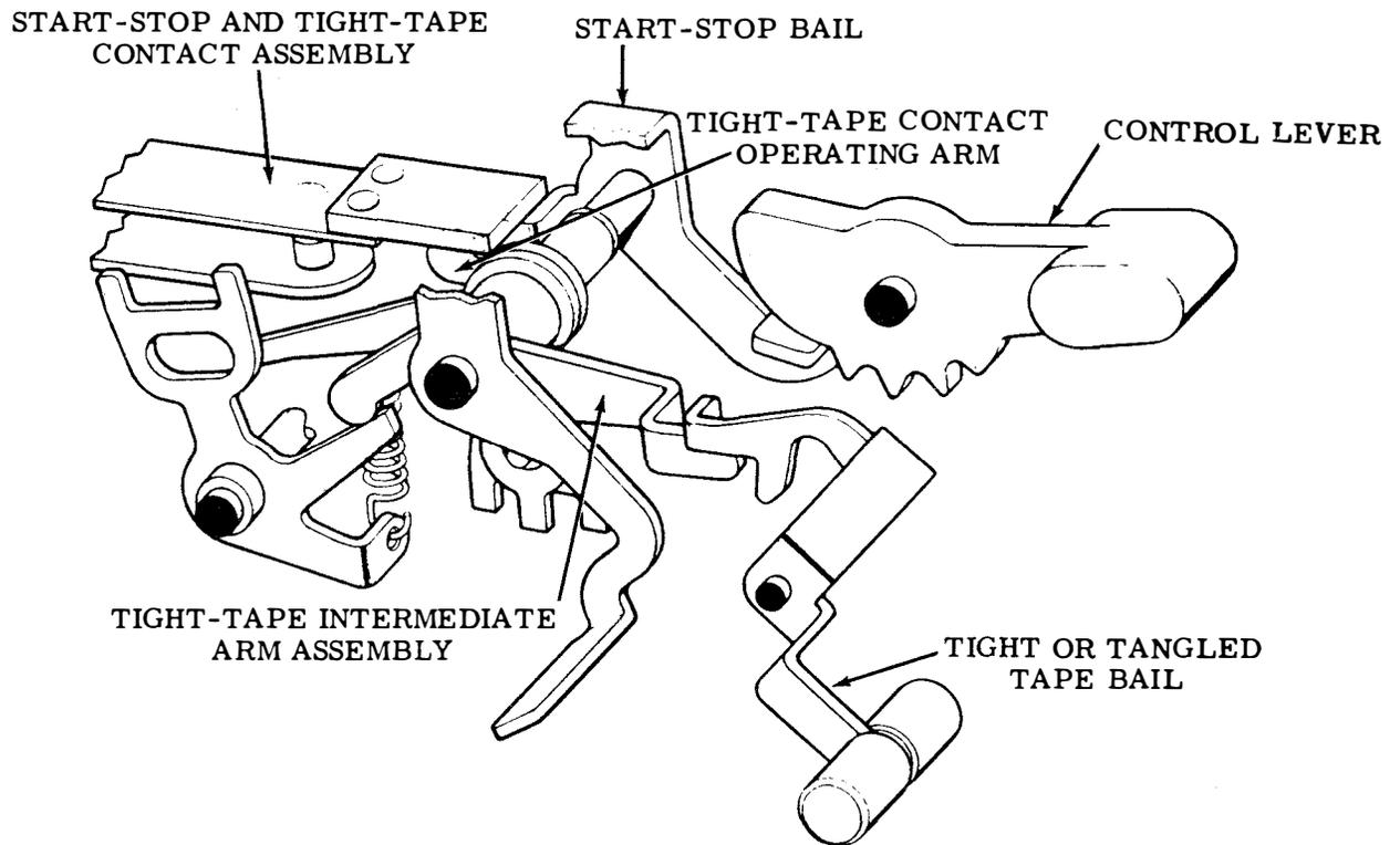
Figure 3-8. Start-Stop and Tight-Tape Switch Mechanisms
