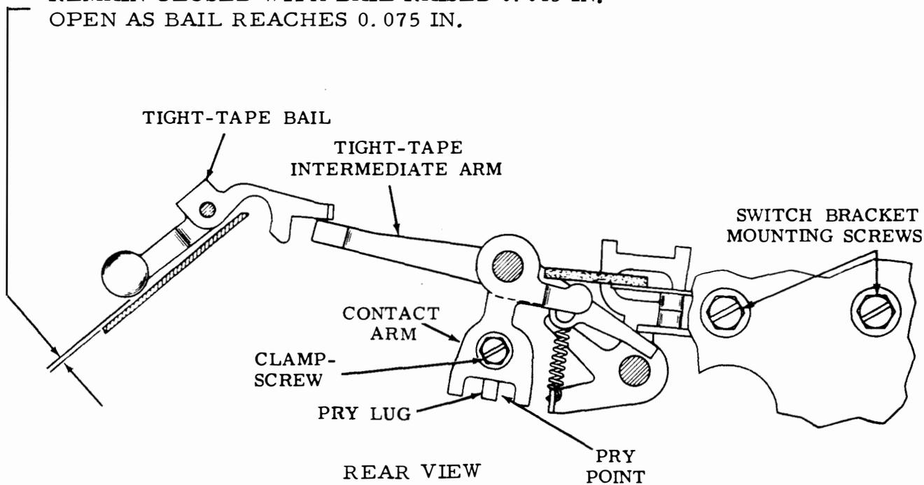
Figure 6-20. Start-Stop Switch Bracket (for Units Equipped with Tape Lid Sensing Lever)
