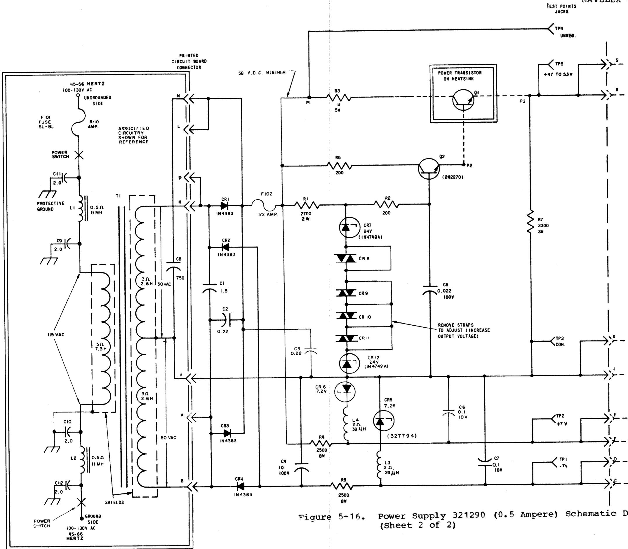
Figure 5-16. Power Supply 321290 (0.5 Ampere) Schematic Diagram (Sheet 2 of 2)
