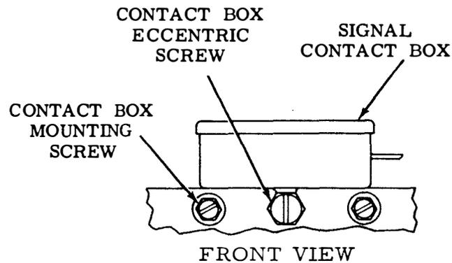
Figure 6-31. Signal Contacts - Electrical
