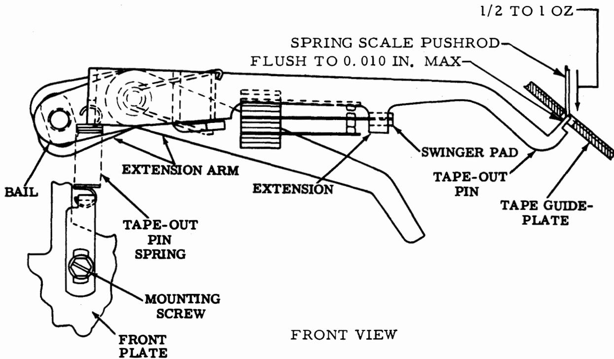
Figure 6-53. Tape-Out Pin Spring and Tape-Out Pin
