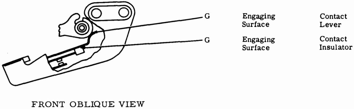
Figure 4-21. Start-Stop Pulse Contact (Variable Features)
