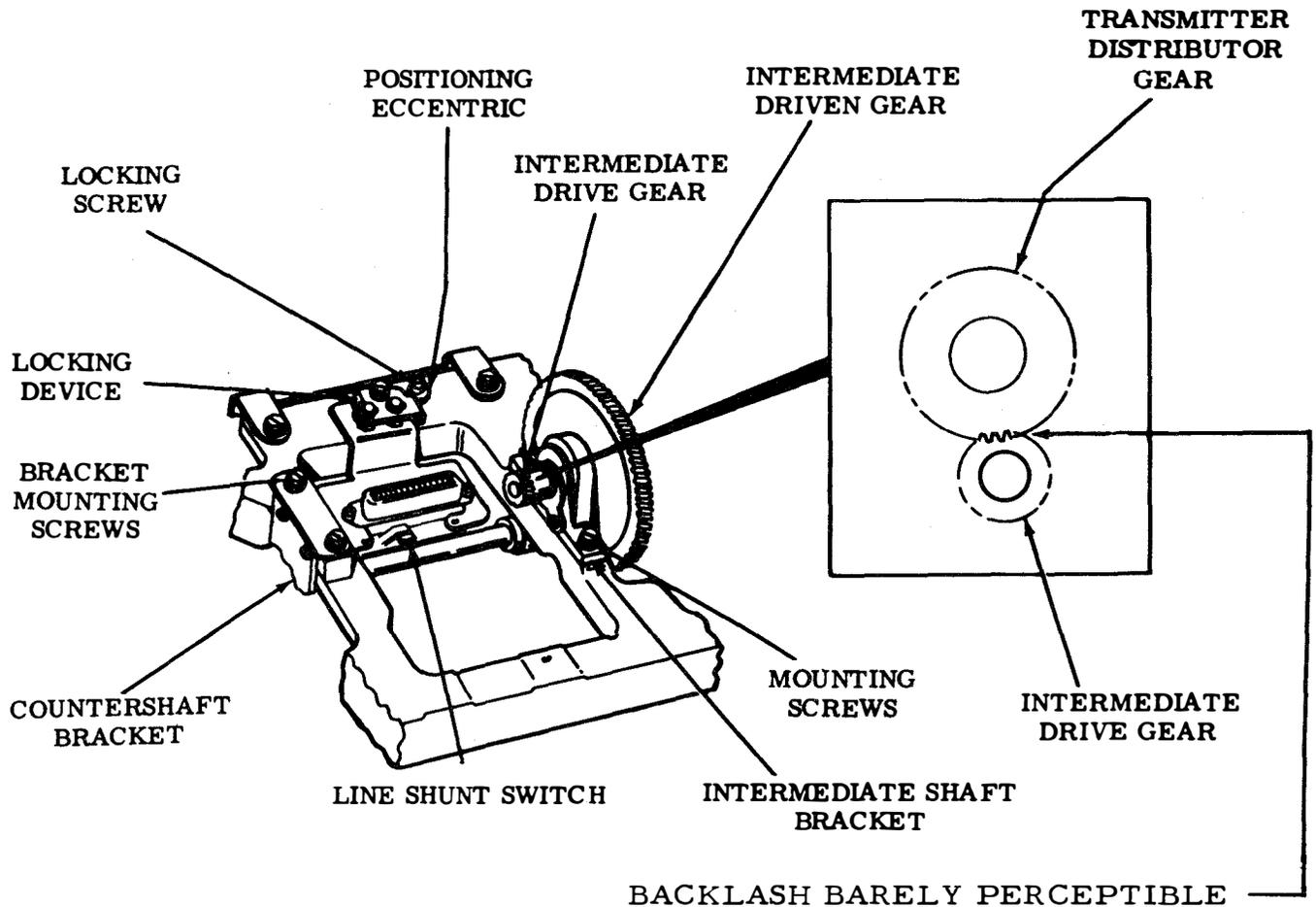
Figure 6-39. Transmitter Distributor Unit Positioning (Variable Speed)
