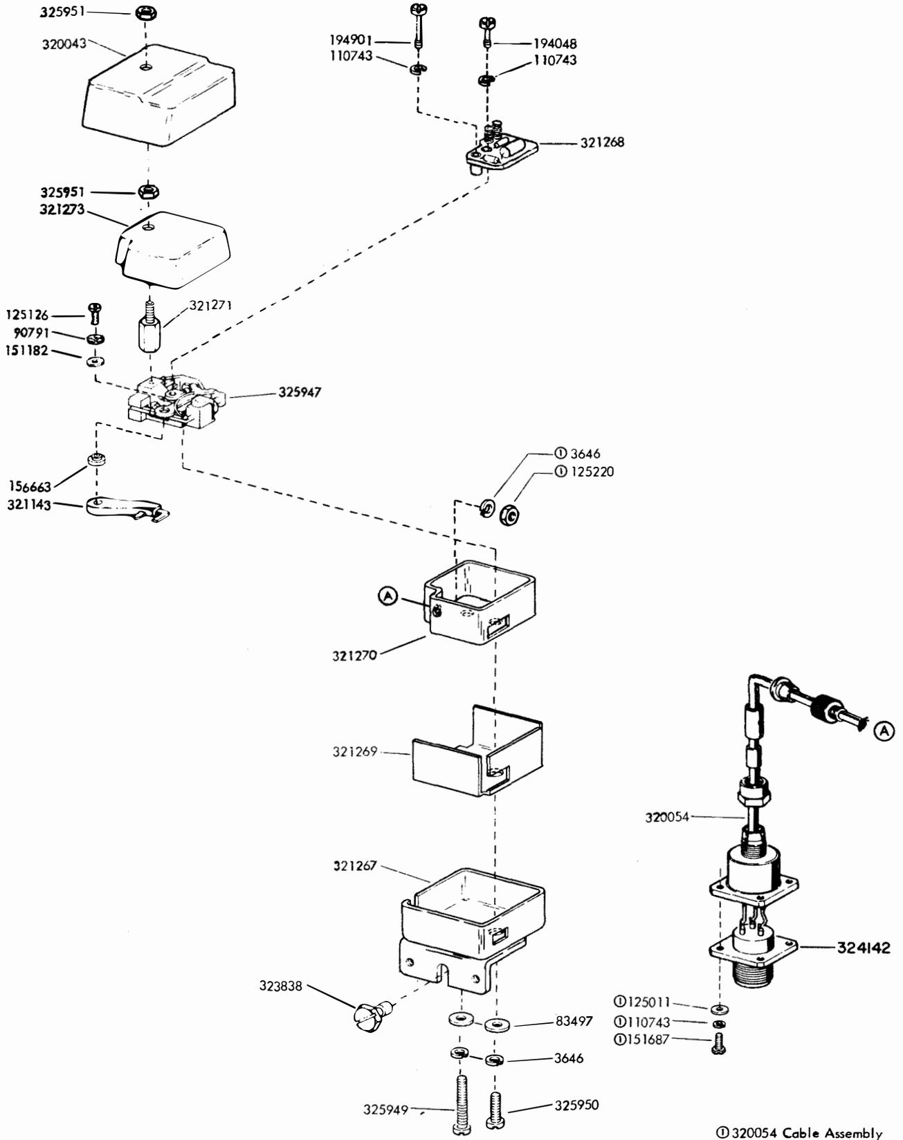
Figure 7-22. Contact Box Assembly 323646 - RFI Suppression Features for Low-Level Sets
