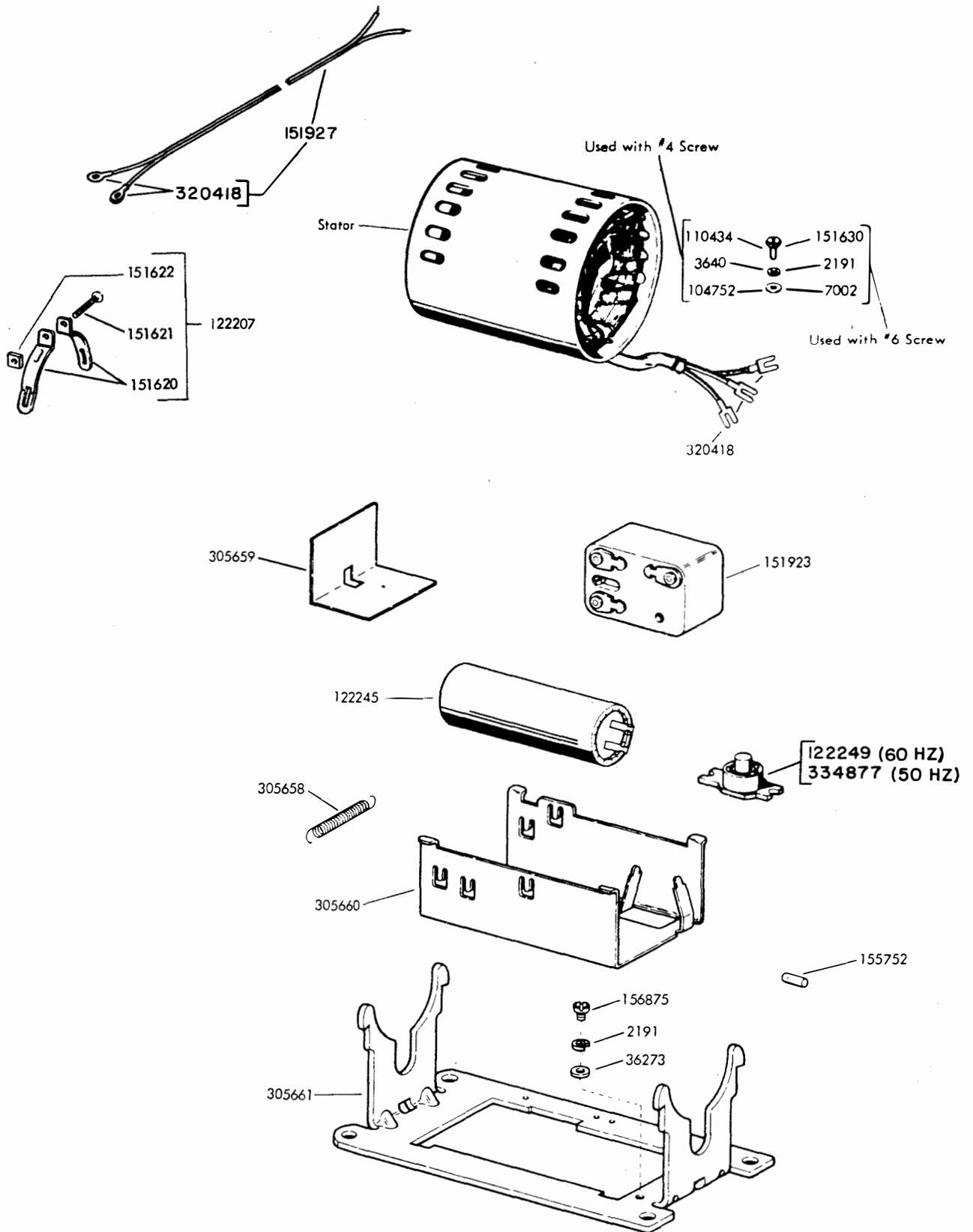
Figure 7-41. Relay and Capacitor Mounting (Synchronous) - Used on LMU3 and LMU38
