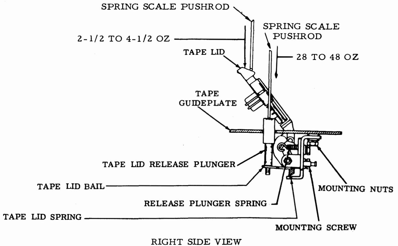
Figure 6-11. Tape Lid Release Plunger Spring and Tape Lid Spring
