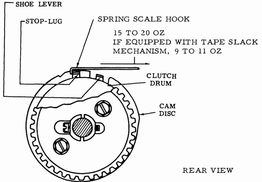
Figure 6-1. Clutch Shoe Lever Spring
