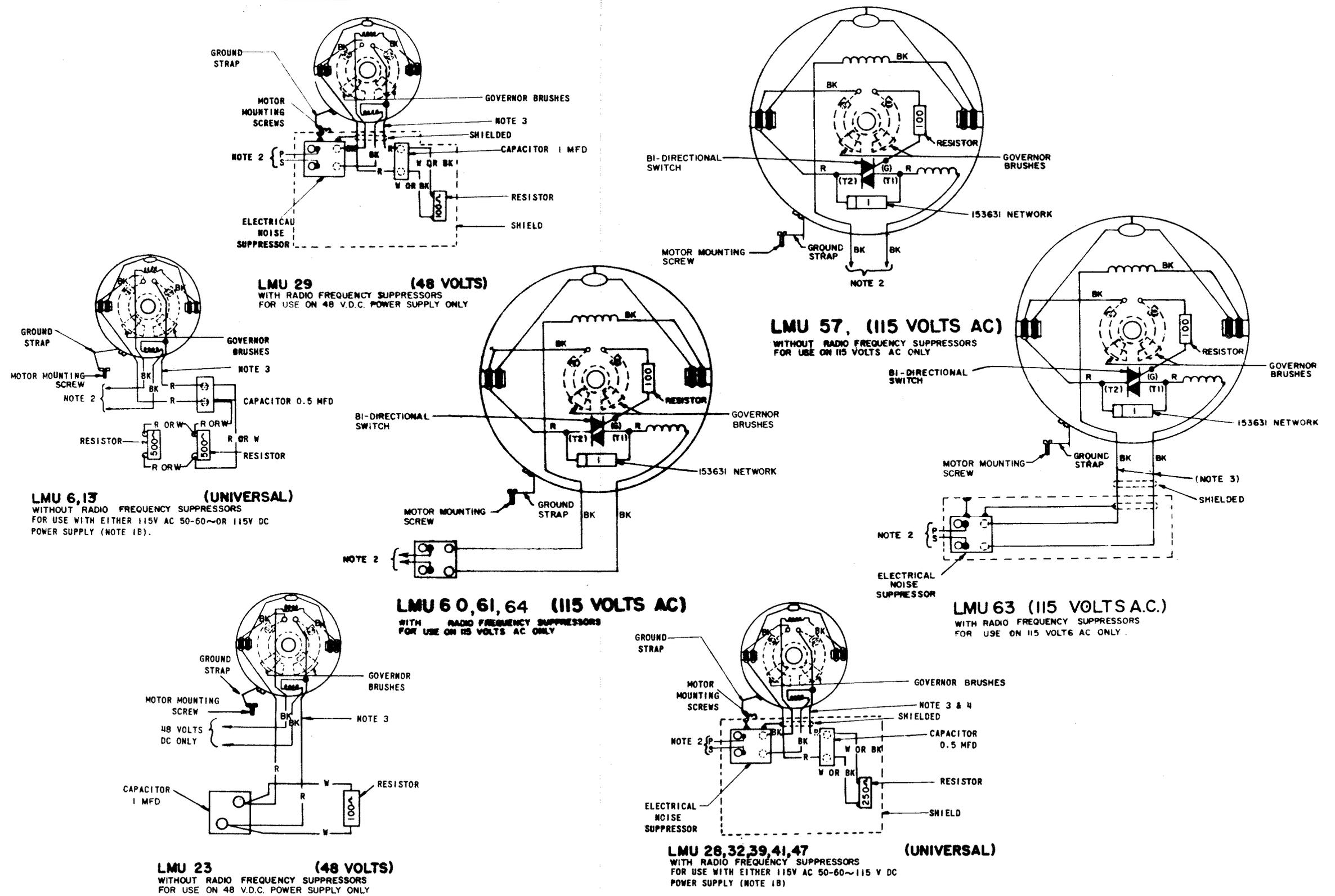
Figure 5-9. Motor Units Wiring Diagram (Sheet 2 of 2)
