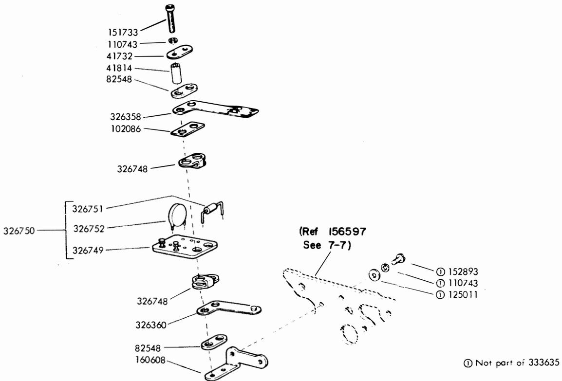
Figure 7-24. Start-Stop Contact Assembly 333635 - RFI Suppression Features for Low-Level Sets
