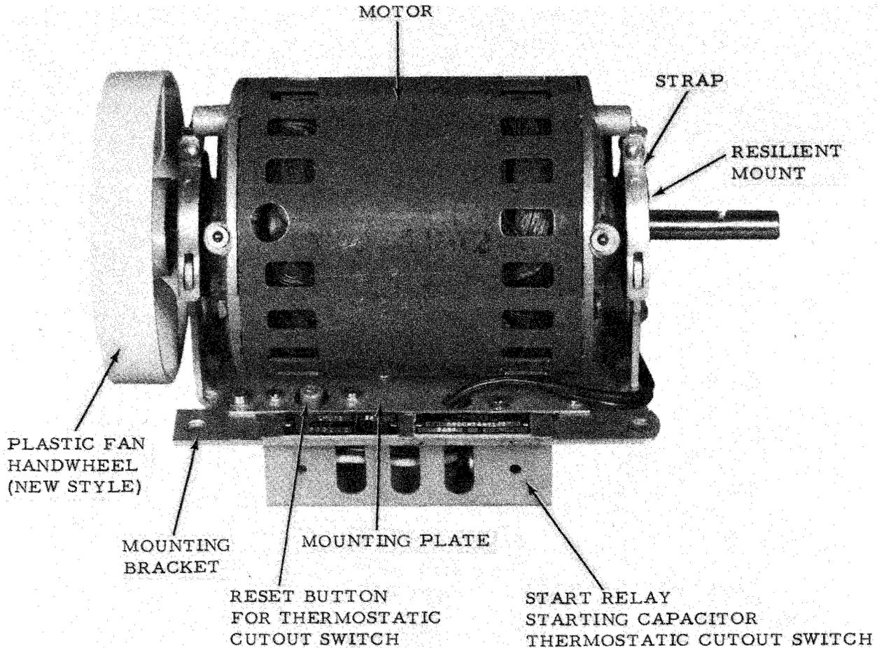
Figure 1-19. Typical Standard or Heavy Duty Synchronous Motor Unit With New-Style Plastic Handwheel
