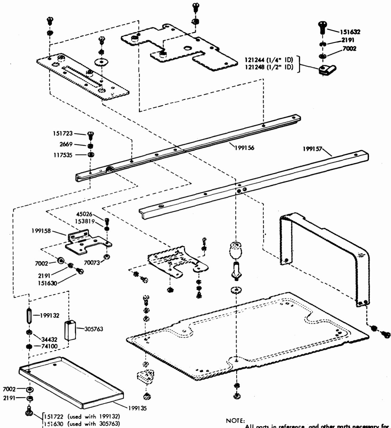
Figure 7-33. Pan, Bracket and Bars to Mount Mechanically Coupled Dual Transmitter Distributor
