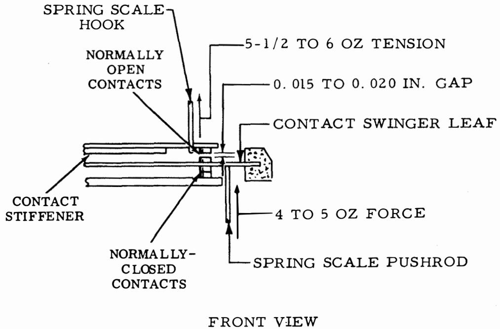
Figure 6-61. Normally-Open Contacts and Normally-Closed Contacts
