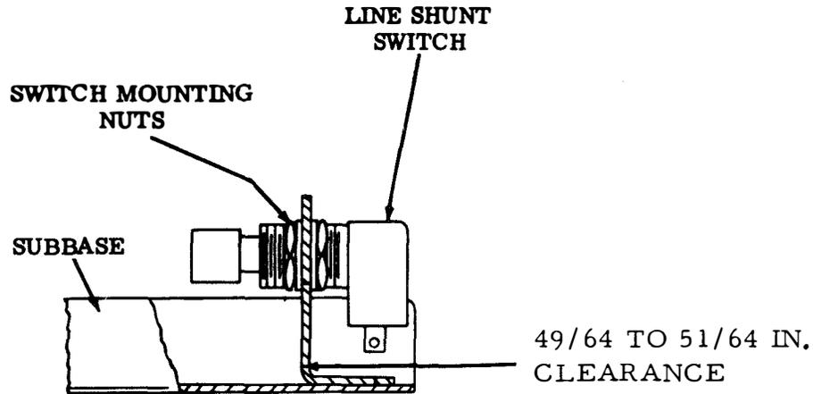
Figure 6-41. Line Shunt Switch TP160370
