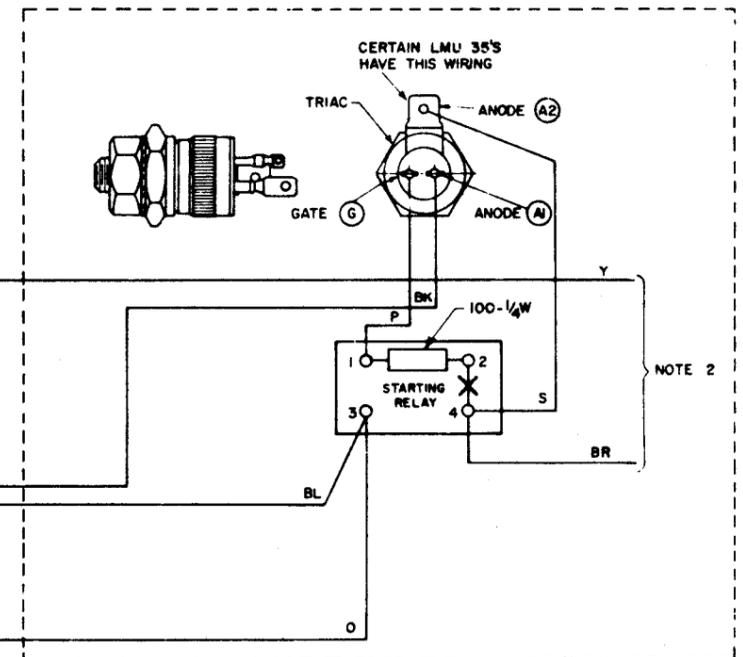
Figure 5-9. Motor Units Wiring Diagram (Sheet 1 of 2)
