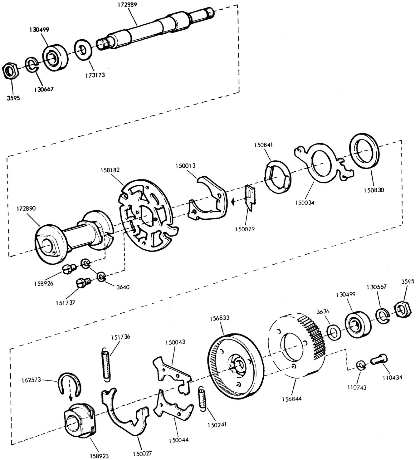
Figure 7-14. Main Shaft Mechanism (Two-Cycle)
