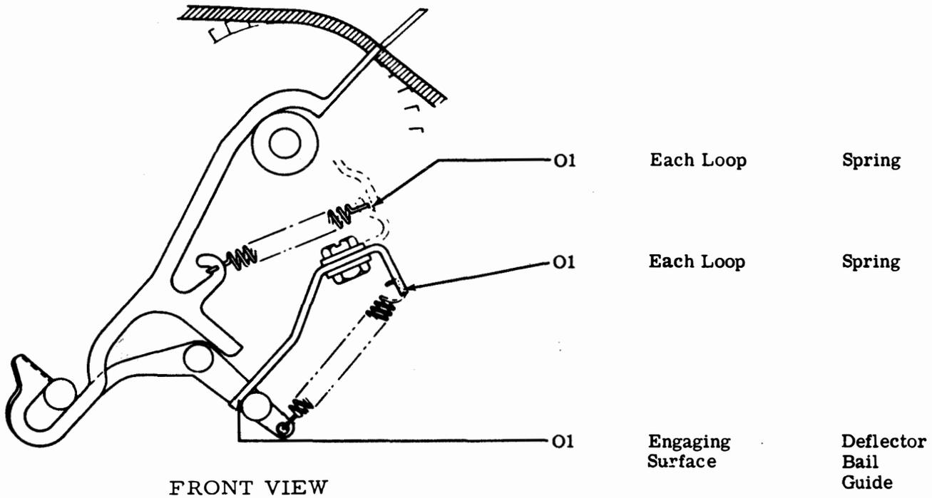
Figure 4-22. Rub-Out Deleter (Variable Features)
