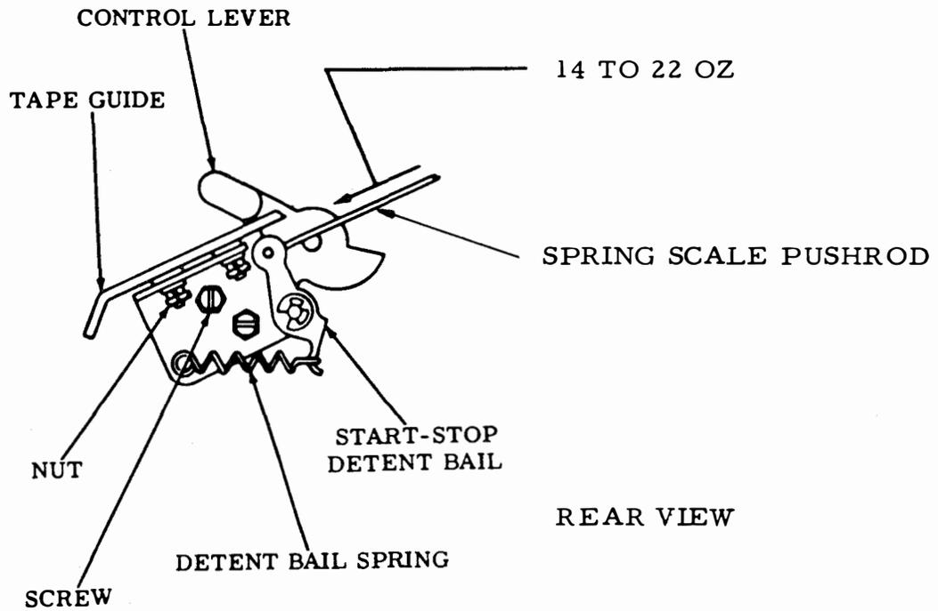
Figure 6-10. Start-Stop Detent Bail Spring
