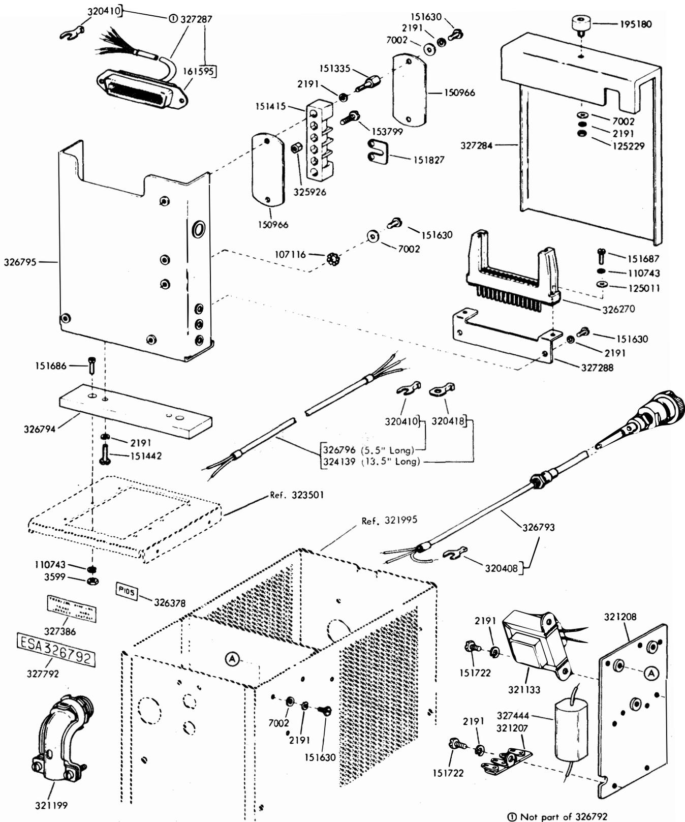
Figure 7-51. Electrical Service Assembly 326792 - Used with Mini TD Set (Sheet 2 of 2)
