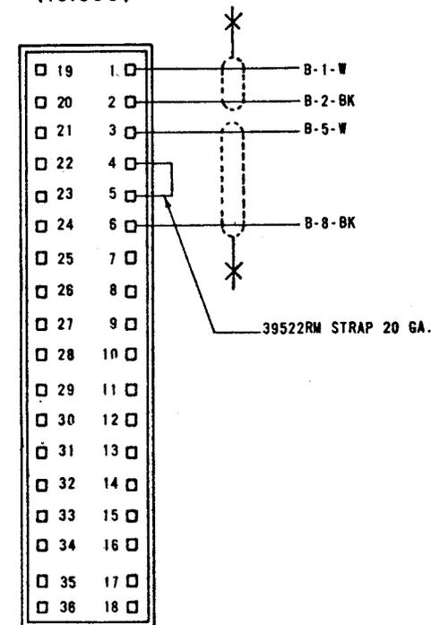
Figure 5-11. Transmitter Distributor Base LXDB20 Wiring Diagram
