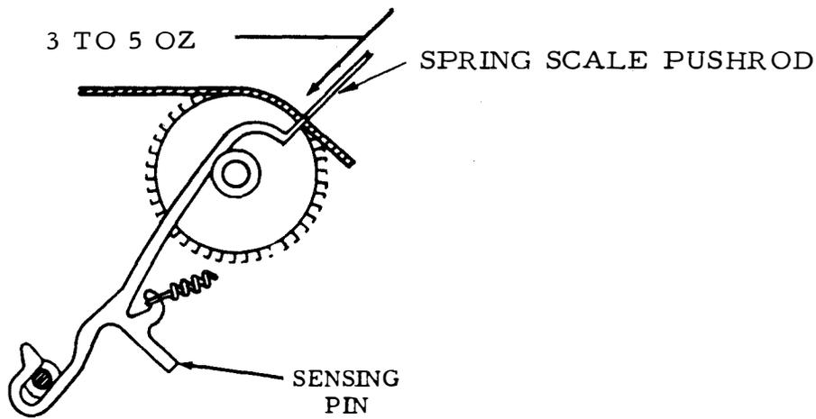
Figure 6-24. Sensing Pin Spring
