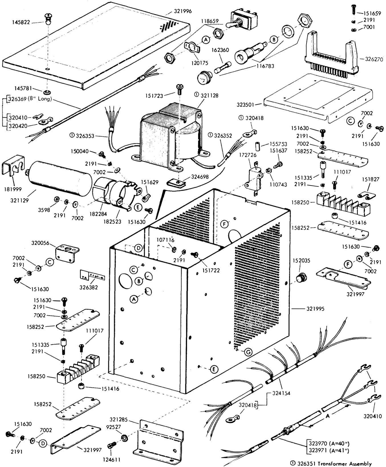
Figure 7-50. Electrical Service Assembly 326792 - Used with Mini TD Set (Sheet 1 of 2)
