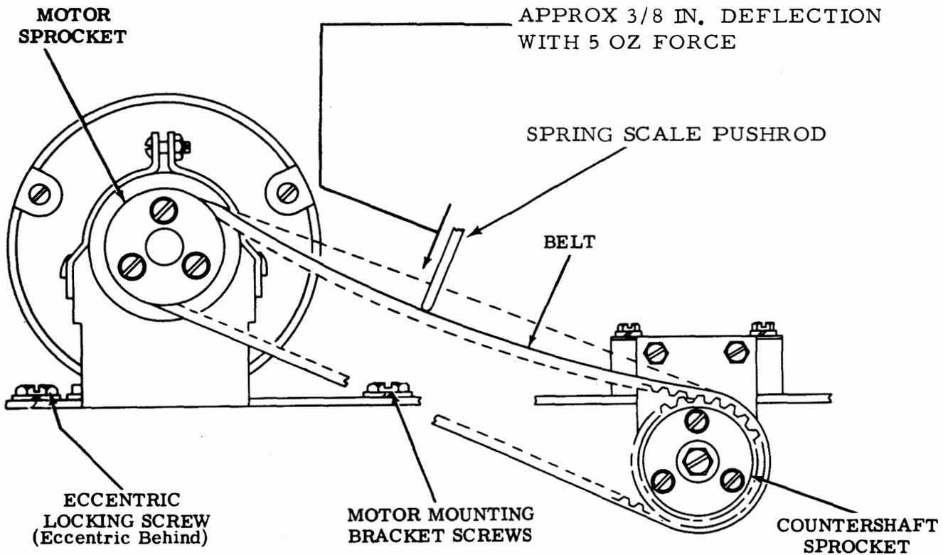
Figure 6-37. Belt Tension (Variable Speed)
