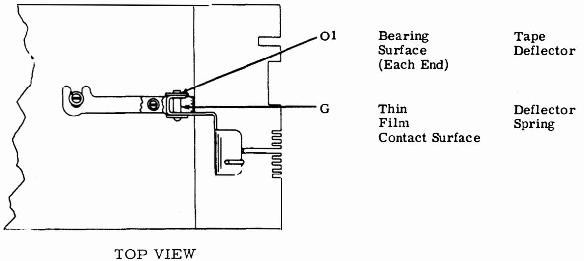
Figure 4-20. Tape Deflector (Variable Features)
