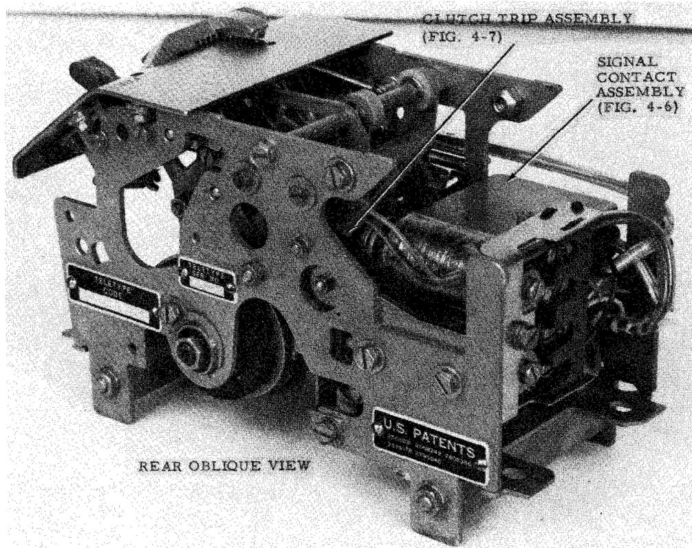
Figure 4-4. Transmitter Distributor
