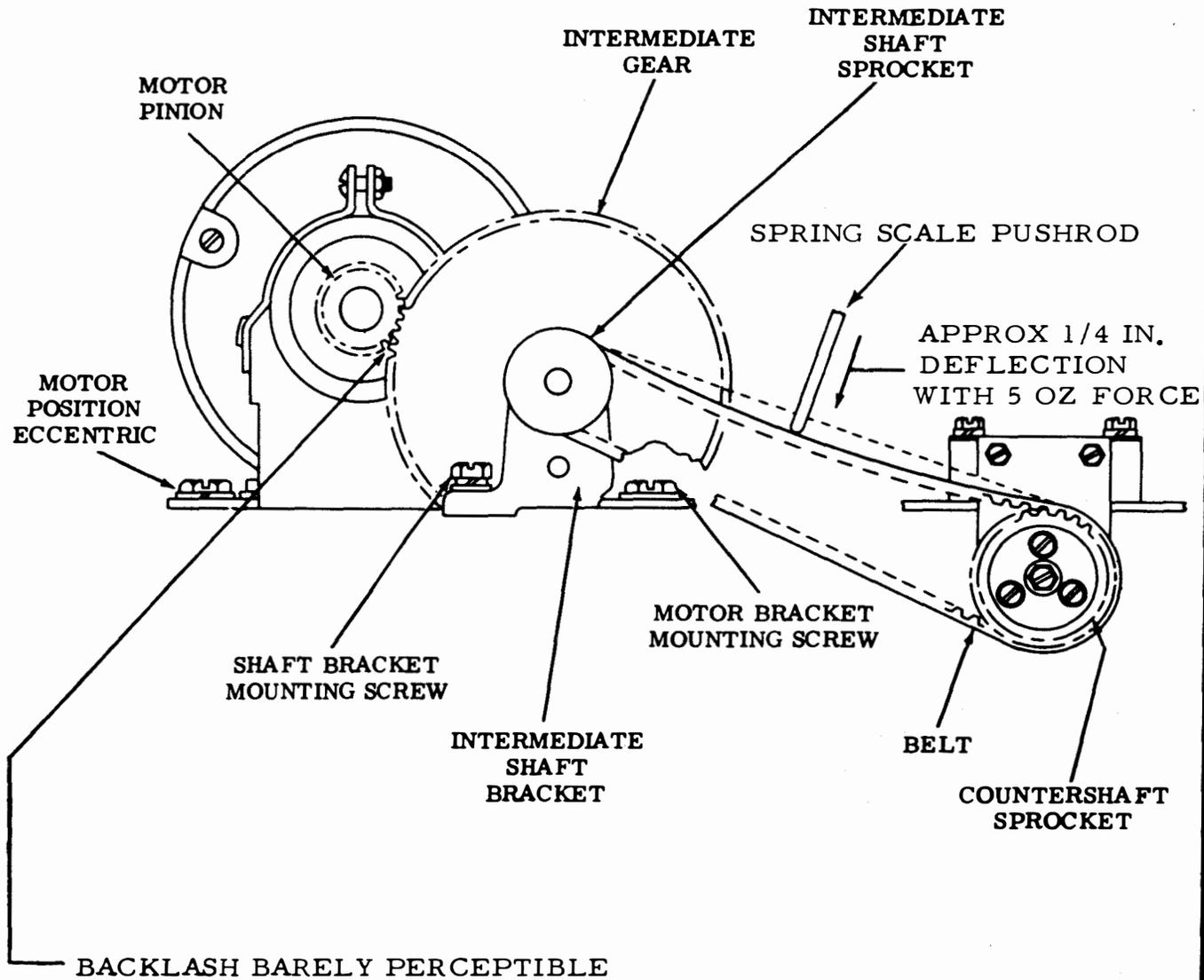
Figure 6-35. Belt Tension (Common Speed) and Motor Pinion - Intermediate Gear Backlash
