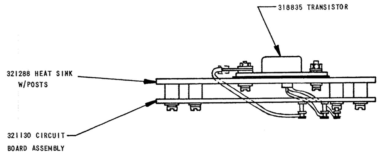
Figure 5-16. Power Supply 321290 (0.5 Ampere) Schematic Diagram (Sheet 1 of 2)
