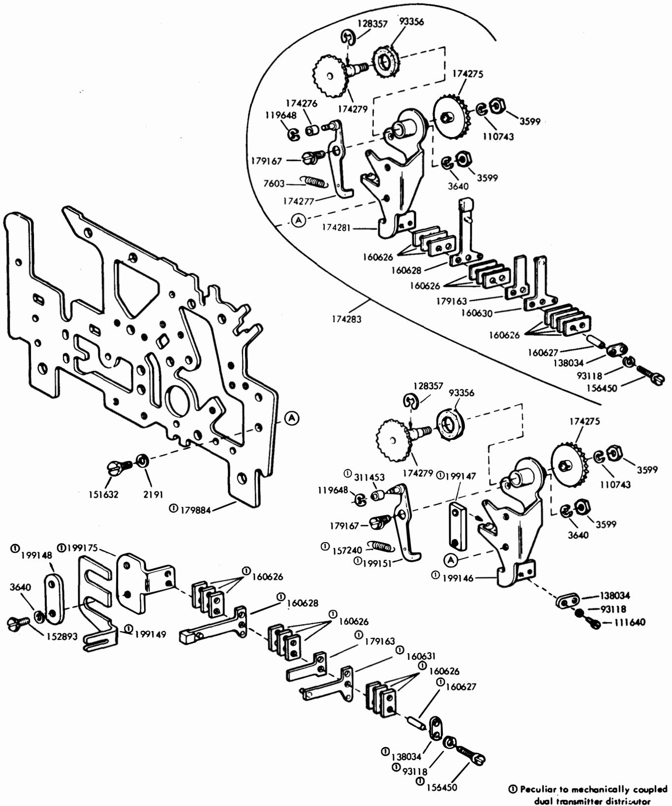
Figure 7-5. Front Plate Mechanism (With Tape Feed Assurance Contact)
