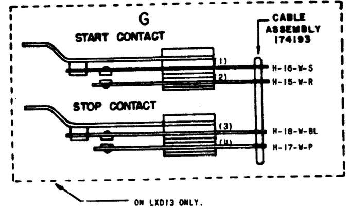
Figure 5-2. Transmitter Distributor Unit LXD4, 9, 13, 15, 18, 19, 20, 26, 601, 602, 800, 802, 30, 41 Wiring Diagram
