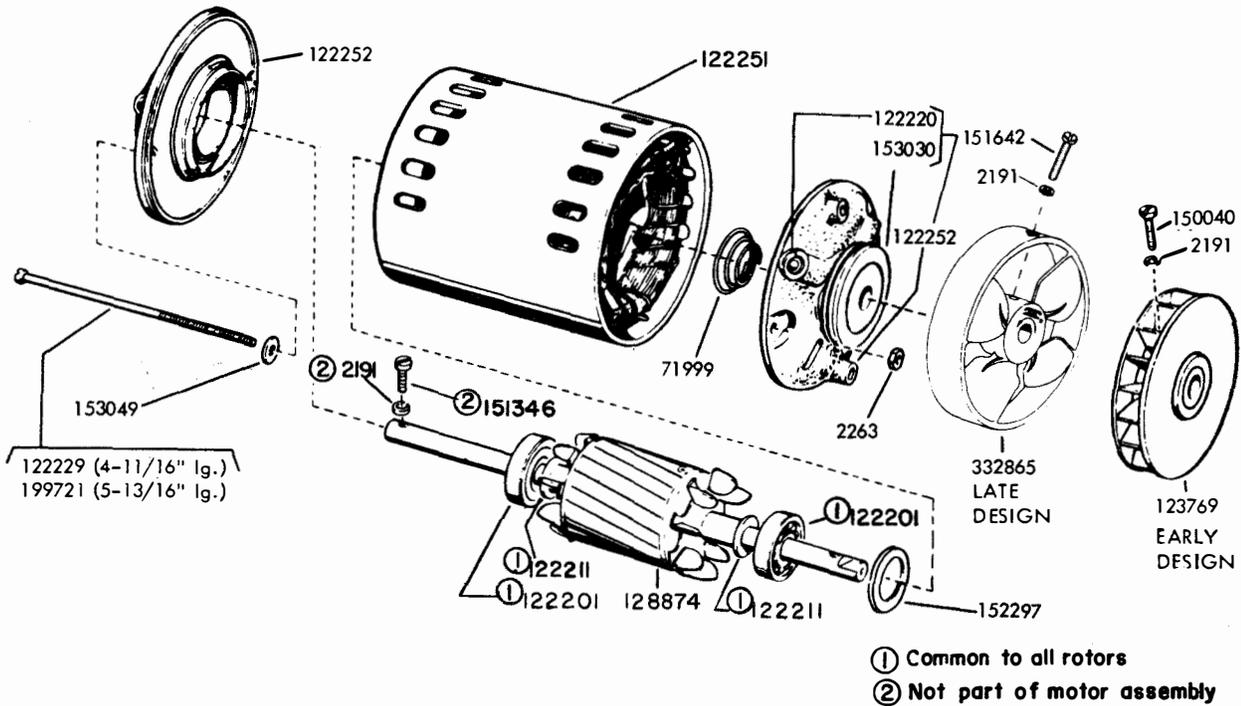
Figure 7-40. Synchronous Motor Assembly 161985 (Miniature) - Used on LMU19
