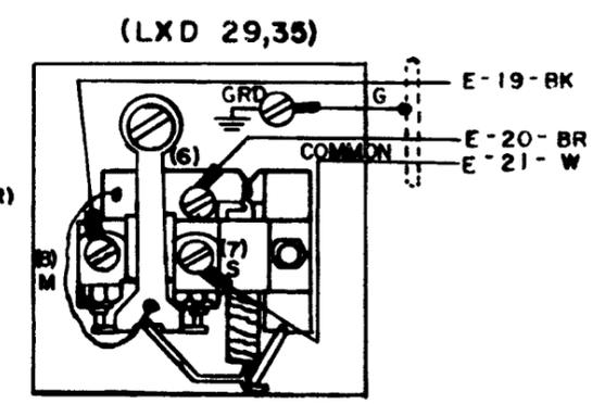
Figure 5-3. Transmitter Distributor Unit LXD11, 29, 35 Wiring Diagram
