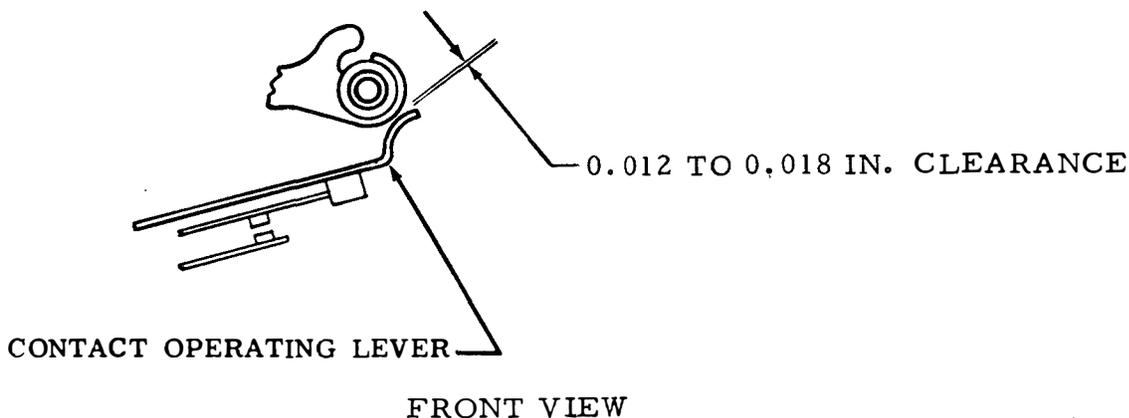
Figure 6-66. Contact Bracket
