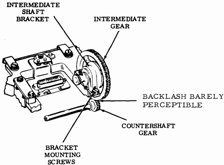
Figure 6-38. Intermediate Gear - Countershaft Gear Backlash
