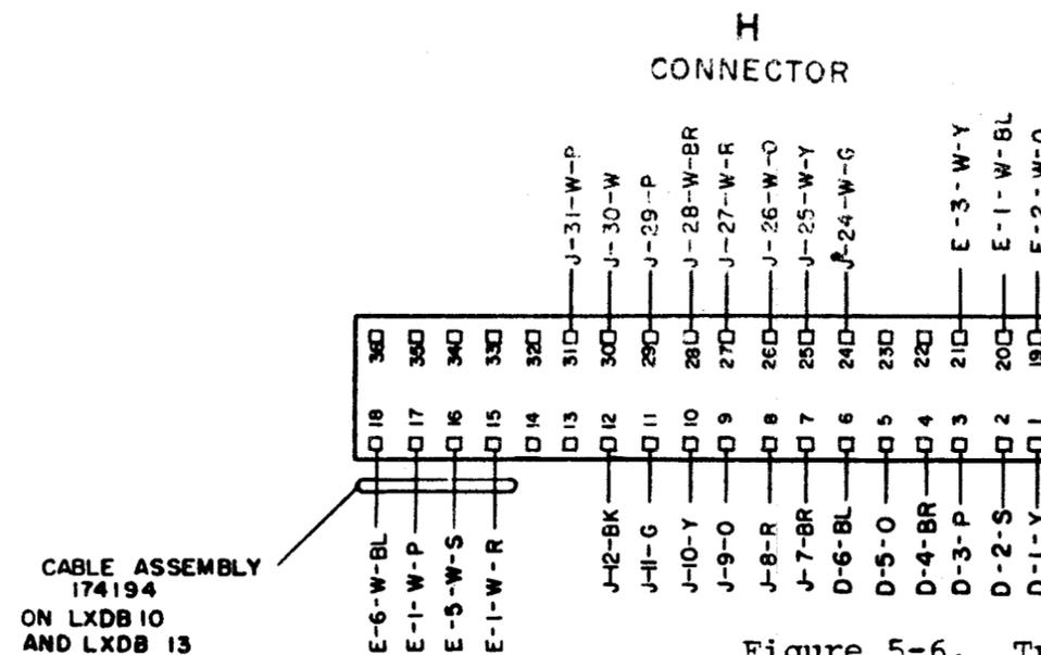
Figure 5-6. Transmitter Distributor Base LXDB3, 4, 5, 10, 13, 15 Wiring Diagram
