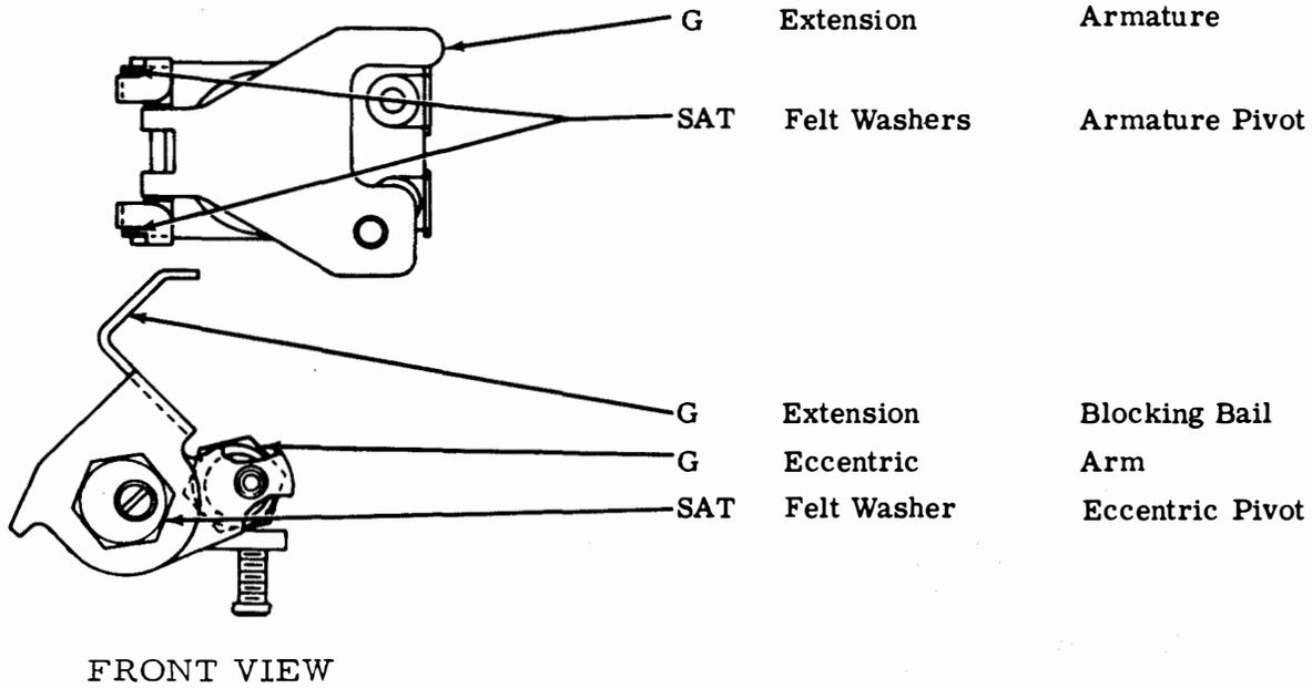
Figure 4-24. Tape-Withhold Mechanism (Variable Features)
