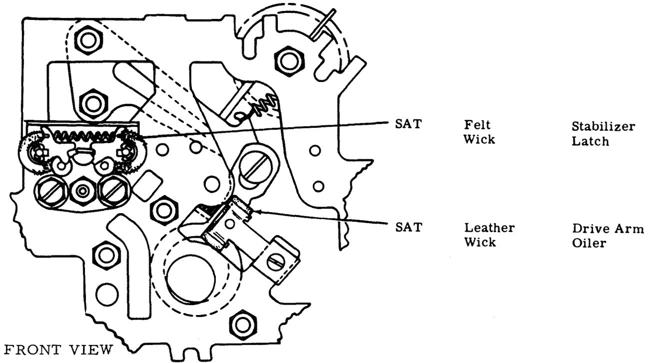
Figure 4-13. Front Plate Assembly
