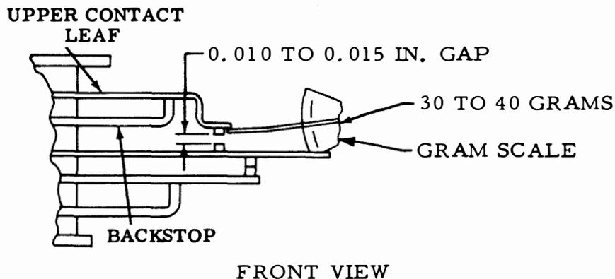
Figure 6-56. Normally-Open Contacts - Gap and Normally-Open Contacts - Spring
