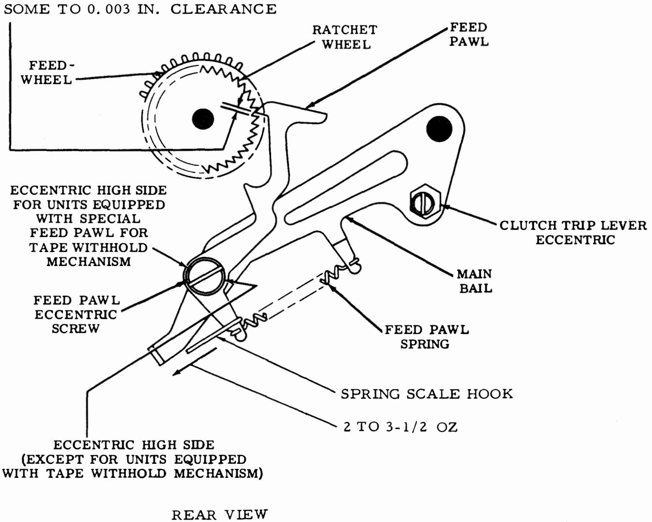
Figure 6-26. Feed Pawl and Feed Pawl Spring
