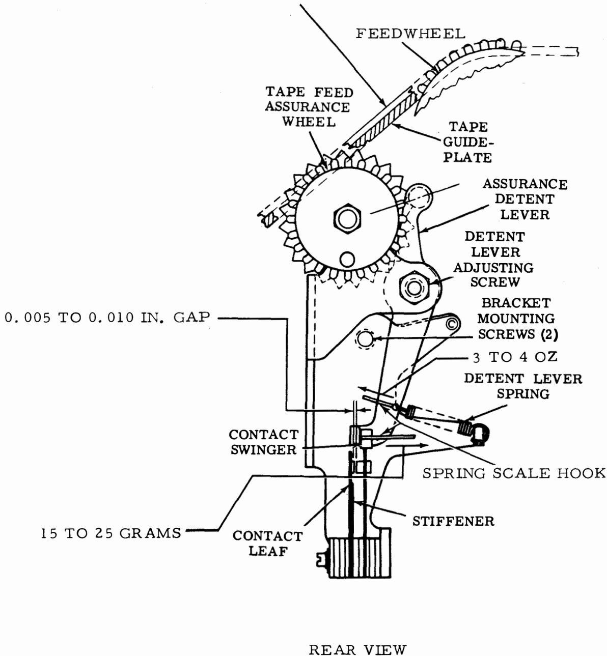
Figure 6-51. Tape Sensing Feedwheel Phasing, Tape Motion Contact Gap, Tape Motion Contact Swinger, and Detent Lever Spring
