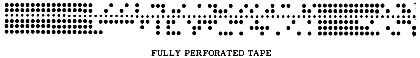
Figure 3-3. Standard 5-Level Perforated Tapes
