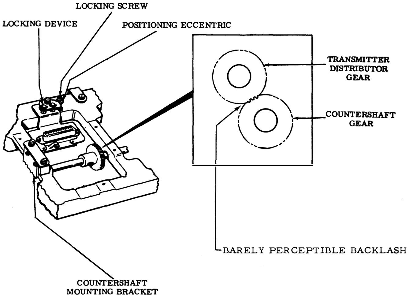
Figure 6-36. Transmitter Distributor Unit Positioning (Common Speed)
