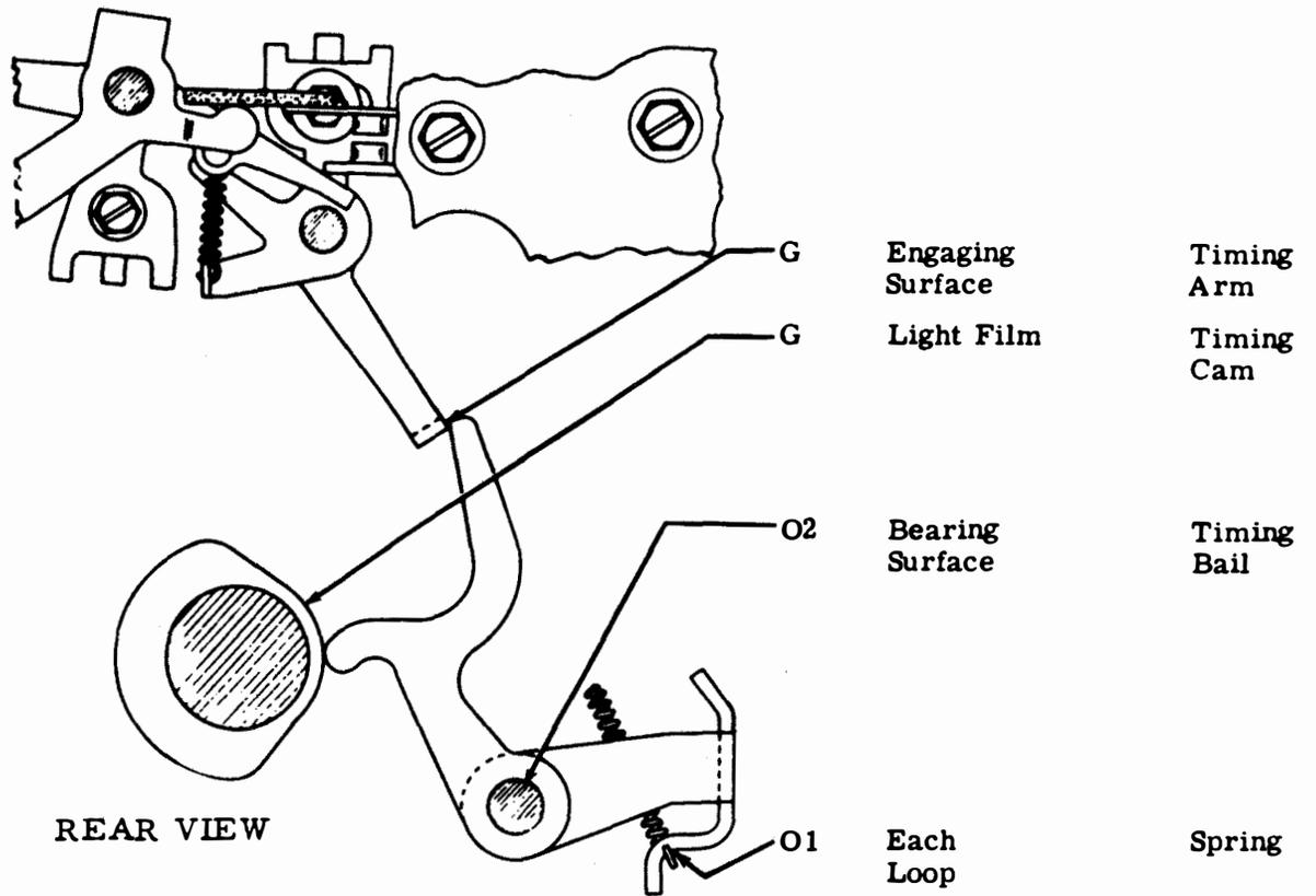
Figure 4-23. Transmitter Stop Mechanism (Variable Features)
