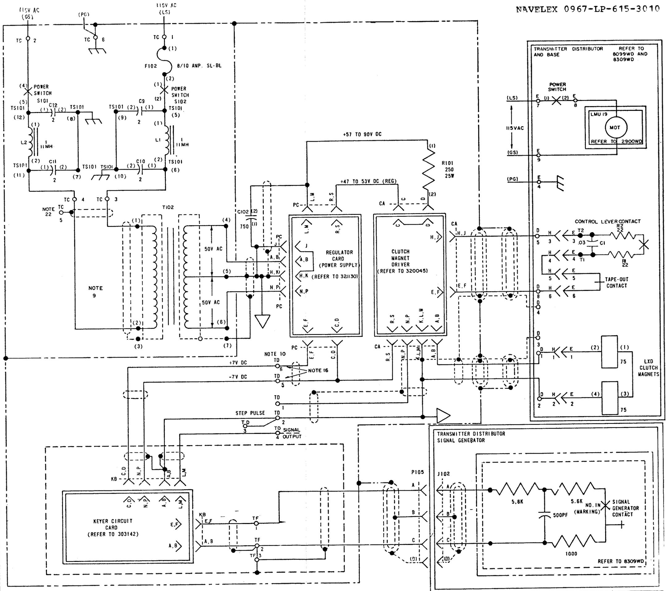
Figure 5-12. Electrical Service Assembly 326792 Schematic Diagram
