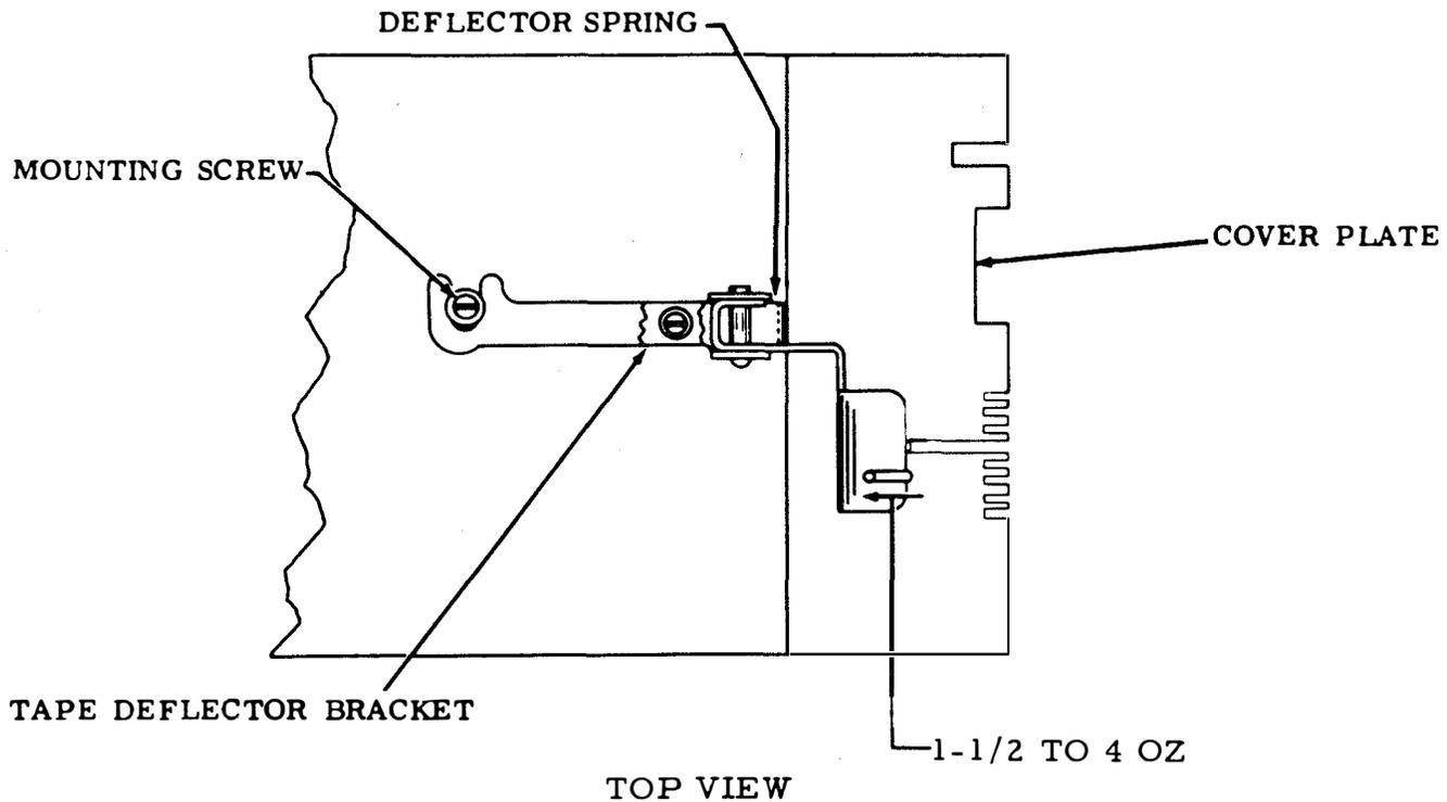
Figure 6-64. Tape Deflector Bracket and Tape Deflector Spring
