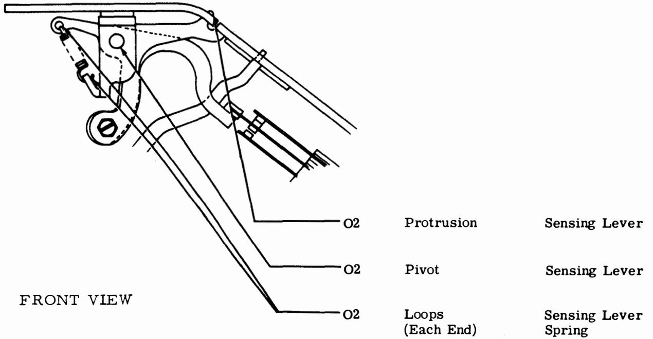
Figure 4-19. Tape Lid Sensing Lever (Variable Features)
