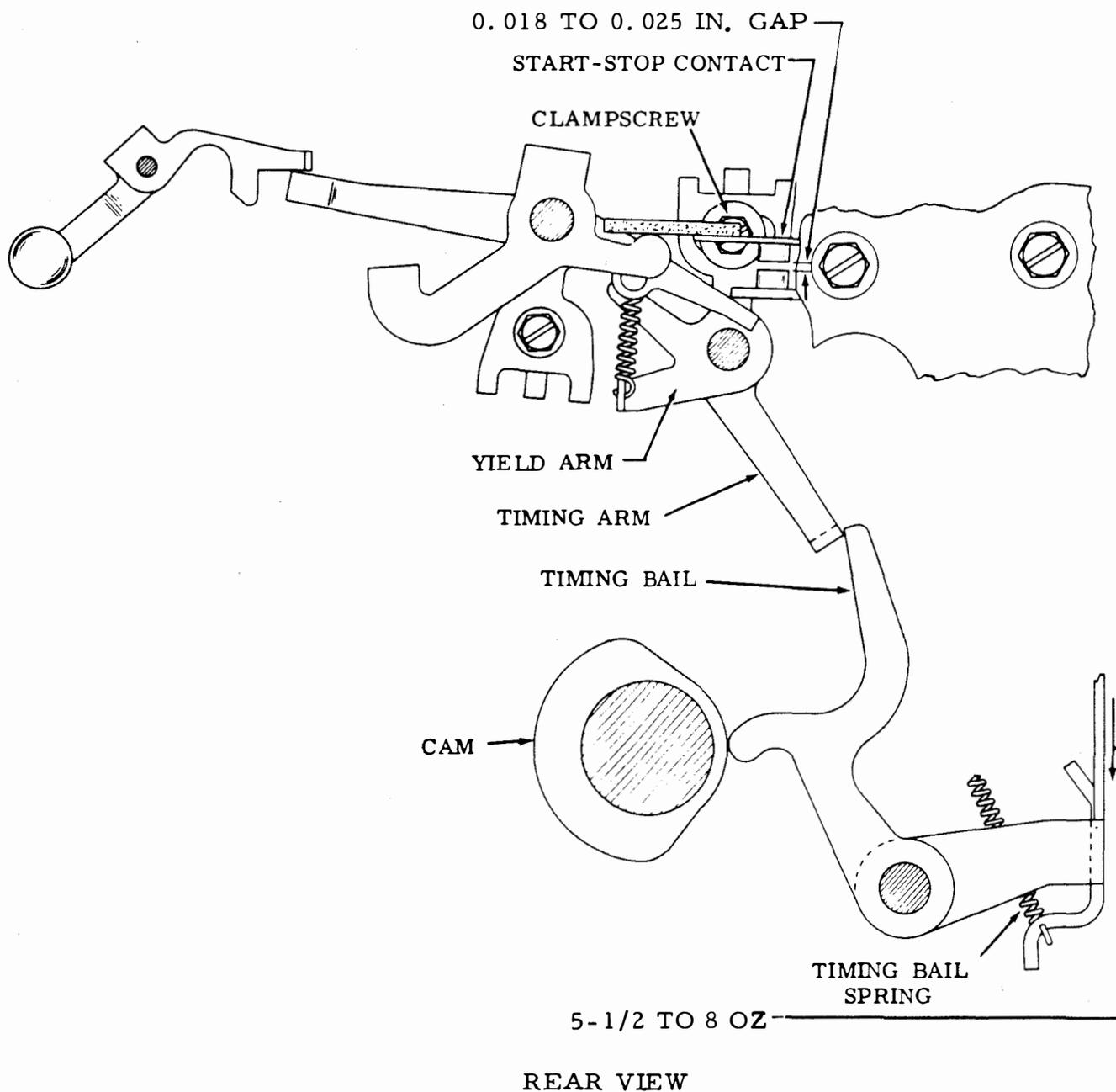
Figure 6-70. Start-Stop Gap (For Tabulator Control) and Timing Bail Spring
