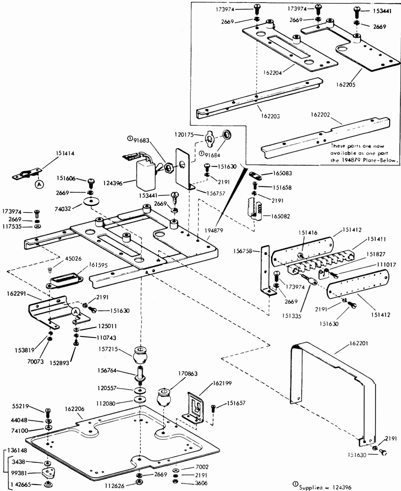
Figure 7-26. Miniature Base and Electrical Components (Sheet 1 of 2)
