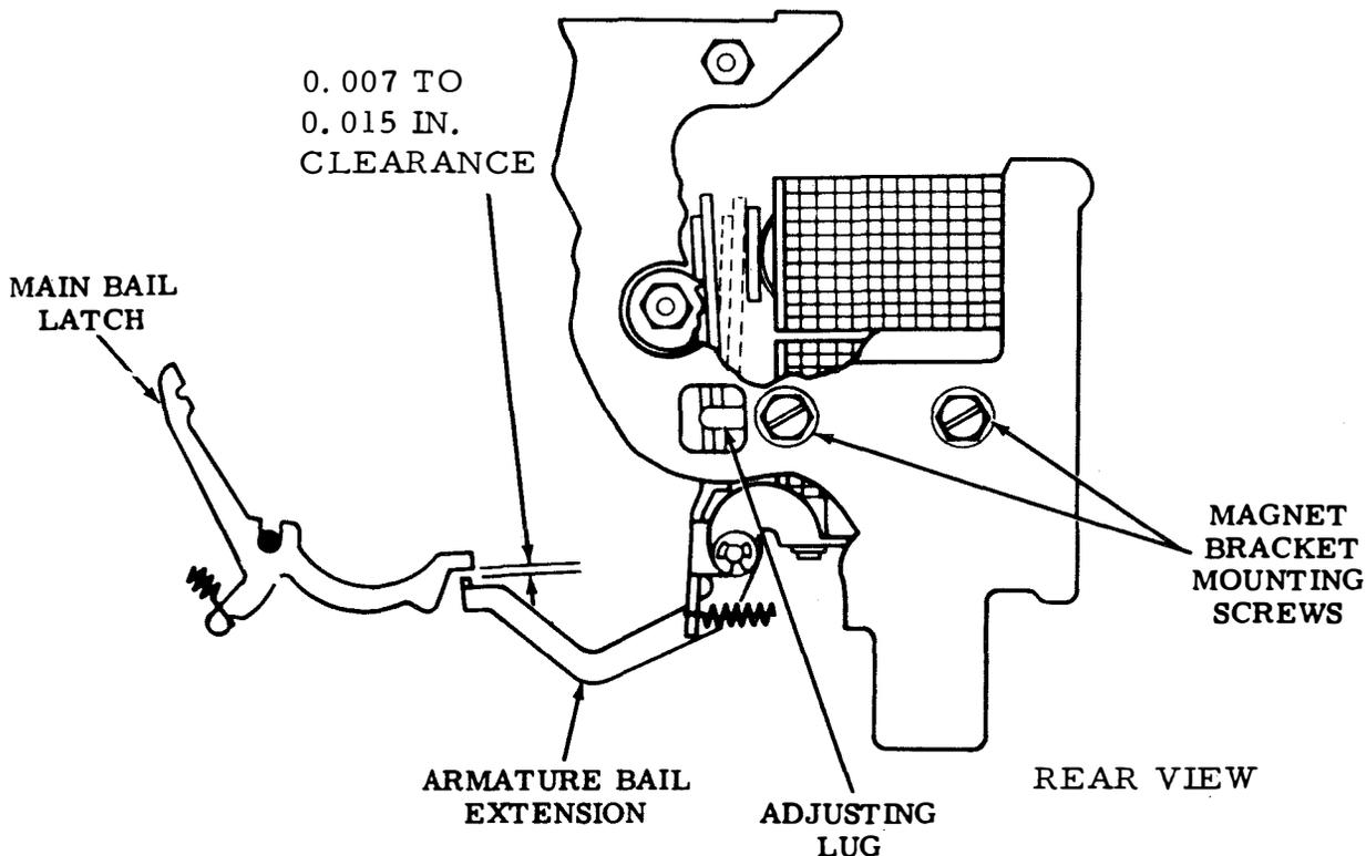
Figure 6-6. Clutch Magnet Assembly (Preliminary) (Main Bail Clearance)
