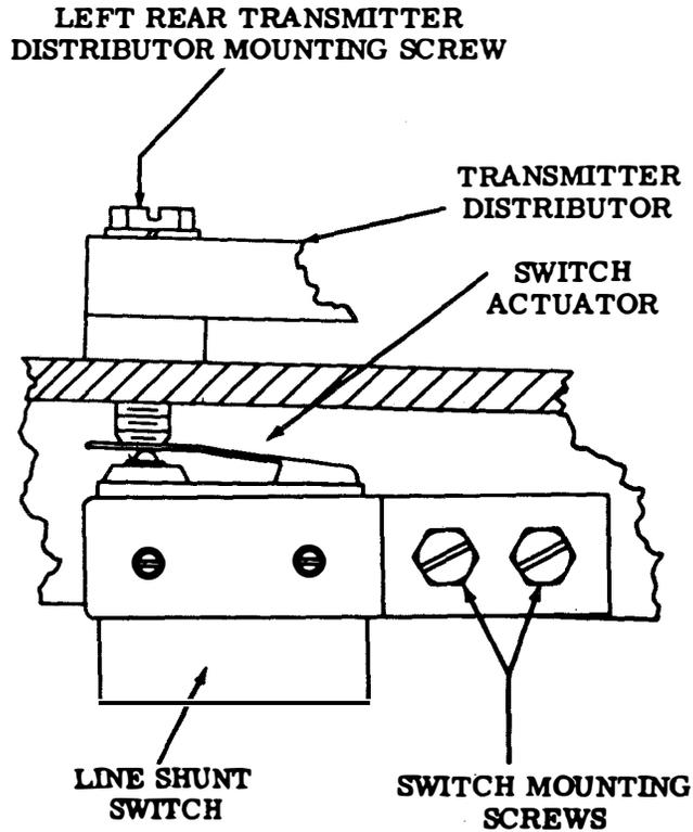
Figure 6-42. Line Shunt Switch TP172847
