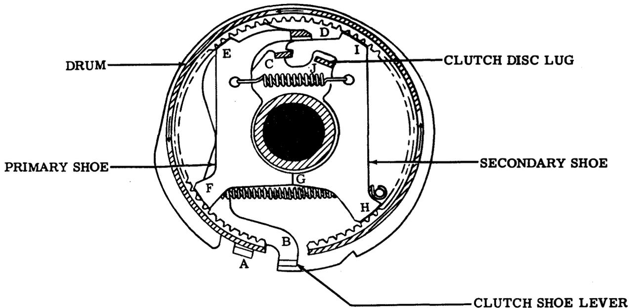
Figure 3-17. Clutch Engaged
