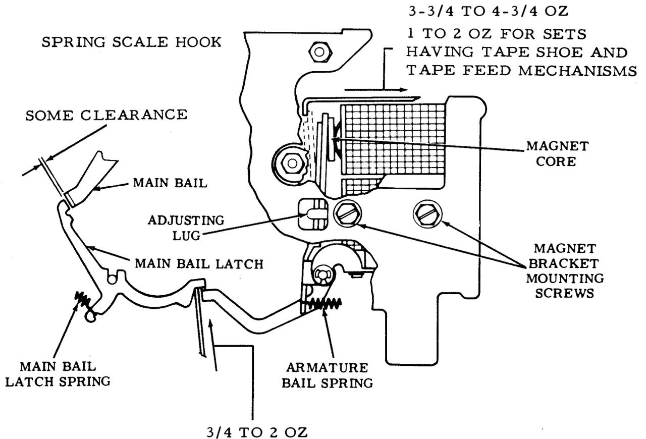
Figure 6-7. Clutch Magnet Assembly (Preliminary) (Latchlever Clearance)
