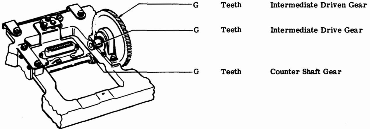
Figure 4-33. Intermediate Gears - Single Contact Multiple Mounting Bases (Variable Speed)
