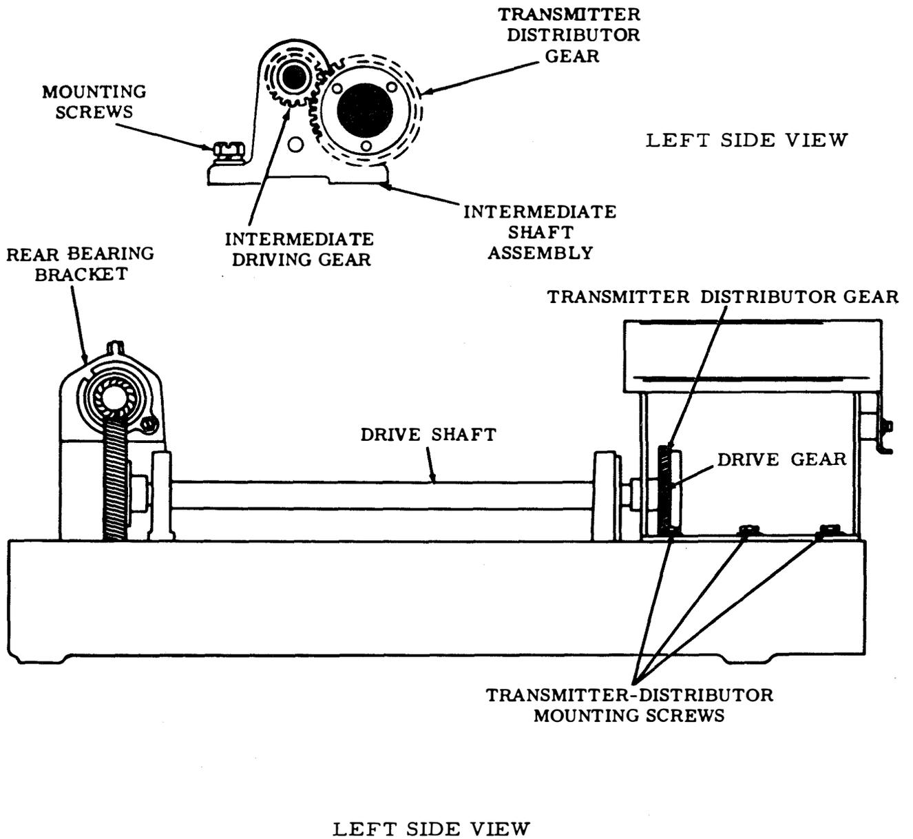
Figure 6-32. Intermediate Gear - Transmitter Distributor Gear Backlash
