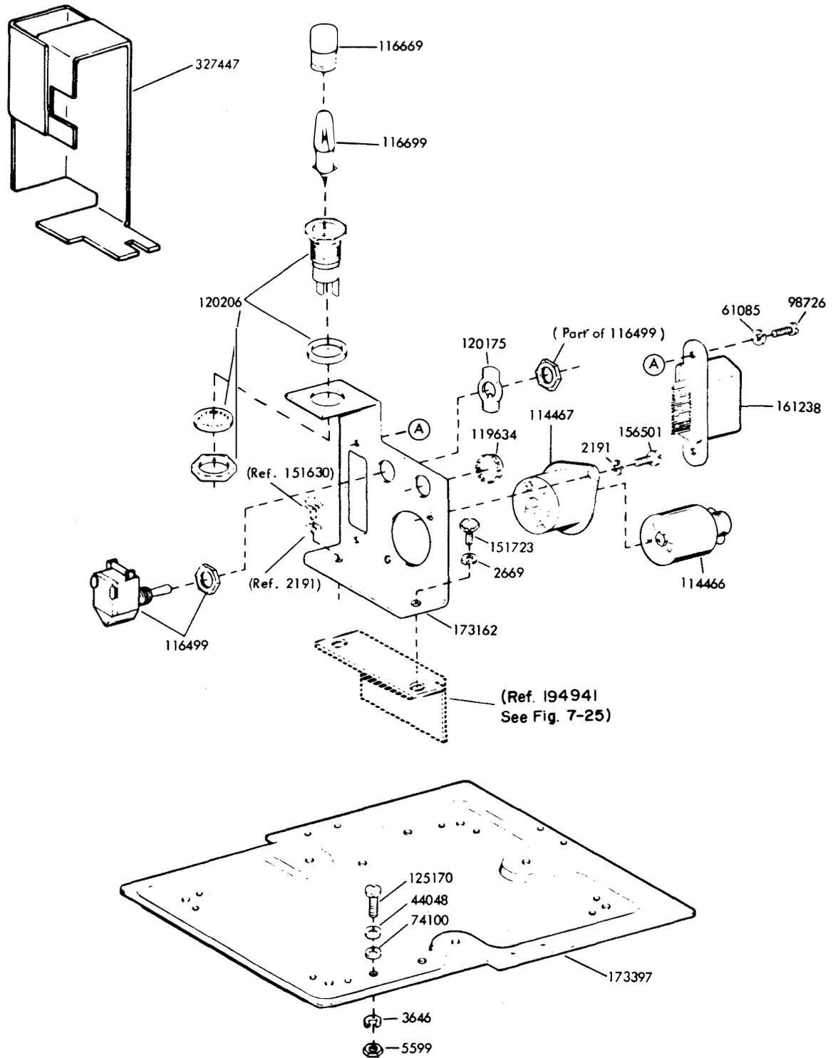
Figure 7-27. Miniature Base and Electrical Components
