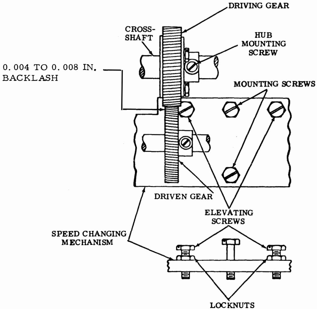
Figure 6-46. Speed Change Gear
