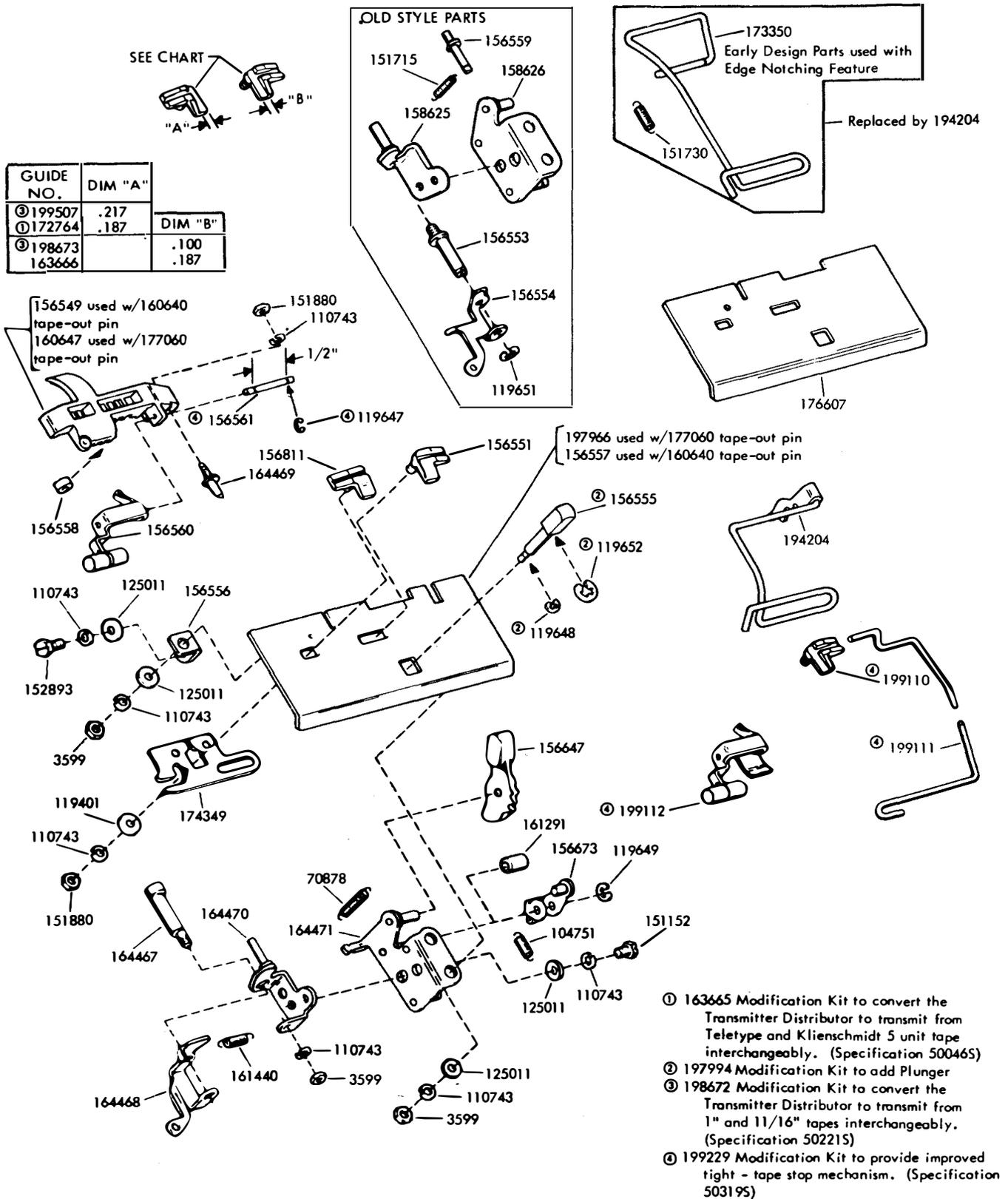
Figure 7-15. Tape Guide Plate Mechanisms (Sheet 1 of 3)
