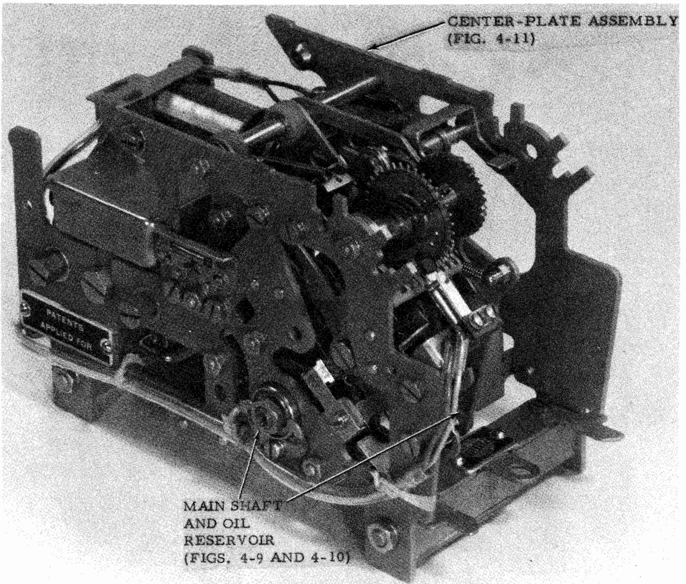
Figure 4-8. Main Shaft, Oil Reservoir, and Center Plate Assembly
