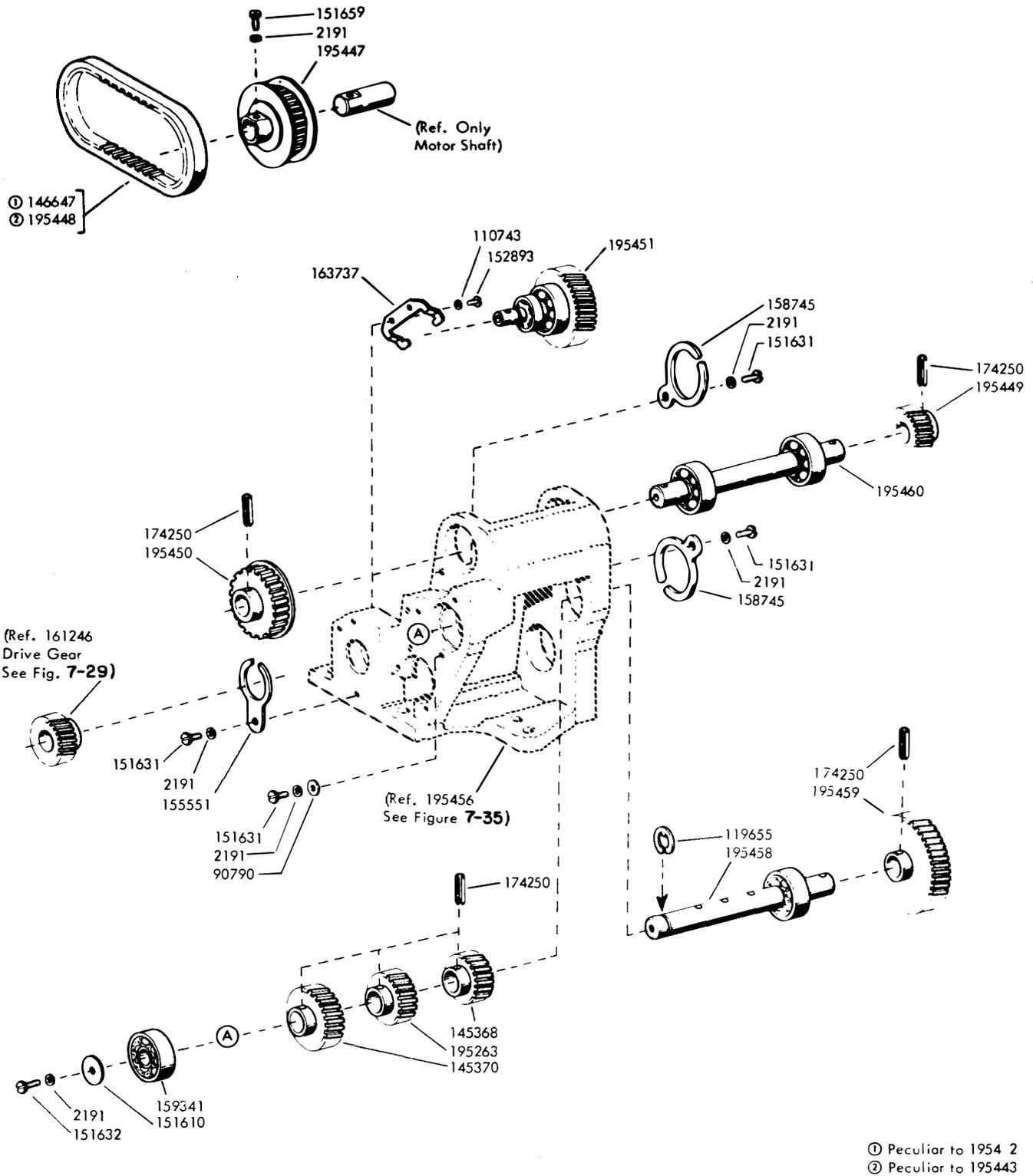
Figure 7-36. Modification Kits 195442 and 195443 to Add Three-Speed Gearshift Assemblies (Sheet 3 of 3)
