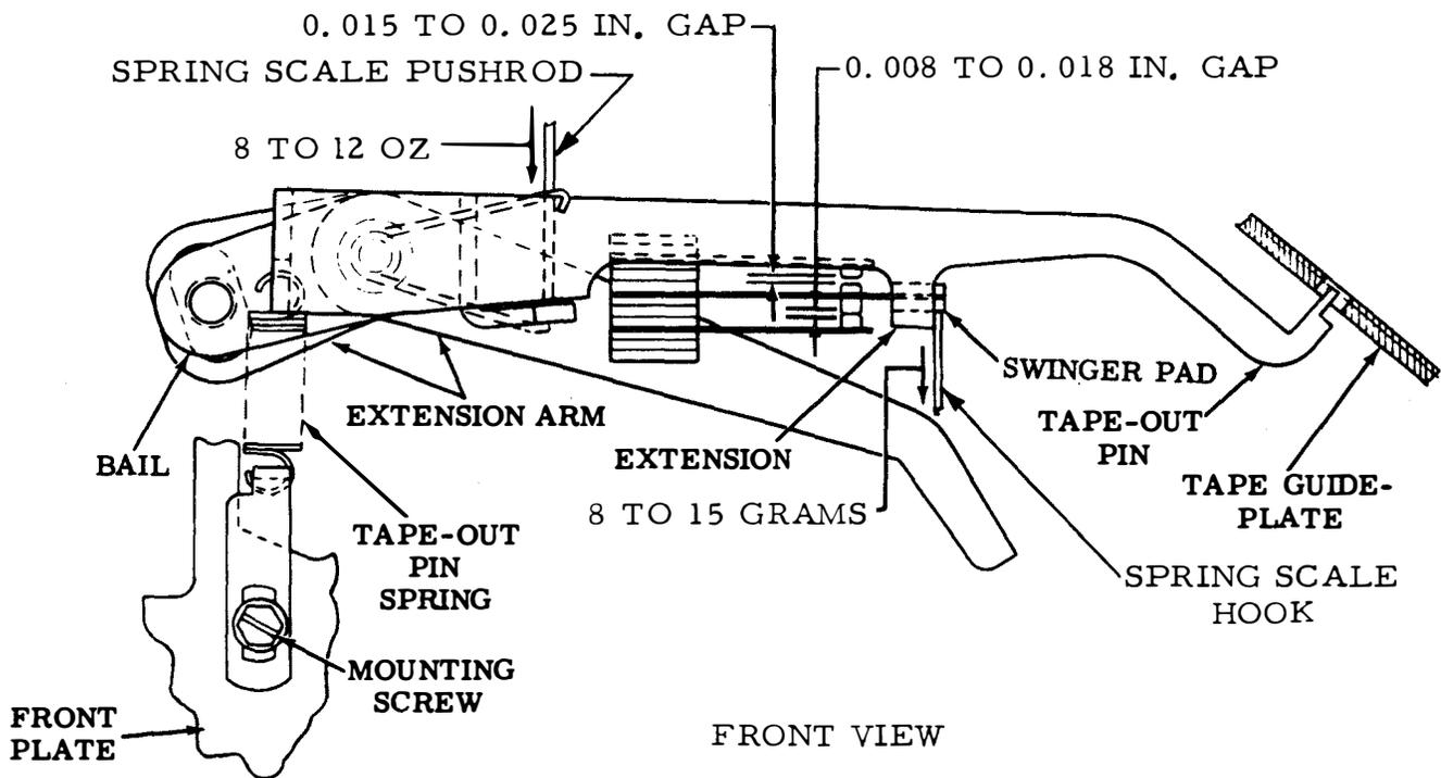
Figure 6-52. Tape-Out Contact and Tape-Out Bail Torsion Spring
