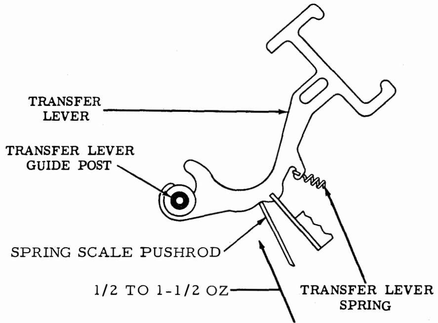
Figure 6-27. Transfer Lever Spring
