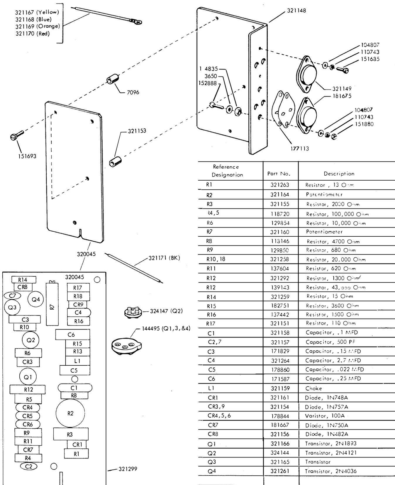
Figure 7-53. Clutch Magnet Driver Circuit Card 321991
