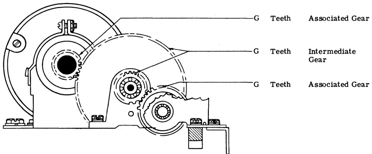
Figure 4-27. Intermediate Gear - Single Contact Single Mounting Bases
