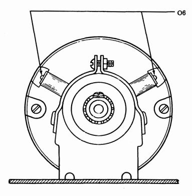
One Oiler at Each End (Depress Oiler With Metal Object) Motor Bearings
