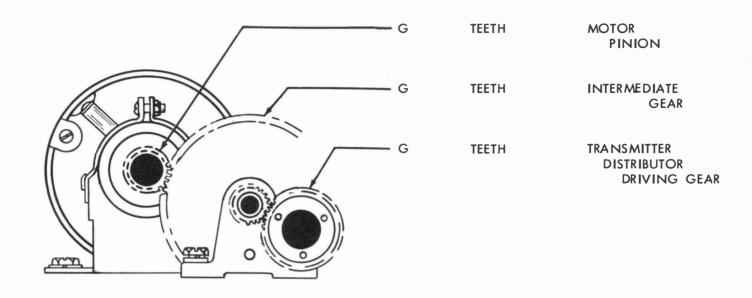
2.05 Intermediate Gear Assembly (Multicontact Self-contained Transmitter-Distributor Set)
