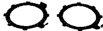
Figure 17.,,Showing the rear ring needed on the spacing drum for auto CR-LF. The new 154626 is on the left, the old 154625 on the right. Note the new one has an extra tab, which engages the bellcrank to move the "Zero" code bar.
