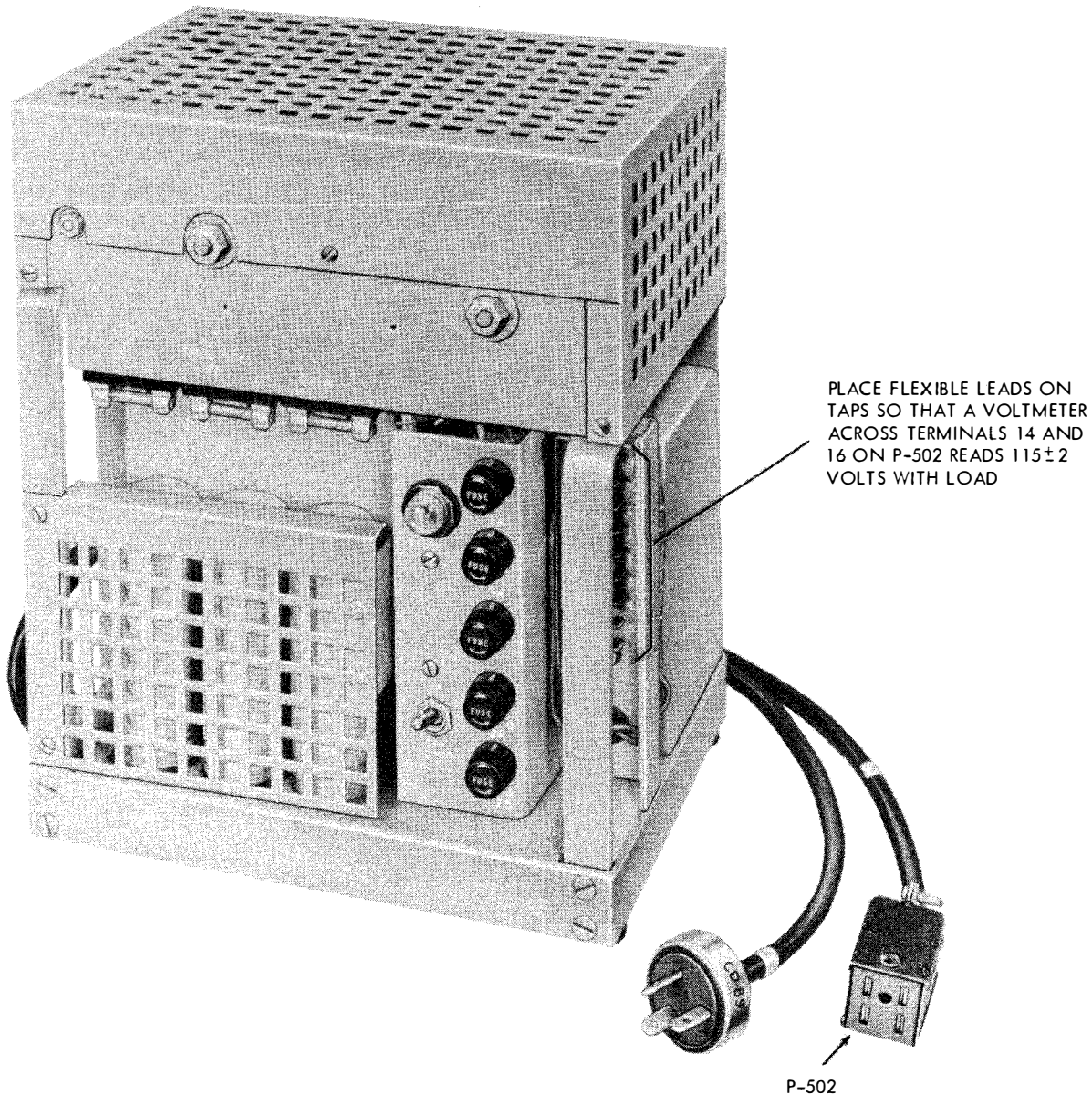
Figure 7-1. Power Supply PP-987/U, Adjustments
