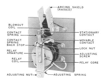
Fig. 1 - Typical Reverse Current Relay
