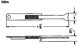
Make-busy tool. For grounding the outside springs of 245-, 254-, 263- and 264-type relays by shorting the springs to the cover ground. On 245- and 254-type relays, the tool clamps on the spring. On 263- and 264-type relays, the tool clamps on the insulator which forces the tool prongs against the spring. Replaces the 530A tool. For use on 245-, 254-, 263- and 264-type relays.
