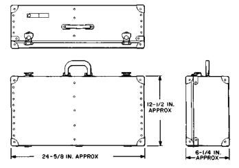
A fabricated gray polyethylene container similar in construction to a small trunk having a hinged cover and equipped with a handle. Arranged to transport cords of various types used with the portable scanner and encoder unit and transmitting data set unit of the Traffic Measurement System No. 1A.
