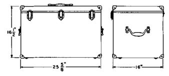
Consists of a black fibre case provided with a hinged cover and handles. The interior is equipped with a tool mounting board and a removable partitioned tray. For use in housing contact cleaning tools for panel systems.
