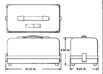
Consists of a molded-plastic base arranged for mounting a data set and associated equipment and a cover equipped with a handle. The base and cover are equipped with latches for assembly. For use in housing and transporting a portable data set J3B005D of which the carrying case is a component part.
