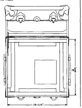
Consists of a wooden frame covered with black vulcanized fibre. The key for the lock on the cover unlocks all KS-14253 cases. For transporting an AMA KS-13835 reader between a central office and a maintenance center.
