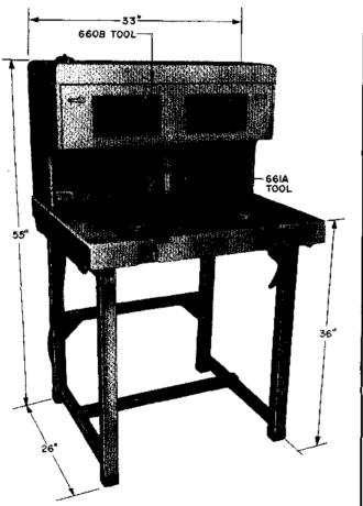
Card coding tool. The 660B and 661A tools are parts of the 659E tool. Replaces the 659B tool. For use in coding cards from blanks for 1-type translators.
