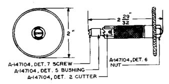
Jack mounting counterbore. For counterboring jack mounting to accommodate the shoulder of a replacement sleeve for worn 141-type jacks.
