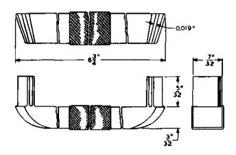
Guard. Replaces the D-178346 tool. For use on the KS-13882 perforators to cover the points of the static eliminator to protect the hands of the operator when making adjustments.
