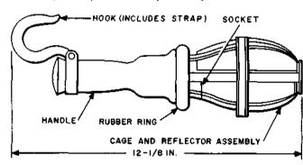
Consists of a kit of parts to be assembled in the field as a "trouble" light. Parts supplied are a soft rubber handle, fiber cage and reflector assembly, lamp socket, and fiber hook. When assembled to a suitable cable, the light is intended for general 120 Vac use.
