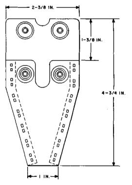
Replaces shave hook guard AT-6893. For use on B shave hook AT-7151. (Specification AT-7151)
