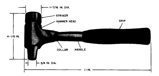
Equipped with a shock-mounted striker with one end tapered for use in restricted areas.
