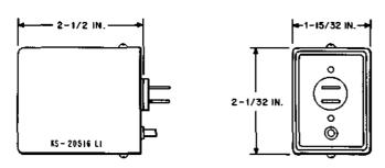
A metal enclosed, single-unit device consisting of a relay driven by a transistorized, astable multivibrator which is powered off a 48-volt dc source. Intended to provide ground pulses for rotating the number wheels of from one to three 14-type message registers at approximately 5 Hz to facilitate cleaning of the registers with a vacuum cleaner.
