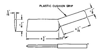
For use in stripping lead-covered cable, PBX installation only. (Specification AT-6312)
