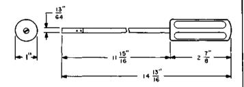
Sleeve terminal locking tool. For use on 49-type jacks to twist the sleeve terminal to lock the sleeve in position.
