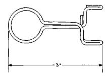
For use in adjusting bellows relays in pneumatic tube equipment.
