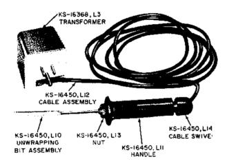
A heated wire-unwrapper tool for use in loosening and removing soldered-wrapped connections of 22-, 24-, and 26-gauge wires. Replacement procedures for parts are covered in Section 075-121-802.
