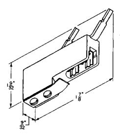
For use on 121-type protectors and 300-type connectors to provide means for connecting to the cable pairs at the test terminals. This clip may be used with the M2EM cord for bypassing the protector.
